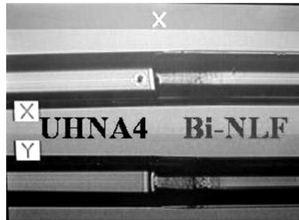
**Fig 5.2** Splicing point of Bi-HNLF to the intermediary fiber [8]
