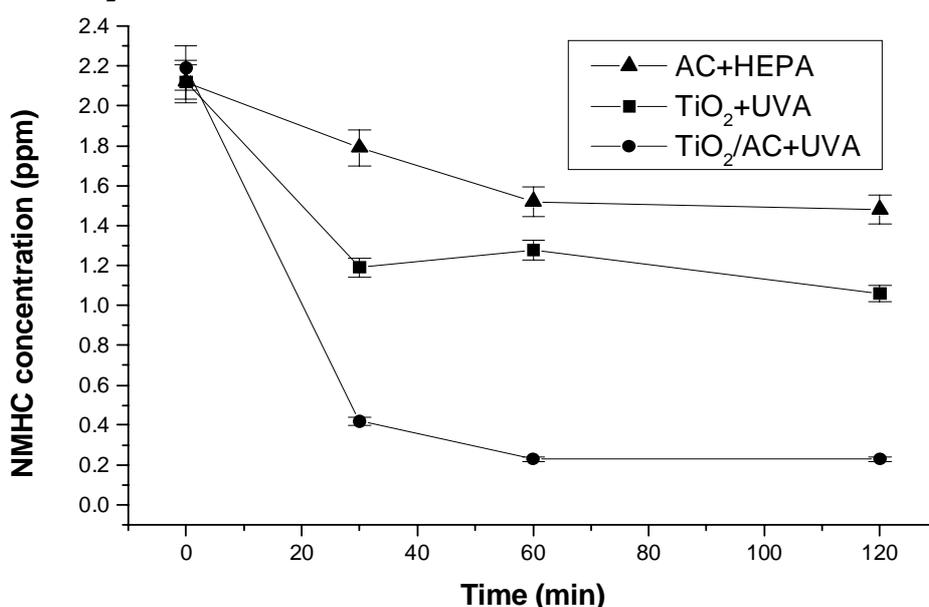
Figure 7.7 Toluene removal by the air cleaner with AC+HEPA, TiO<sub>2</sub> filter and TiO<sub>2</sub>/AC filter.
