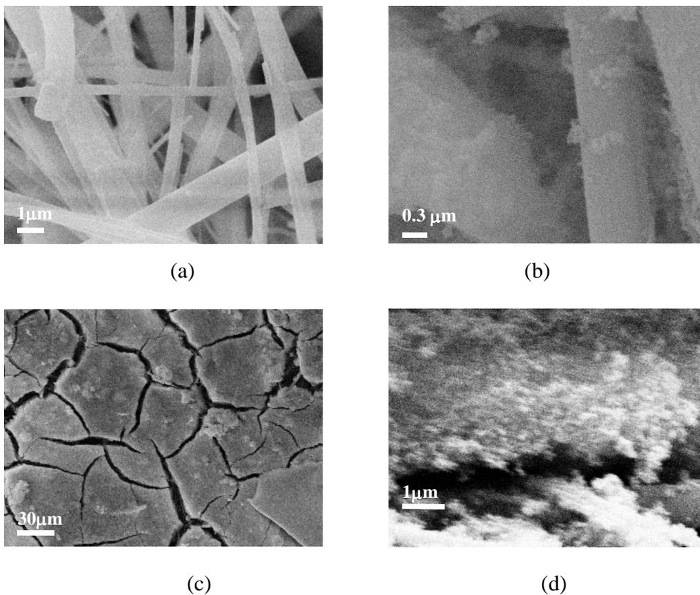
*Figure 4.1* Scanning electron micrographs of (a) fiber, (b) fiber coated with  $\text{TiO}_2$ , (c) top and (d) cross-section.
