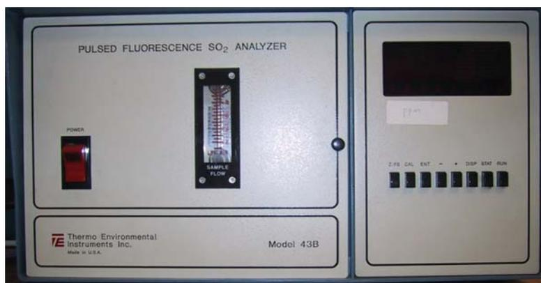
Figure A3 SO<sub>2</sub> analyzer (Thermo Environmental Instrument Inc., Model 43b).
