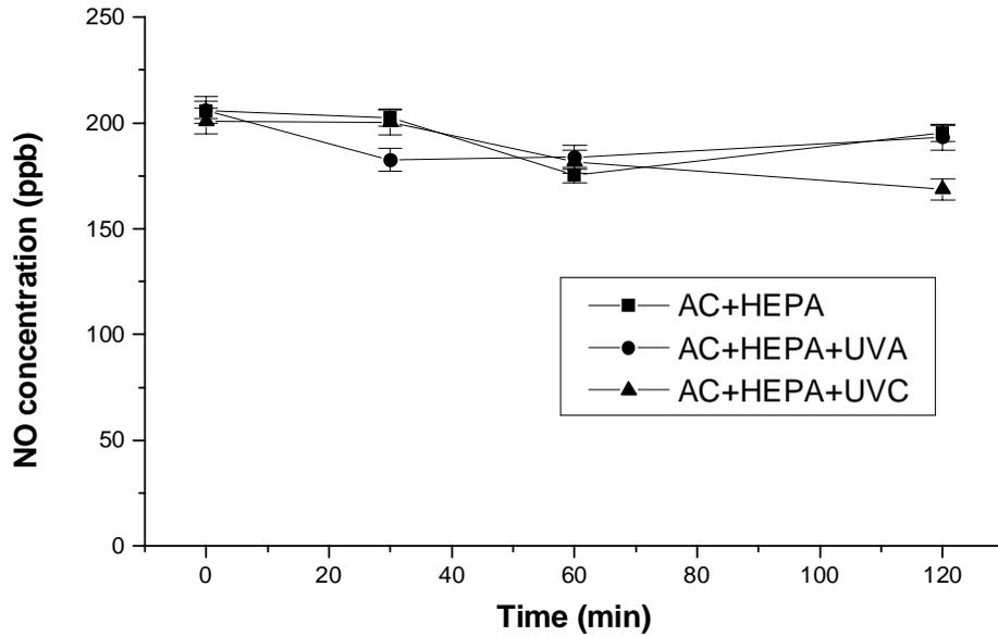
Figure 7.3 NO removal using the air cleaner settings.
