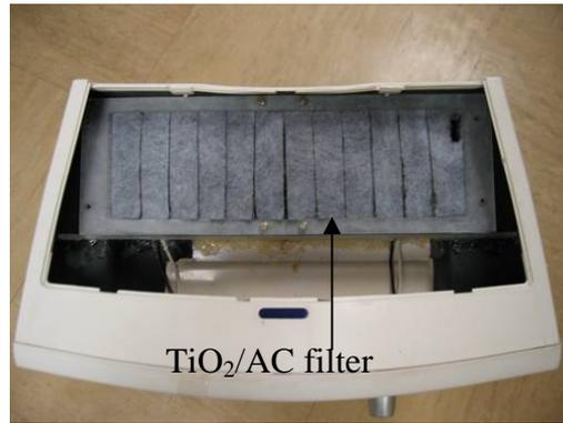
*Figure 3.6* Top view of the commercial air cleaner installed with the TiO<sub>2</sub>/AC filter.
