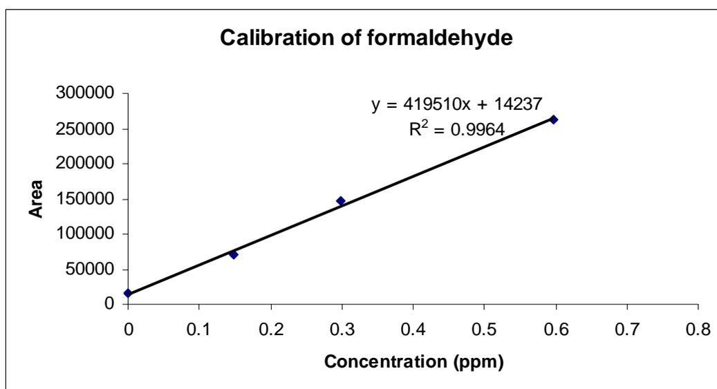
Figure 3.14 Formaldehyde calibration curve.
