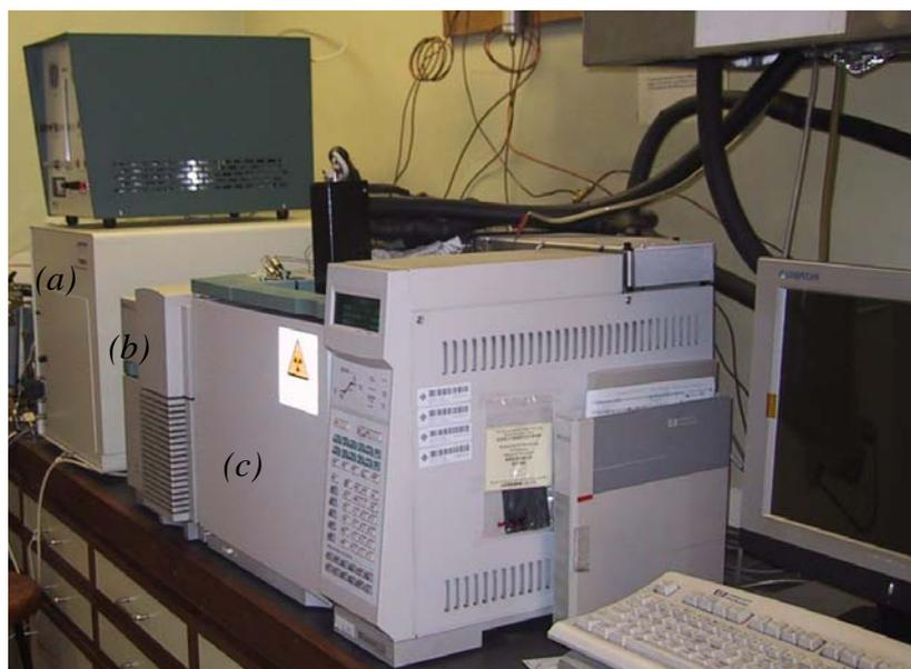
*Figure A6* GC/MS system used for VOCs analysis; (a) Nutech Cryogenic Concentrator; (b) Mass Selective Detector; (c) Gas Chromatography.
