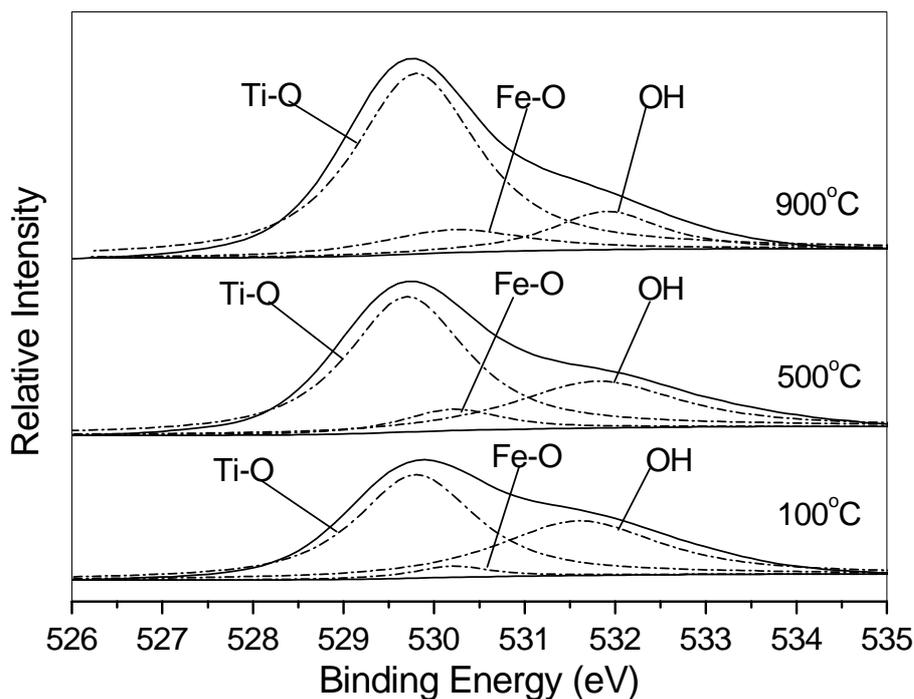
*Figure B7* High-resolution XPS spectra of the O1s region of the TiO<sub>2</sub> thin films calcinated at 100, 500 and 900°C.
