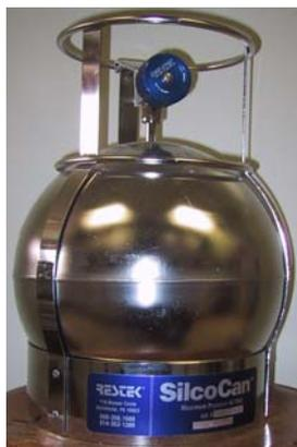
*Figure A5* Summer canister used for VOCs sampling.
