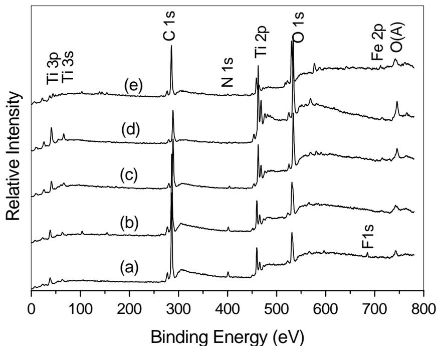
*Figure B5* XPS survey spectra for the surface of TiO<sub>2</sub> films calcinated at (a) 100, (b) 300, (c) 500, (d) 700 and (e) 900°C.
