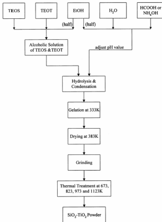
*Fig. 2.11* Preparation of  $\text{TiO}_2\text{-SiO}_2$  powder by sol-gel method<sup>(Yu and Wang, 2000)</sup>.
