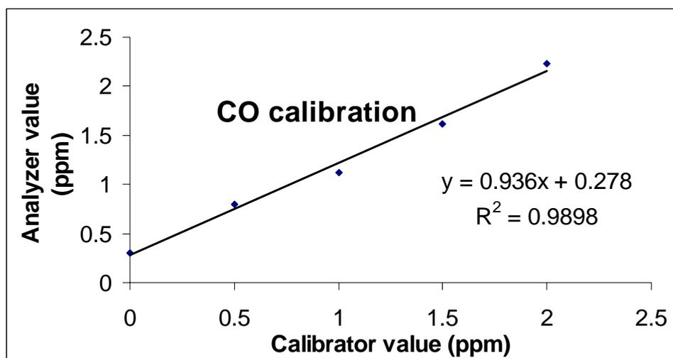
Figure 3.12 CO calibration curve.
