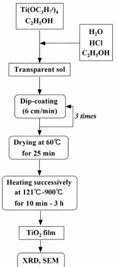
Fig. 2.10 Preparation of  $\text{TiO}_2$  thin film by sol-gel method<sup>(Lin et al., 1998)</sup>.
