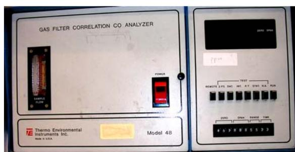
Figure A1 CO analyzer (Thermo Environmental Instruments Inc. Model 48)
