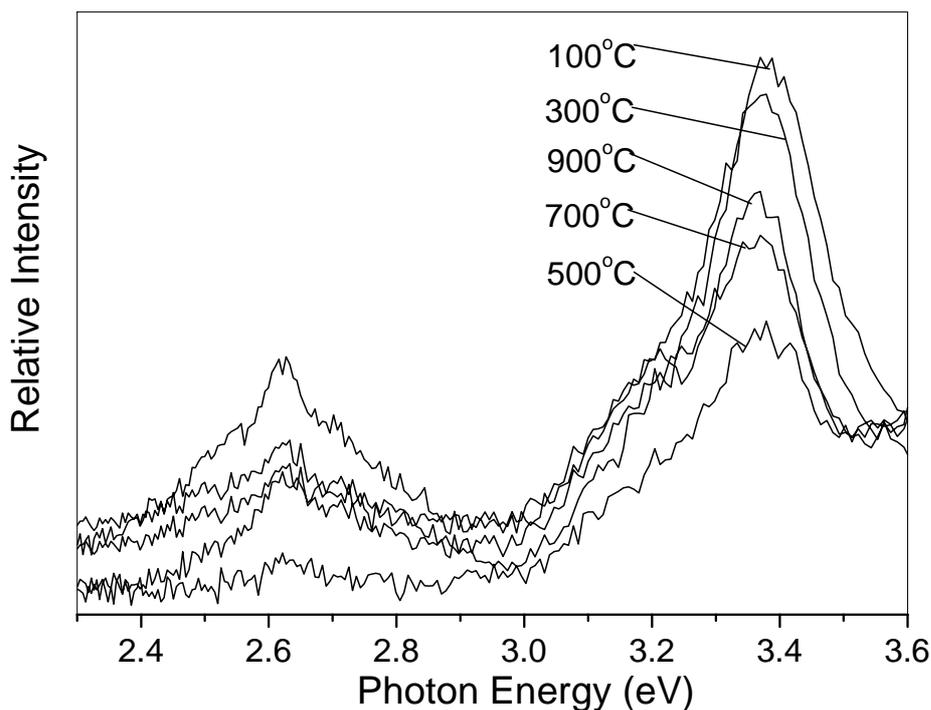
Figure B4 Photoluminescence spectra of TiO<sub>2</sub> thin films calcinated at 100, 300, 500, 700 and 900°C.
