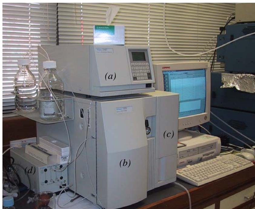
Figure A8 HPLC (Waters) for aldehydes analysis; (a) UV detector; (b) binary pump; (c) column; (d) in-line degasser.
