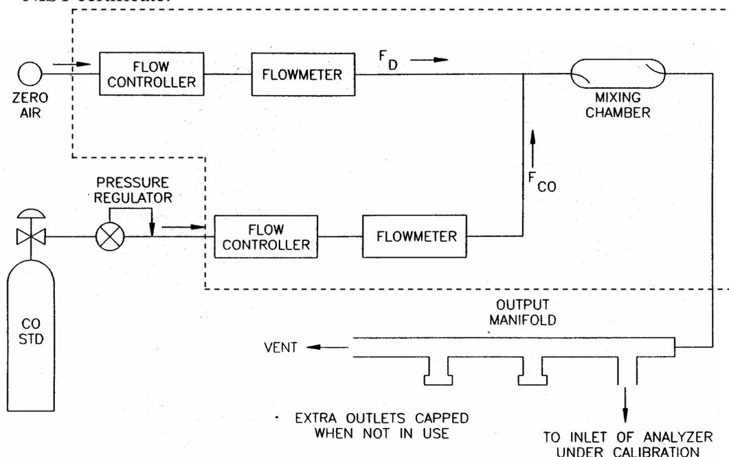
Figure 3.11 Schematic diagram of CO calibration.
