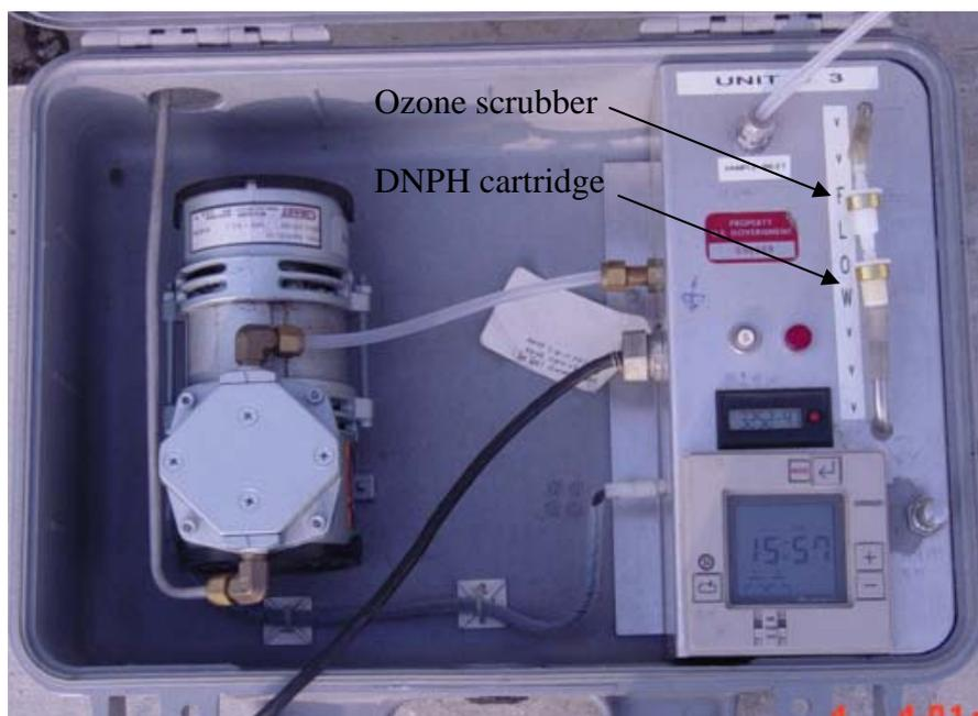
Figure A7 DRI standard carbonyl sampler.
