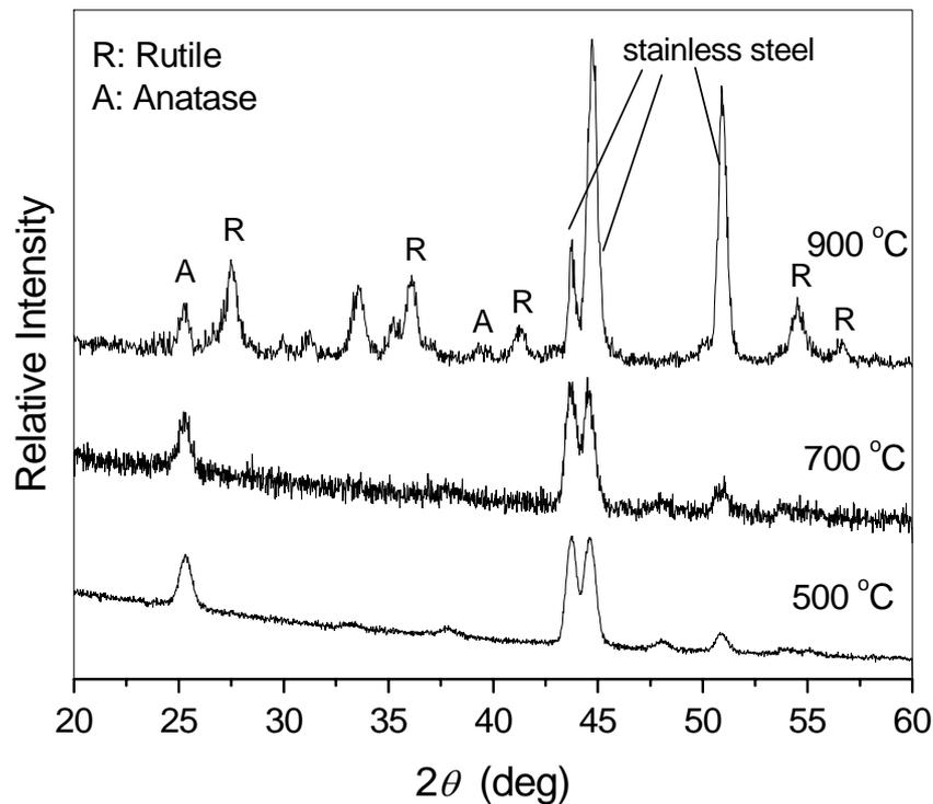
Figure B2 X-ray diffraction patterns of TiO<sub>2</sub> thin films calcinated at 500, 700, and 900°C.
