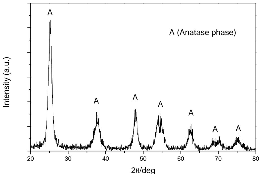
Figure 4.8 XRD patterns of photocatalyst T1.
