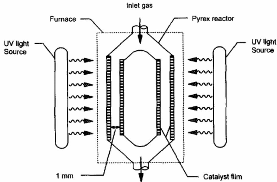
Figure 2.8 Schematic diagram of a typical annular flow reactor with external illumination<sup>(Larson et al., 1995)</sup>.
