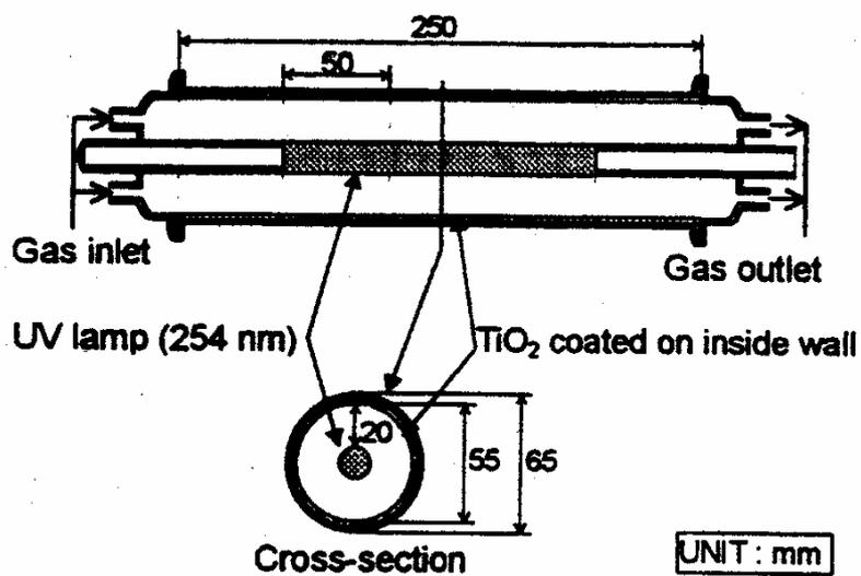
Figure 2.7 Schematic diagram of a typical annular flow reactor with internal illumination (Sakamoto et al., 1999)
