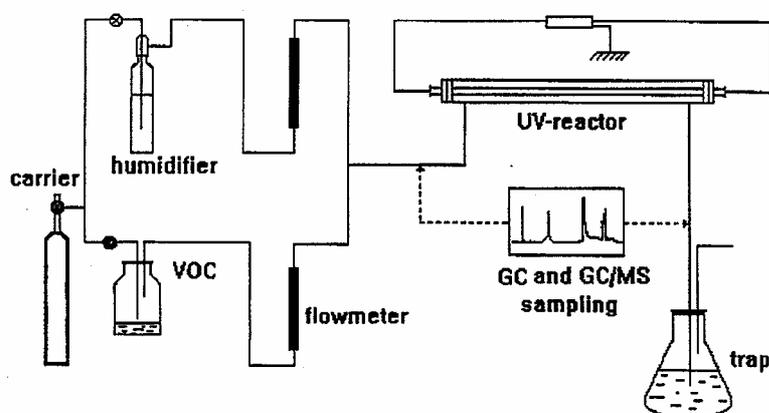
Figure 2.5 Schematic diagram of a typical photocatalytic experiment using liquid VOCs as pollutant source (Alberici and Jardim, 1997).
