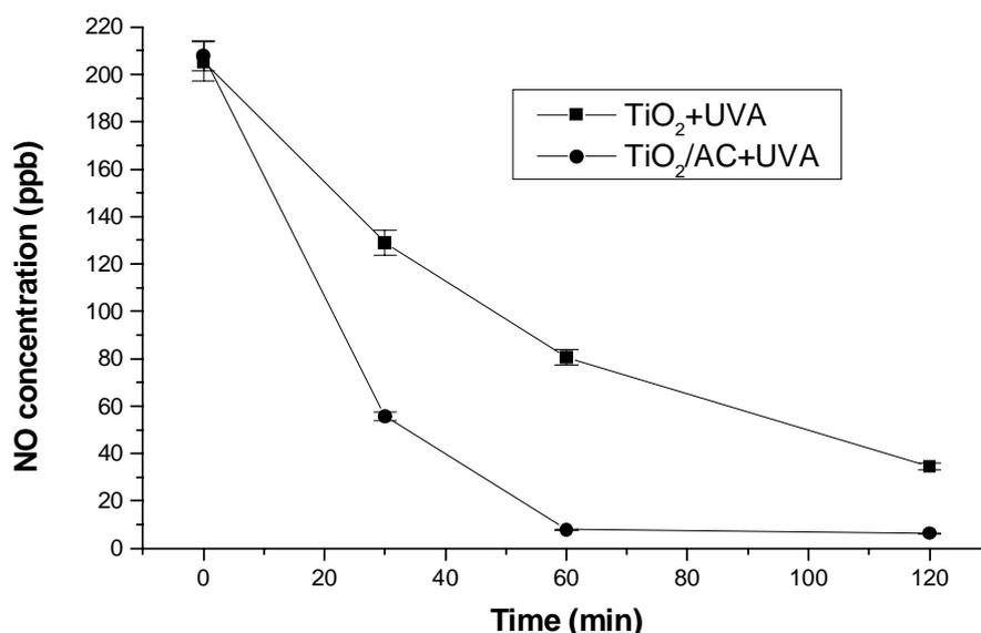
Figure 7.5 NO removal using TiO<sub>2</sub> filter and TiO<sub>2</sub>/AC filter.
