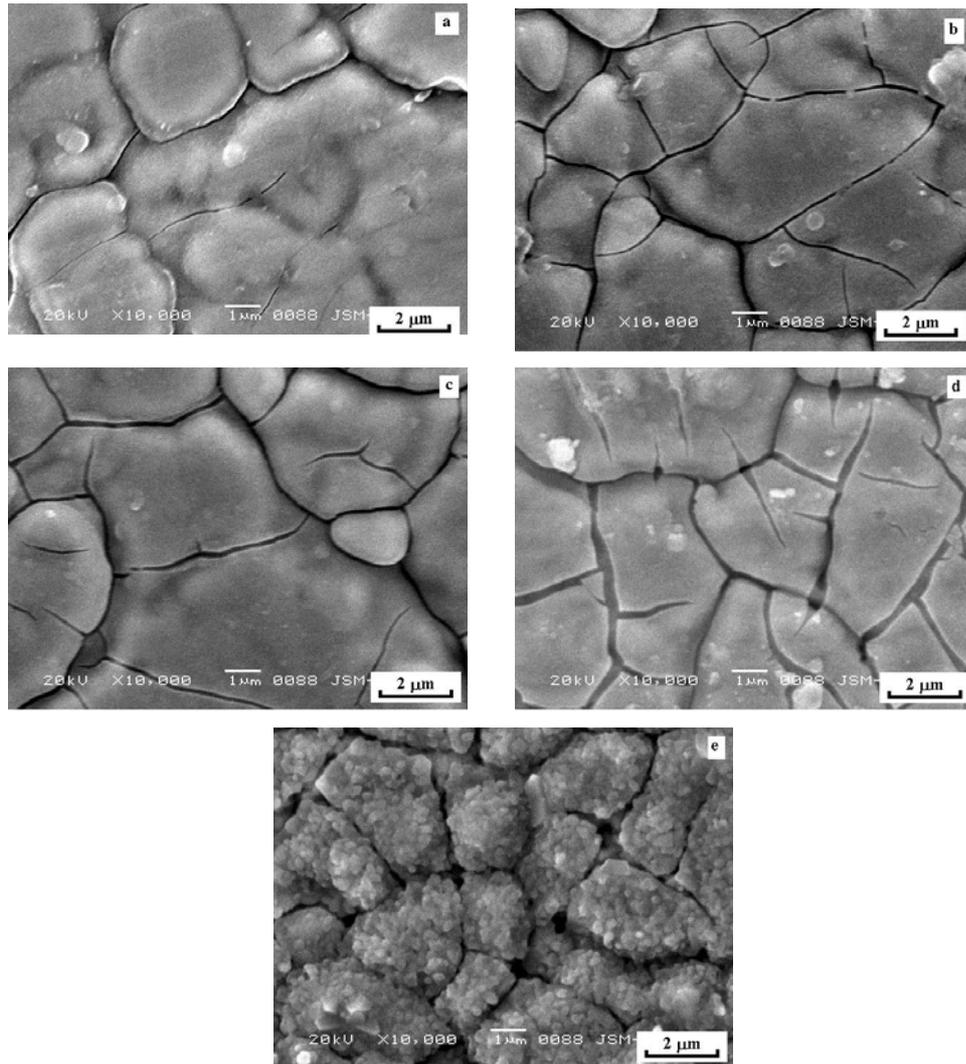
*Figure B3* SEM micrographs of TiO<sub>2</sub> films calcinated at (a) 100, (b) 300, (c) 500, (d) 700 and (e) 900°C.
