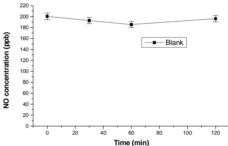
Figure 7.1 Leakage test of the environmental chamber using NO.
