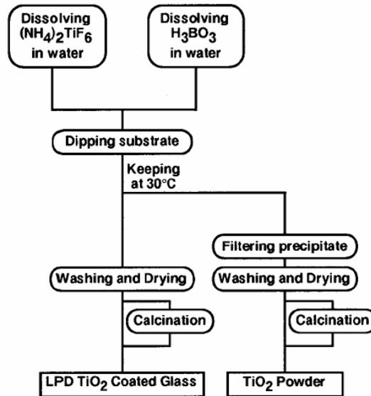
Fig 2.9 Schematic diagram of TiO<sub>2</sub> thin film and powder synthesis by LPD method<sup>(Kishimoto et al., 1998)</sup>.
