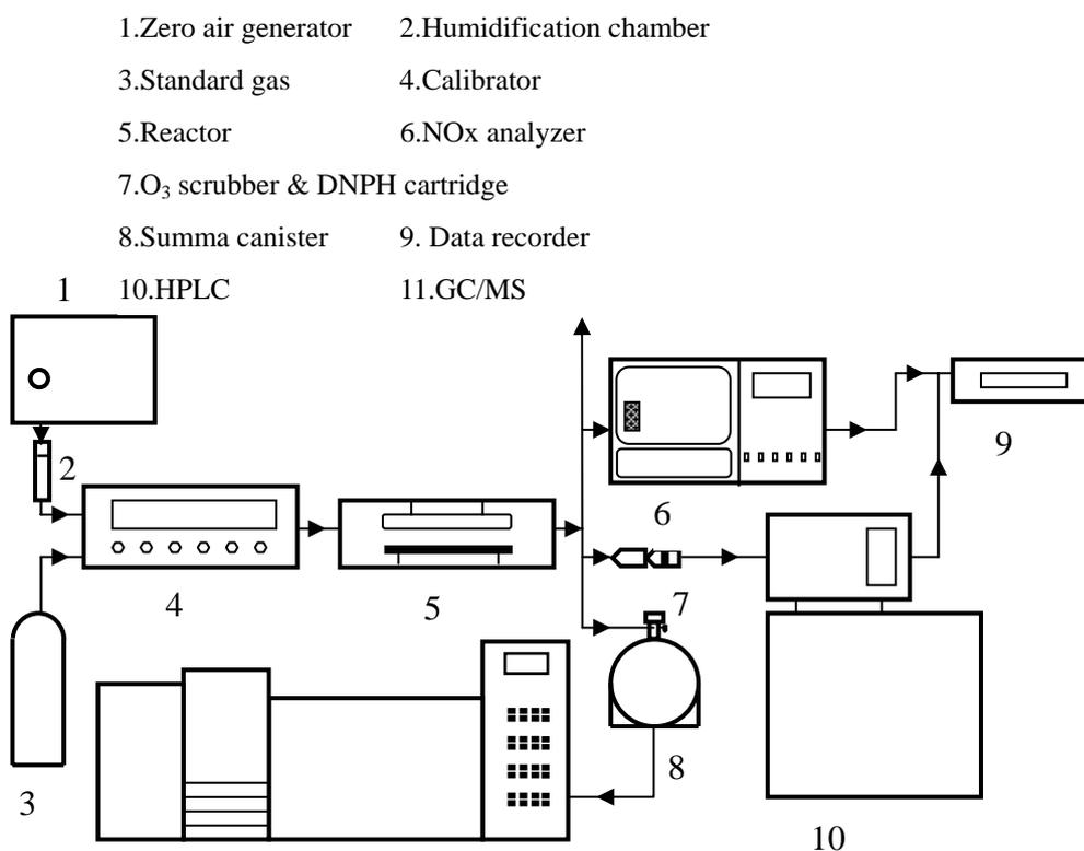
Figure 3.2 Schematic diagram of the experimental setup.
