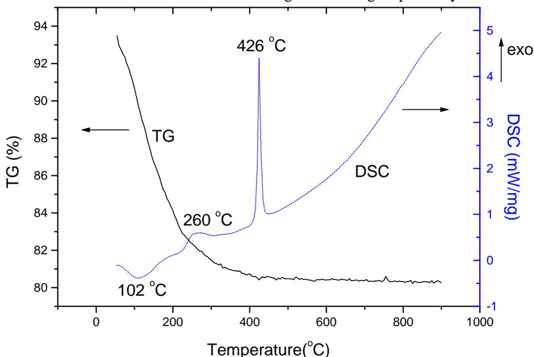
Figure 4.9 DSC-TG analyses of photocatalyst T1.
