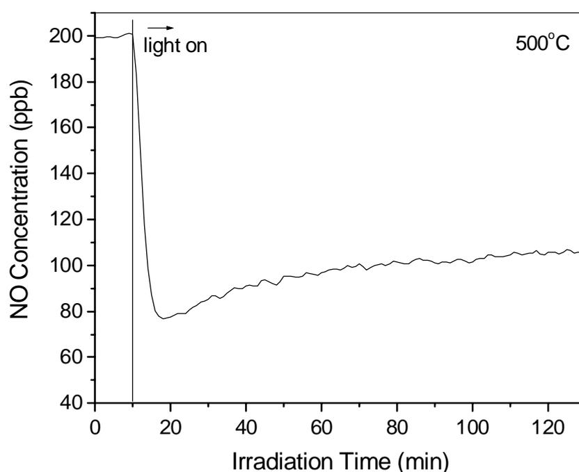
*Figure B8* The photodegradation of NO for the TiO<sub>2</sub> thin film sample calcinated at 500°C. Experimental conditions: residence time 3.7 min, humidity levels 2,200 ppmv, 200 ppb NO.
