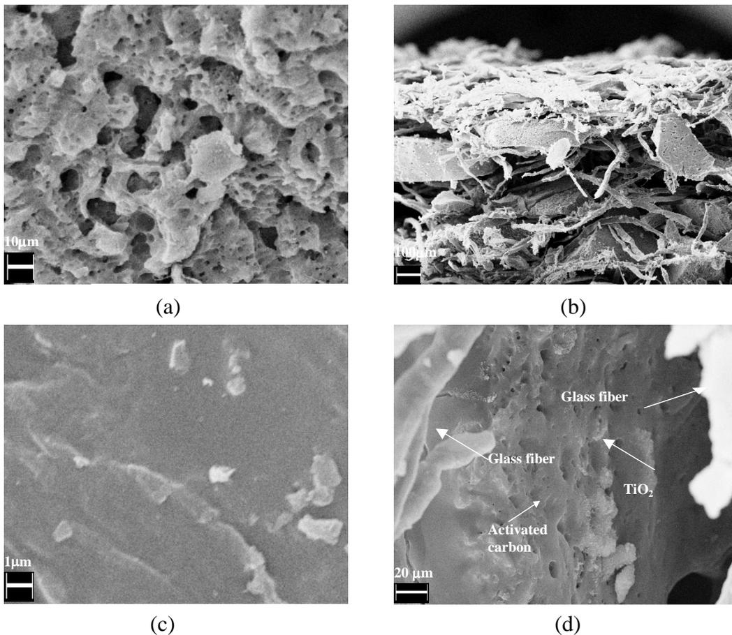
*Fig 5.1* Scanning electron micrographs of (a) activated carbon, (b) glass fiber combined with activated carbon, (c) intimate contact of  $\text{TiO}_2$  and activated carbon (d) inner layer of activated carbon coated with  $\text{TiO}_2$ .
