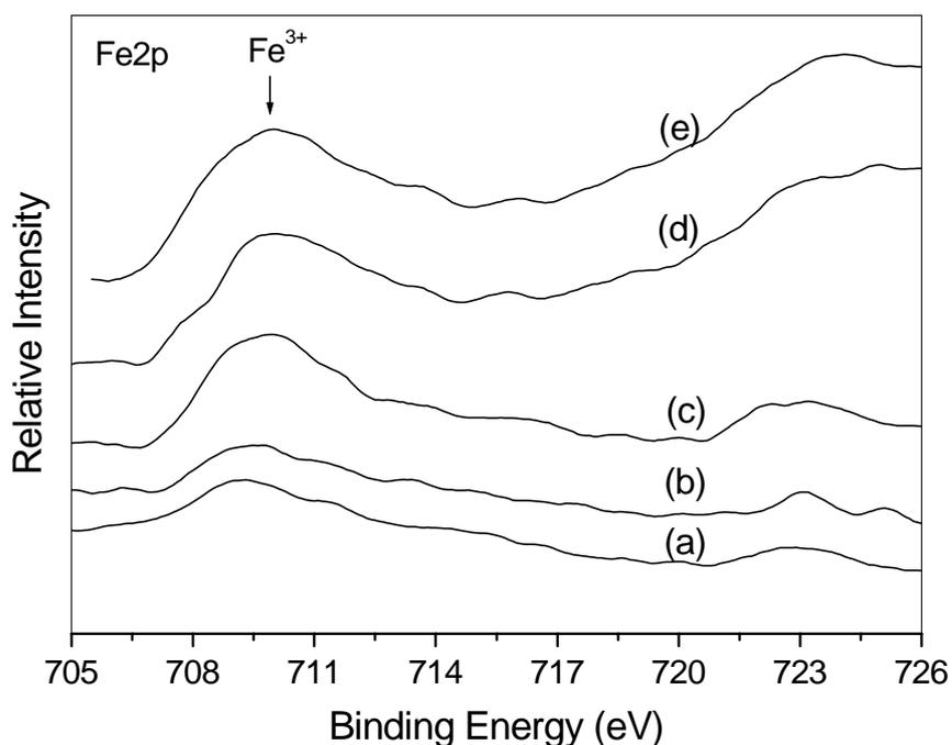
*Figure B6* High-resolution XPS spectra of the Fe2p region of the TiO<sub>2</sub> thin films calcinated at (a) 100, (b) 300, (c) 500, (d) 700 and (e) 900°C.
