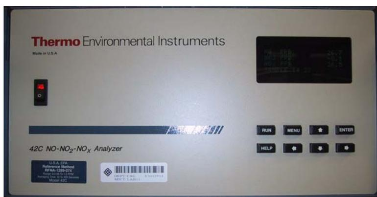
Figure A2 NO-NO<sub>2</sub>-NO<sub>x</sub> analyzer (Thermo Environmental Instrument Inc., Model 42c).
