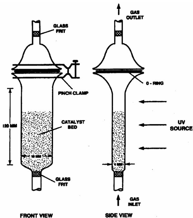
Figure 2.6 Schematic diagram of fluidized bed reactor used by Dibble and Raupp (Dibble and Raupp, 1992)
