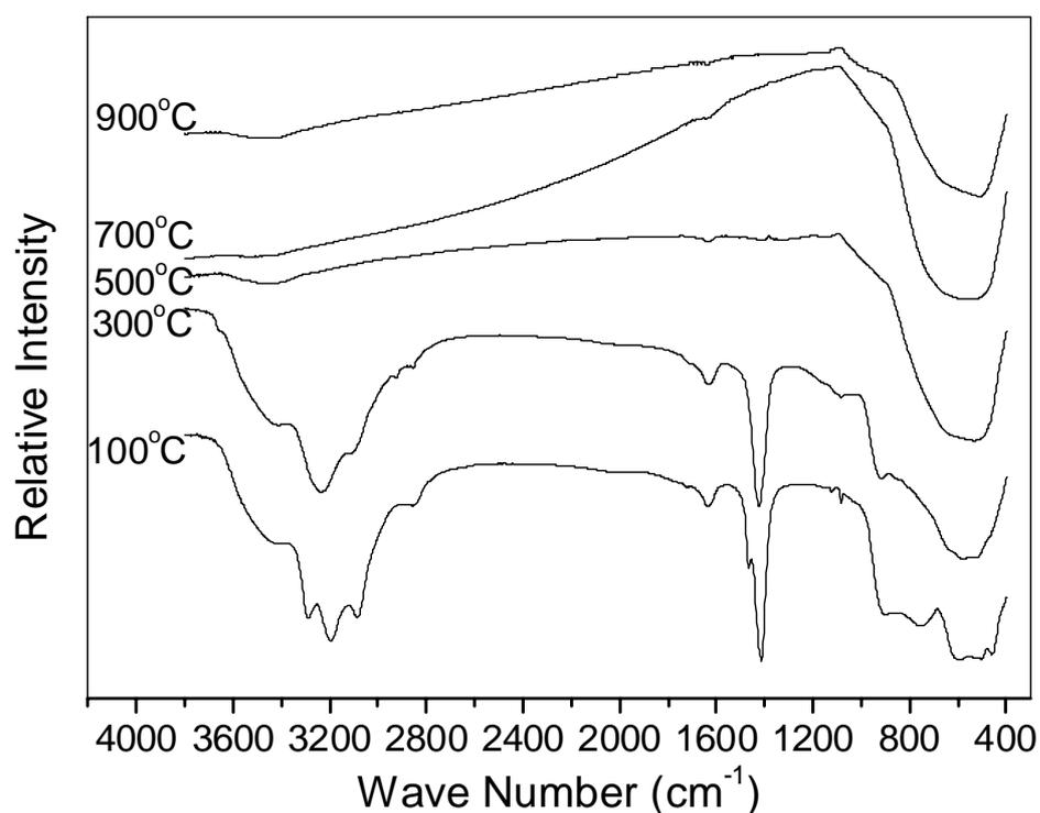
*Figure B1* Infrared spectra of TiO<sub>2</sub> powder calcinated at 100, 300, 500, 700 and 900°C.
