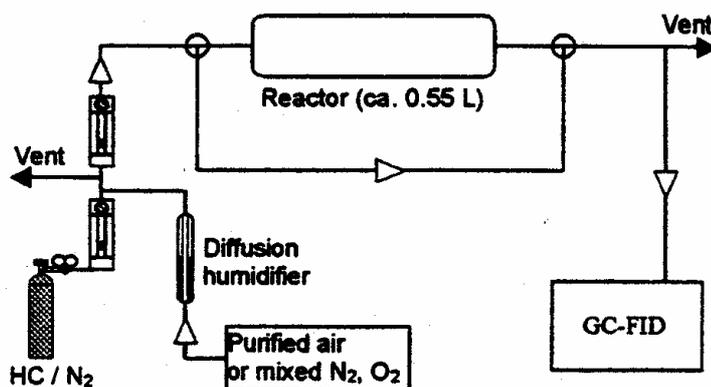
Figure 2.4 Schematic diagram of a typical photocatalytic experiment using standard gas as pollutant source (Sakamoto et al., 1999).
