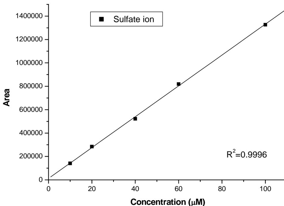
Figure 3.15 Sulfate ion calibration curve.
