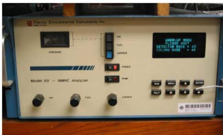
Figure A4 NMHC analyzer (Thermo Environmental Instrument Inc., Model 43b).
