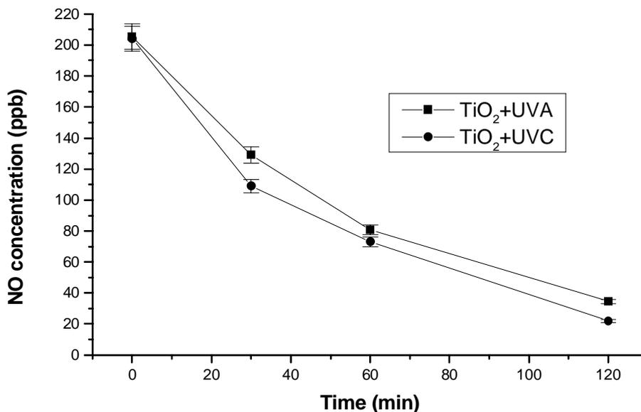
Figure 7.4 NO removal using TiO<sub>2</sub> filter with UVA lamp and UVC lamp.
