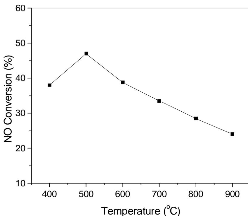
*Figure B9* The removals of NO for the TiO<sub>2</sub> thin films calcinated at different calcination temperatures. Experimental conditions: residence time 3.7 min, humidity levels 2,200 ppmv, 200 ppb NO.
