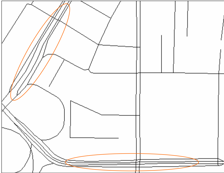
Figure 8-8 Undetected mismatches in parallel lanes
