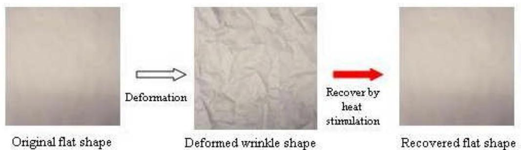
**Figure 3.6 Fabric shape memory effect of flat appearance**
