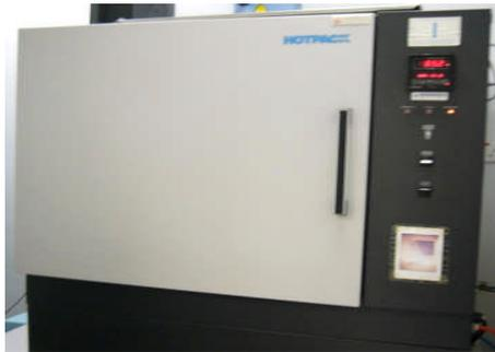
**Figure 3.20 Conditioning Chamber (outside view)**
