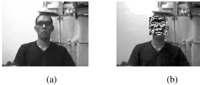
Figure 3-3 (a) The original image, and (b) its LBP representation at the face region.
