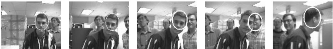
Figure 2-4 Tracking based on using gradient intensity to measure an object's boundary shape and a color histogram to measure the color of an object's interior. (Figure reprinted from [32])
