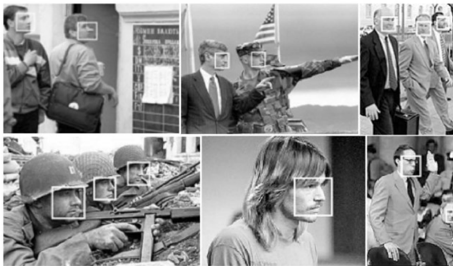
Figure 2-7 Multi-view face detection results for the classifier trained by the FloatBoost algorithm.
