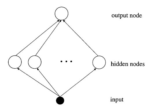
Figure 2.2: Architecture of a two-layer feed-forward neural network with one input, n hidden nodes and one output node.
