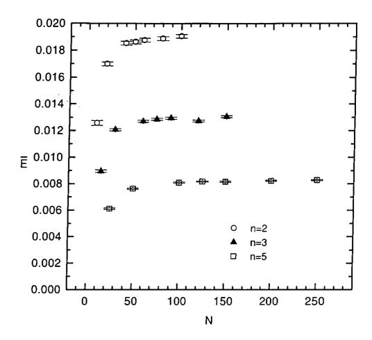
Figure 3.3: Plot of the average error measure  $\bar{E}$  against the number of sample points N in the target function. The three curves result from networks with number of hidden nodes n=2,3 and 5 respectively.
