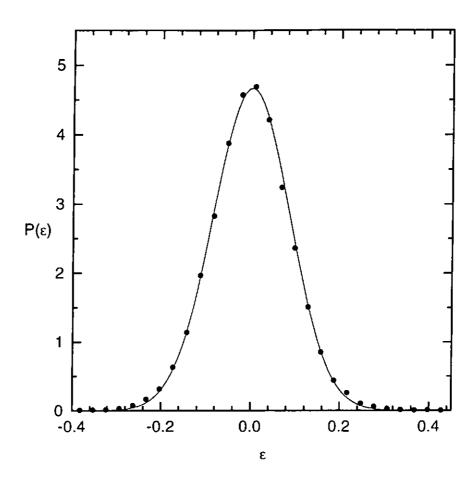
Figure 3.6: Probability distribution  $P(\epsilon)$  of the output error  $\epsilon$ . The fitted line follows the normal distribution with standard deviation  $\sigma_{\epsilon} = 0.0855$ .
