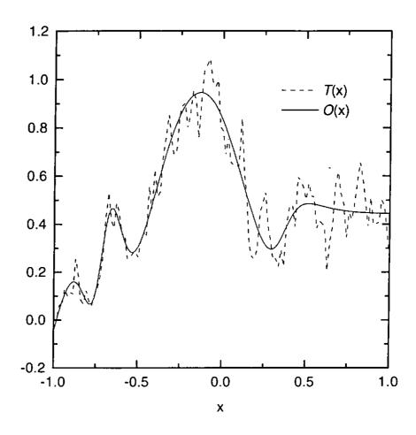
Figure 2.1: An example of a target function T(x) in the form of a Brownian function with N=125 sample points (dotted line). Also shown is the output function O(x) of a trained neural network with n=5 hidden nodes (solid line).
