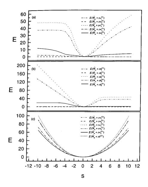
Figure 3.1: One-dimensional cross-sections of the error measure E cutting through a local minimum  $\vec{W}_m$  along axes of the network parameters  $w_i^{(1)}$  (a),  $\theta_i^{(1)}$  (b),  $w_i^{(2)}$  and  $\theta^{(2)}$  (c) respectively.
