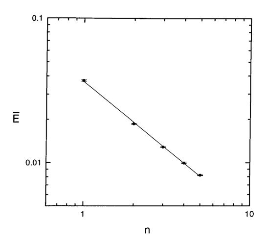
Figure 3.5: Log-log plot of the average error measure  $\bar{E}$  against the number of hidden nodes n at saturation. The slope of the fitted line is -0.942.
