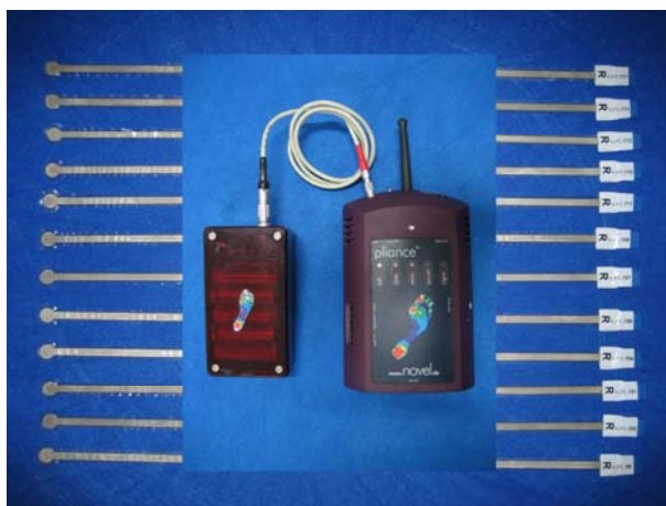
Figure 7.11 The Novel pressure measure system
