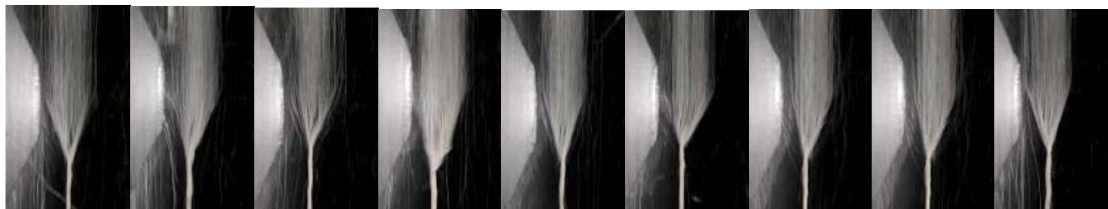
Figure 3-4 Consecutive Photographs of Geometrical Variation of Spinning Triangle in Low Torque Ring Yarn (Spinning speed = 7000rpm, yarn count = 58tex, yarn twist = 398tpm)
