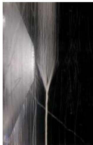
The spinning triangle with multi-bundle
