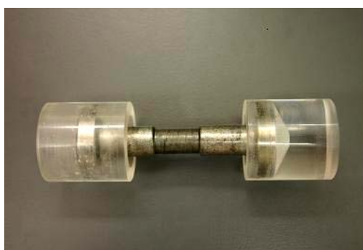
Figure 3-1 General View of the Transparent Roller for Photographic Experiment
