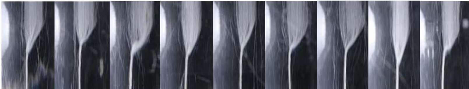
Figure 3-5 Consecutive Photographs of Geometrical Variation of Spinning Triangle in Conventional Ring Yarn (Spinning speed = 7000rpm, yarn count = 58tex, yarn twist = 1193tpm)
