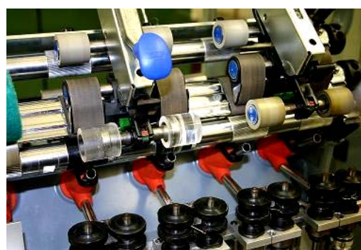
Figure 3-2 General View of the Transparent Roller Mounted on the Spinning Frame
