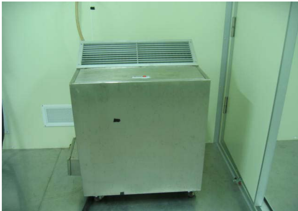
Photo 8 Load generation unit inside conditioned spaces
