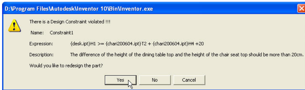
Figure 7.18: The message showing a design constraint is violated and its reason
