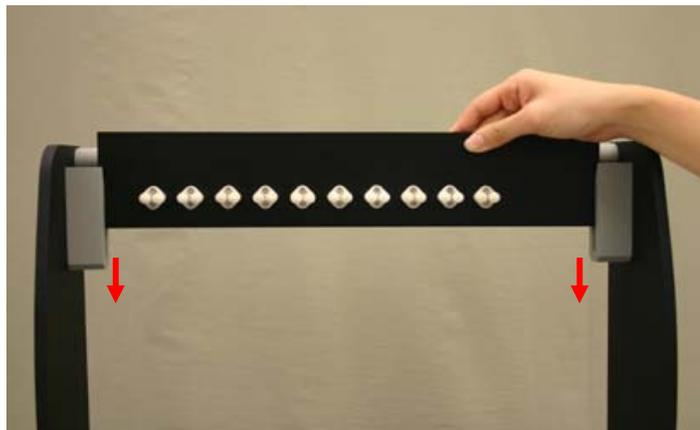
(2) The yarn package is inserted onto the corresponding yarn specimen holder
