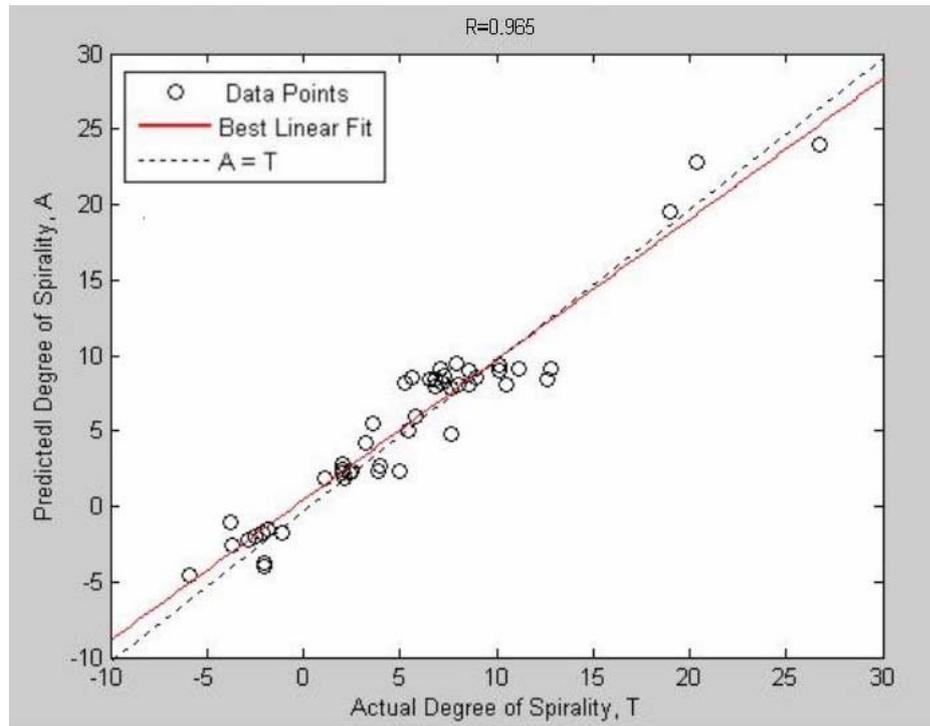
**Figure 5.3 Relationship between the actual and predicted values of spirality for the training set of data (multiple regression model)**
