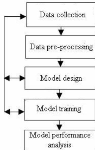
**Figure 5.7** The procedure for neural network development
