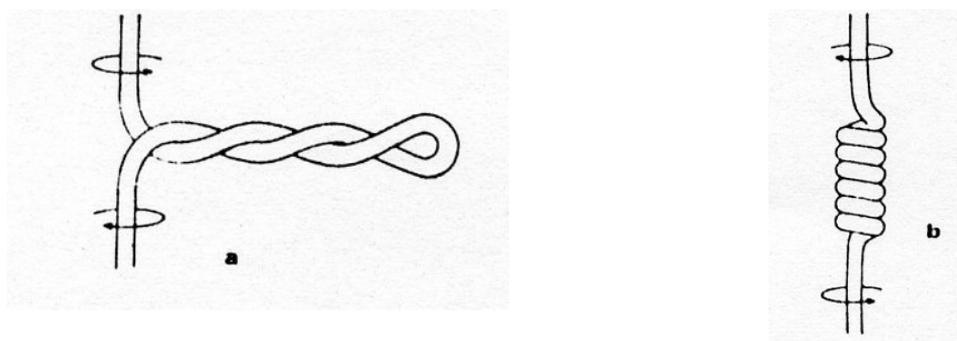
**Figure 2.2(a) Bi-component helical snarl    Figure 2.2(b) Single component helical snarl**
