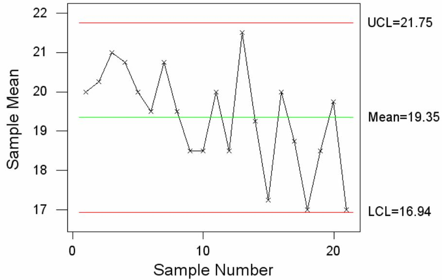
Figure 4.5  $\bar{X}$  Chart for the production trial results
