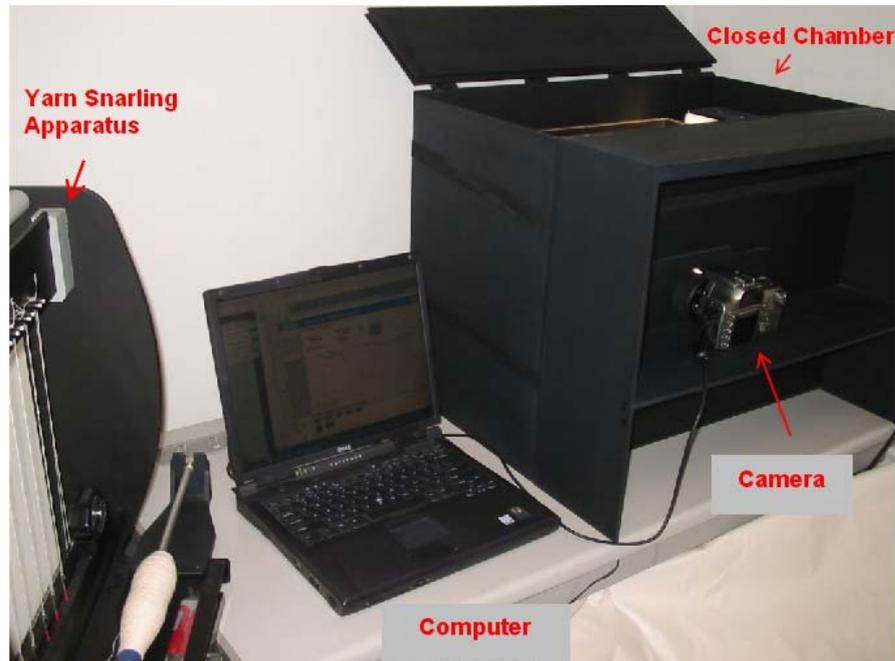
(a) The image acquisition unit set-up
