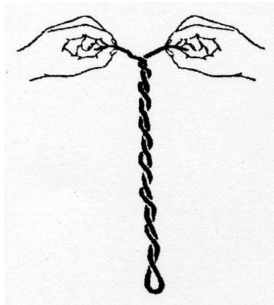
**Figure 2.1 Snarling in a twist lively yarn**
