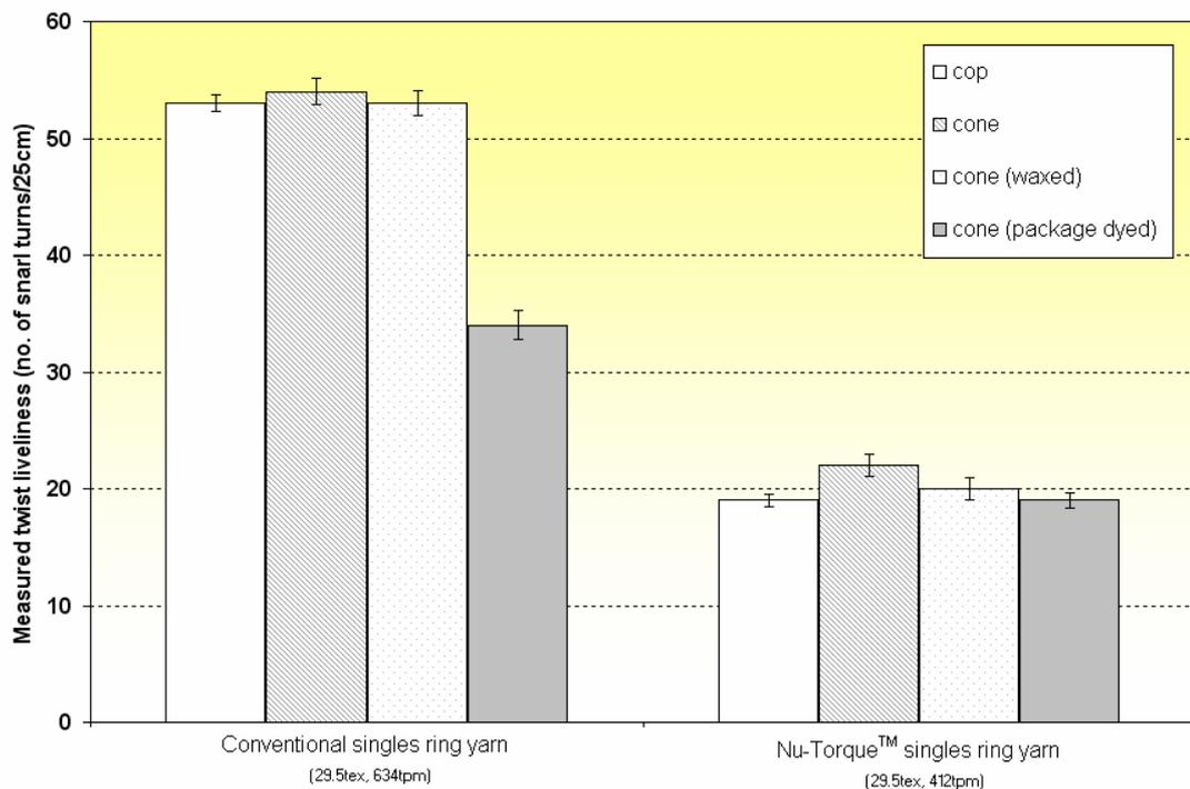
**Figure 4.4 Effect of post-spinning processing on twist liveliness**
