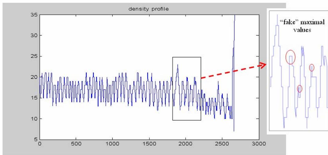
(b) Density profile of the actual yarn sample and illustration of the “fake” maximal values
