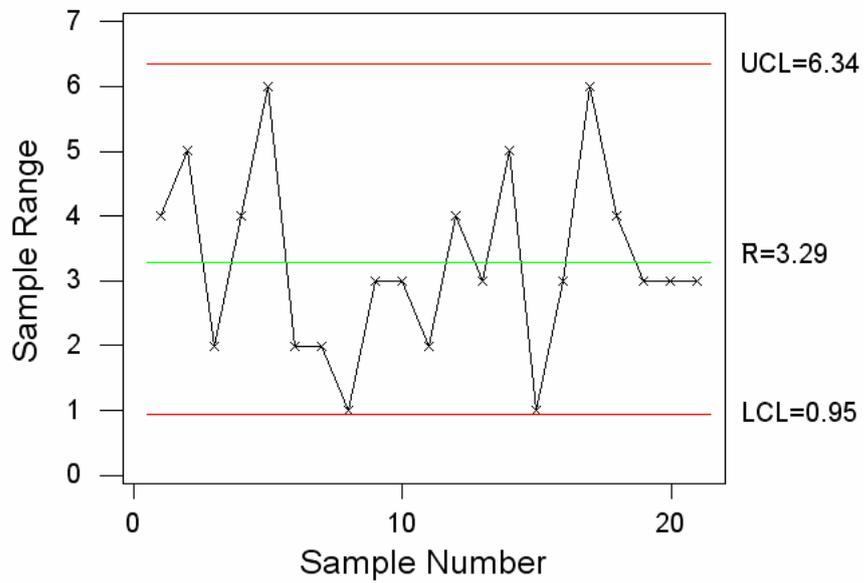
Figure 4.6  $\bar{R}$  Chart for the production trial results
