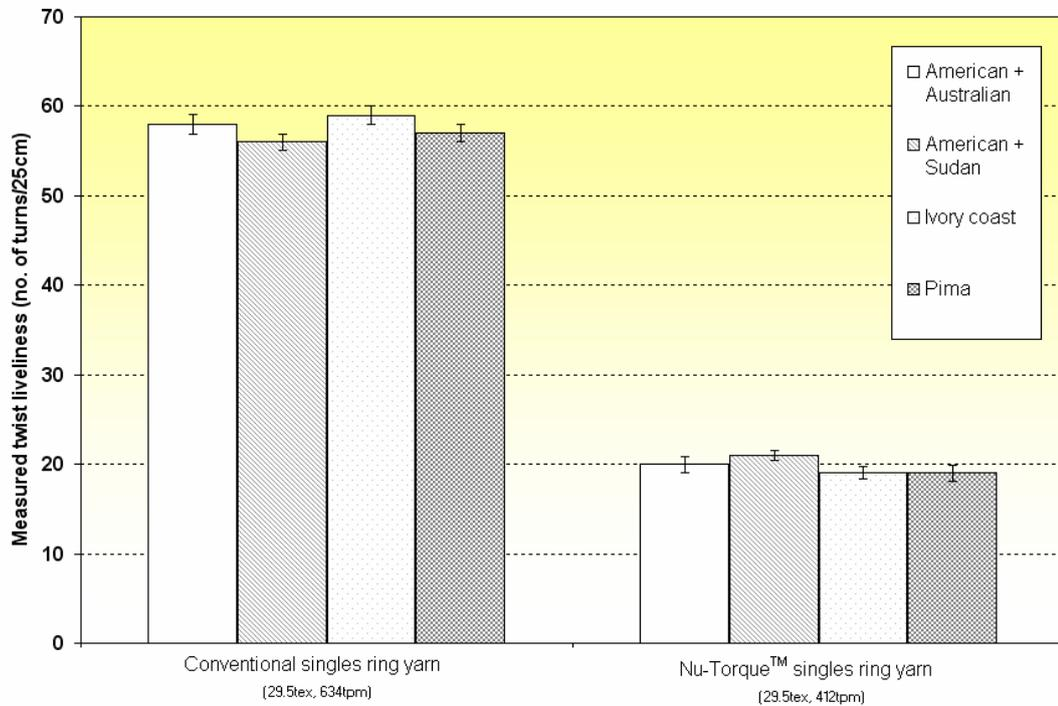
**Figure 4.3 Effect of fibre quality on yarn twist liveliness**
