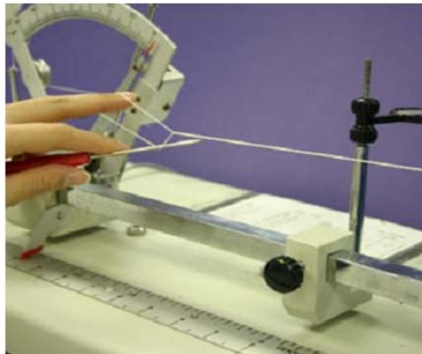
**Figure 3.9 Counting the number of snarl turns on the twist tester**
