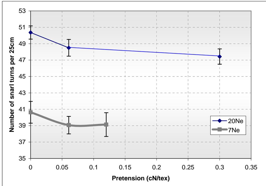
**Figure 3.10 Effect of pretension on the number of snarl turns**
