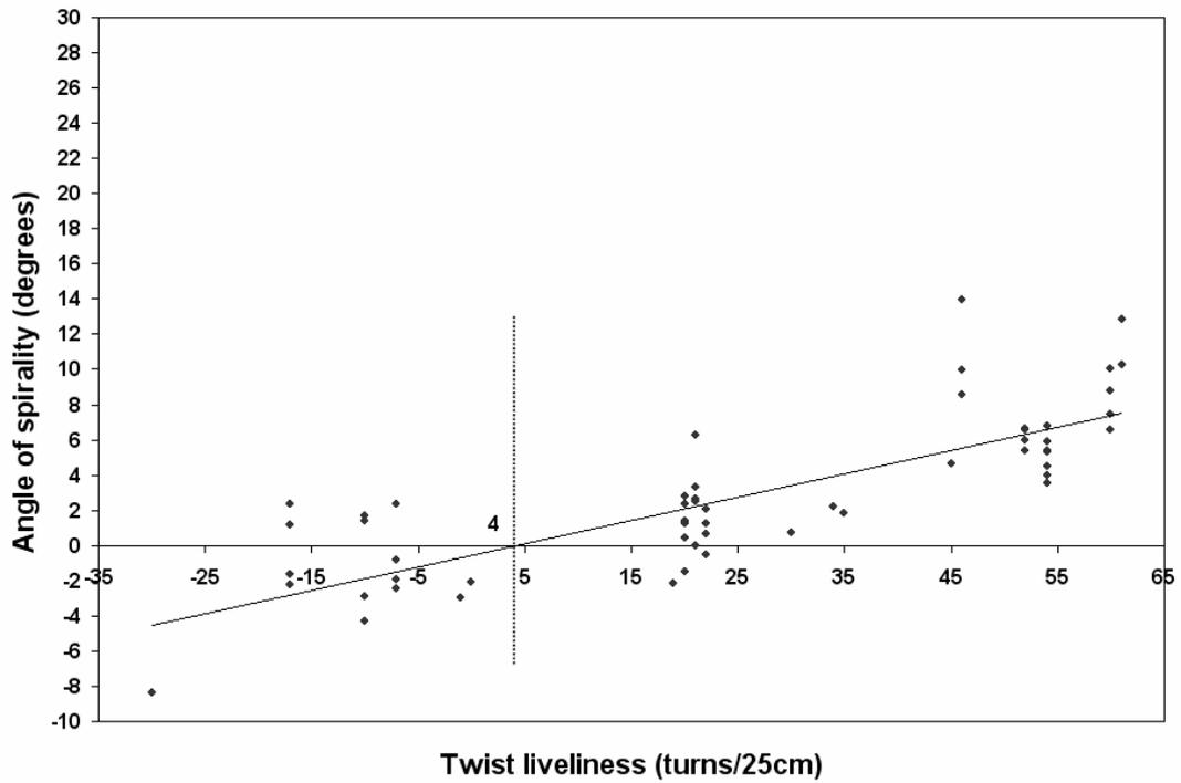
**Figure 5.2(a) Relationship between the measured twist liveliness and angle of spirality of the dry relaxed fabrics**
