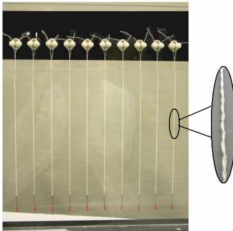
**Figure 6.1** Image of the samples under test in the water bath
