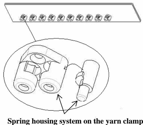
**Figure 3.6 Illustration of the yarn sample holder and yarn clamps**
