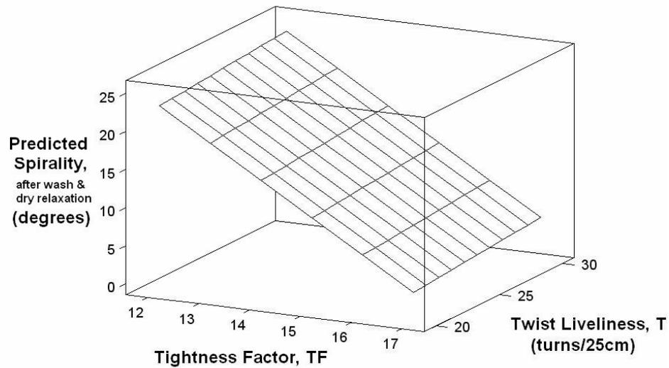
**Figure 5.4 Effect of twist liveliness and tightness factor on spirality**
