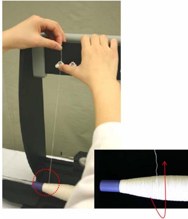
**Figure 3.4 Method for drawing the yarn end from the specimen holder**
