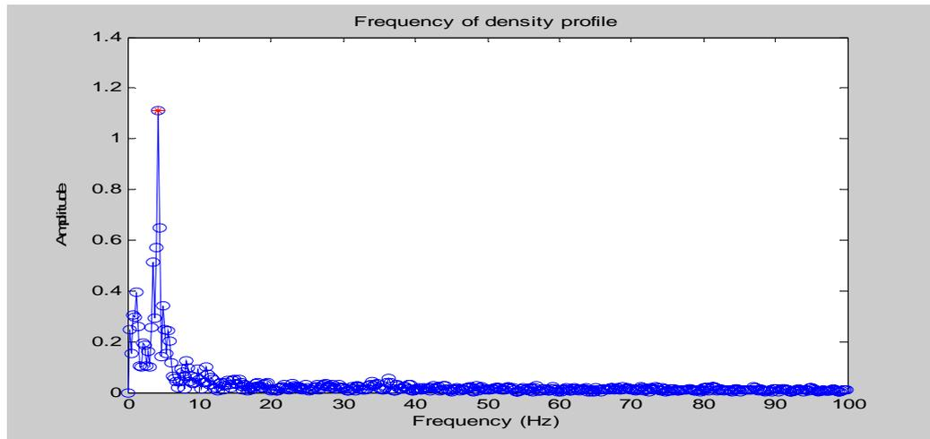
**Figure 6.8** Result of applying FFT to the density profile of the actual yarn sample
