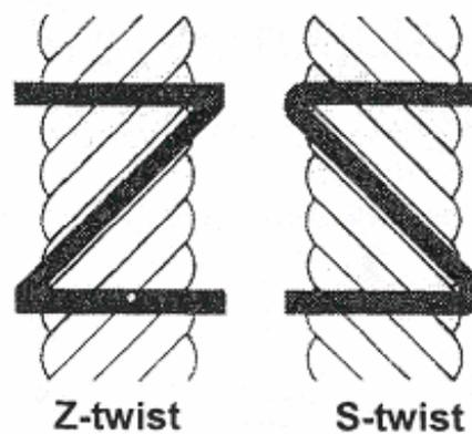
**Figure 2.5 Twist direction**
