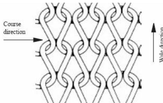
**Figure 2.4 Technical face of a single jersey fabric**
