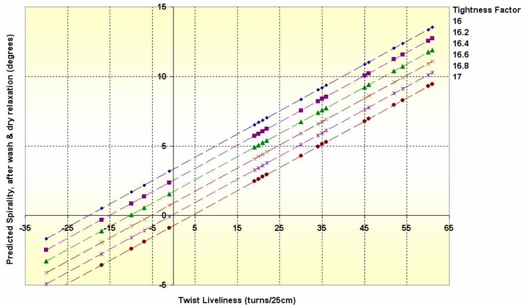
**Figure 5.5 Relationship between spirality and twist liveliness for various values of tightness factors**
