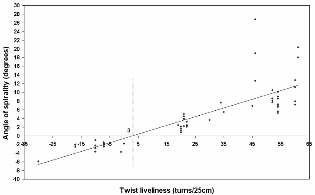
**Figure 5.2(b) Relationship between the measured twist liveliness and angle of spirality of the wash and dry relaxed fabrics**
