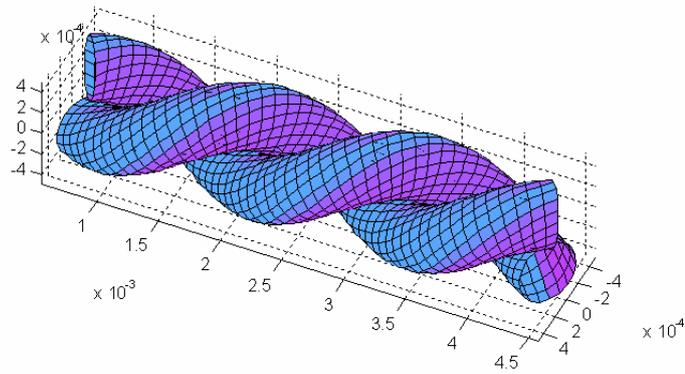
**Figure 6.4 Simulated 3D yarn structure with a uniform distribution of snarls**
