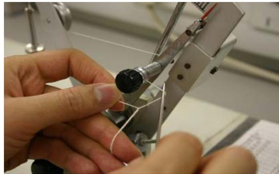
The other end of yarn sample is pulled out from the clamping element and fixed to the opposite clamp on the twist tester.
