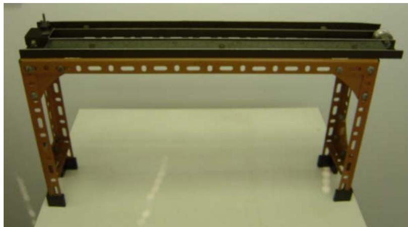
**Figure 3.1 Residual Torque Tester**
