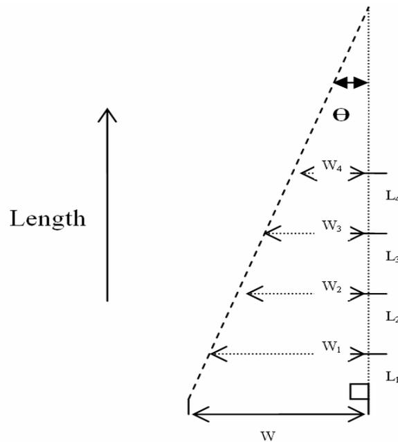
**Figure 5.1** Technique for measuring fabric spirality
