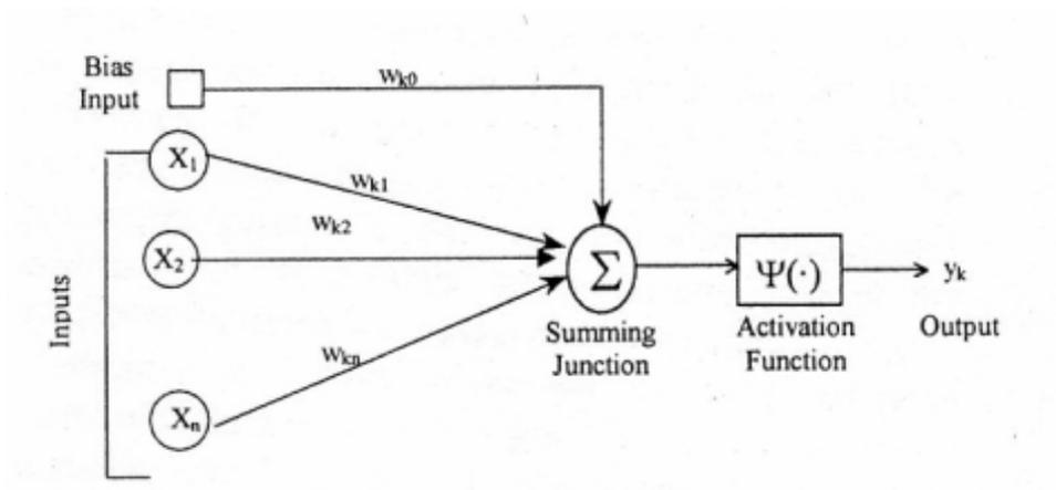
**Figure 5.6 Schematic representation of an artificial neuron**
