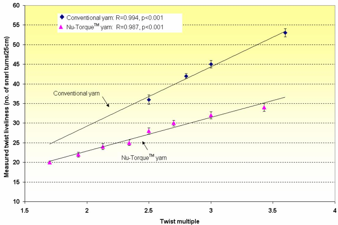
**Figure 4.2 Conventional and Nu-Torque yarn (29.5tex) measured twist liveliness vs twist multiple**
