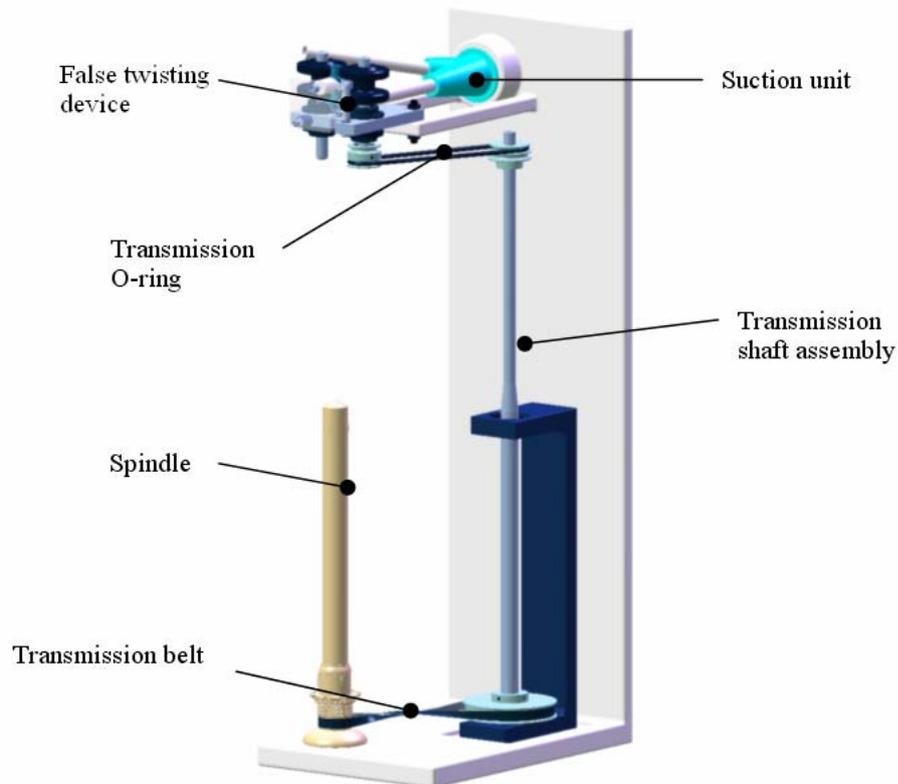
**Figure 4.1 Nu-Torque spinning system**
