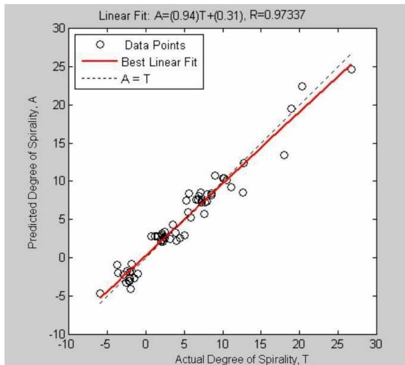
**Figure 5.10 Relationship between the actual and predicted values of spirality for the training set of data (neural network model)**
