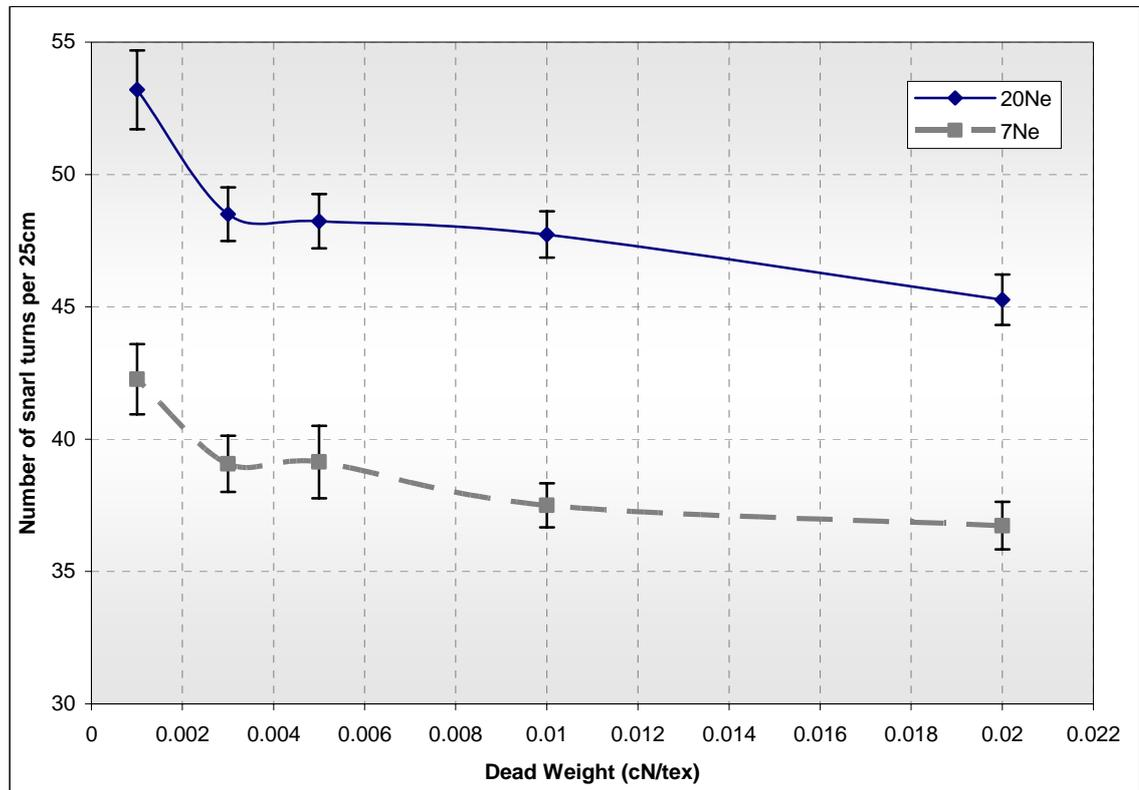
**Figure 3.11 Effect of dead weight on the number of snarl turns**
