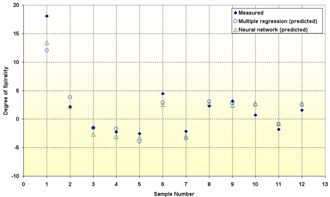
**Figure 5.11 Results of the multiple regression model and neural network model predictions and the actual measured degree of spirality for the test fabrics**
