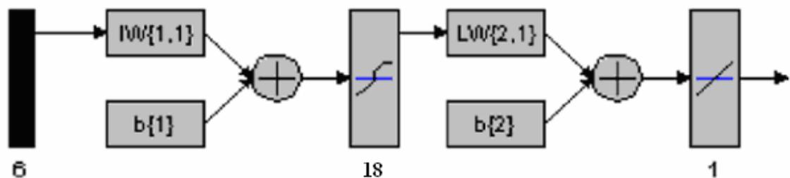
**Figure 5.9** Backpropagation neural network for spirality prediction
