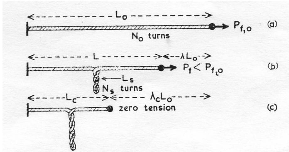
**Figure 2.3 Snarling in a twisted rod at reducing tension.  $\lambda$  is extension ratio**
