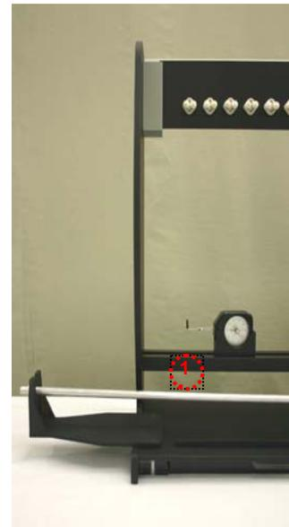
(4) The yarn package is moved in line with the pretension meter starting with position one
