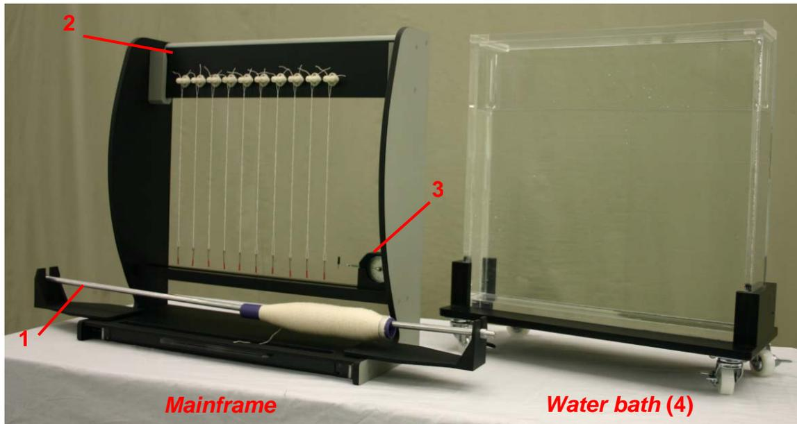
**Figure 3.2 The Yarn Snarling Apparatus**
