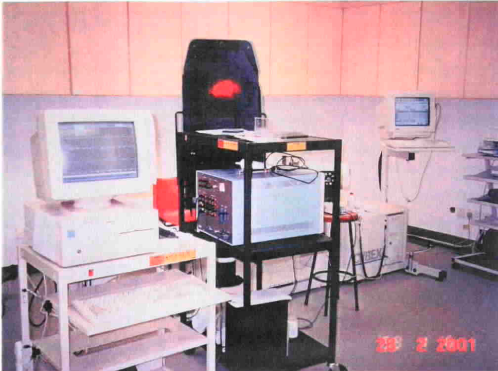
The complete setup consists of the computerized dynamometer (most right), the oscilloscope (middle) and the personal computer (left).
