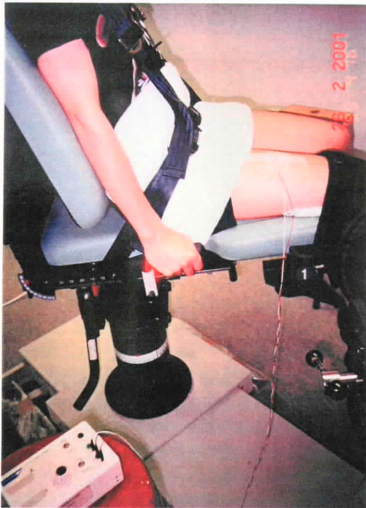
A close-up view of the position of the electrodes and the junction box (AVB-21) that contains the preamplifier
