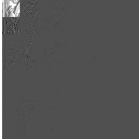
Figure 5.1: BDCT coefficients rearranged into a wavelet subband structure
