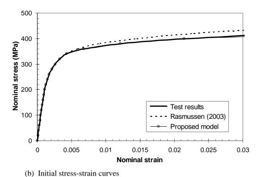
Figure A.12 Nominal stress-strain curves for the flat tension coupon cut from section SHS 100×100×8 tested by Gardner and Nethercot (2004).
