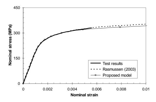
Figure 3.6 Nominal stress-strain curves for the longitudinal tension coupon cut from the ferritic stainless steel plate tested by Korvink *et al.* (1995).
