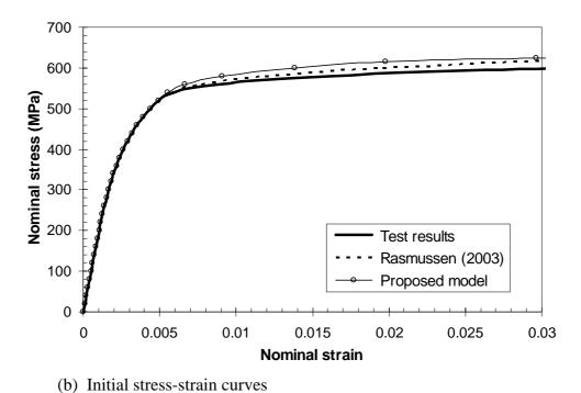
Figure A.20 Nominal stress-strain curves for the flat tension coupon cut from section RHS 120×80×6 tested by Gardner and Nethercot (2004).
