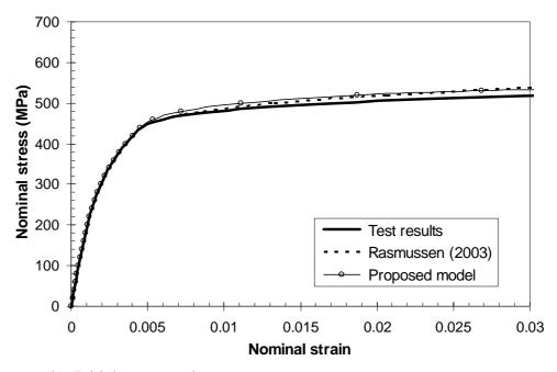
Figure A.18 Nominal stress-strain curves for the flat tension coupon cut from section RHS 120×80×3 tested by Gardner and Nethercot (2004).
