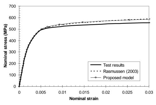
Figure A.28 Nominal stress-strain curves for the flat tension coupon cut from section RHS 100×50×4 tested by Gardner and Nethercot (2004).
