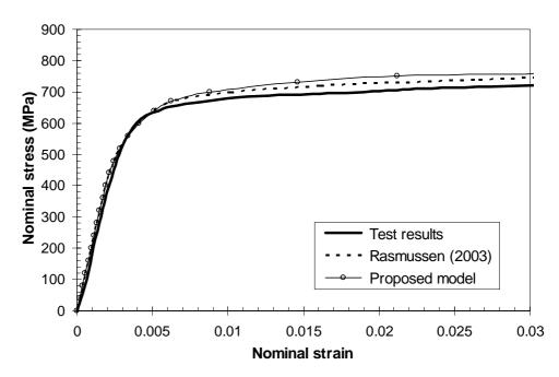
Figure A.34 Nominal stress-strain curves for the transverse tension coupon cut from the duplex stainless steel plate tested by Rasmussen *et al.* (2003).
