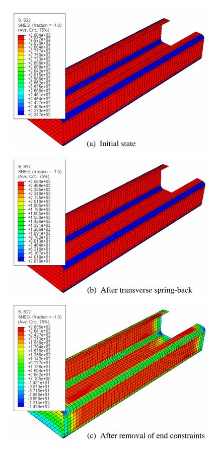
Figure 9.1 Longitudinal stress contours on the outer surface of the carbon steel stub column with D/t = 200 at different states of a nonlinear static analysis.
