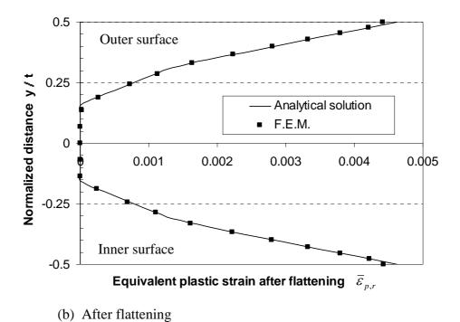
Figure 4.6 Comparison of equivalent plastic strains between the analytical solution and finite element analysis for the carbon steel sheet.
