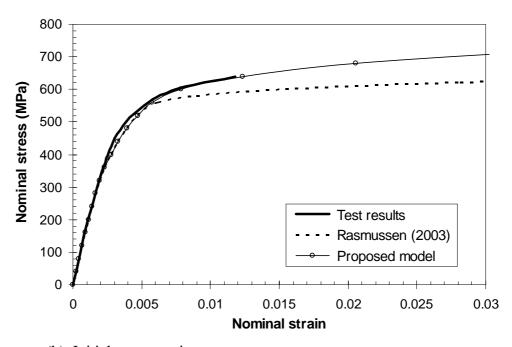
Figure A.33 Nominal stress-strain curves for the longitudinal compression coupon cut from the duplex stainless steel plate tested by Rasmussen *et al.* (2003).
