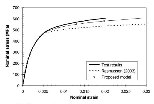
Figure A.9 Nominal stress-strain curves for the flat compression coupon cut from section SHS 100×100×4 tested by Gardner and Nethercot (2004).
