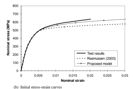
Figure A.21 Nominal stress-strain curves for the flat compression coupon cut from section RHS 120×80×6 tested by Gardner and Nethercot (2004).
