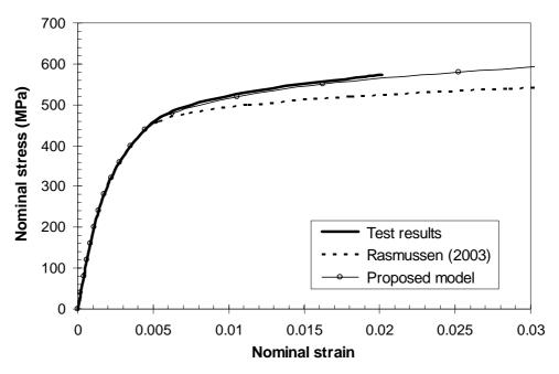
Figure A.19 Nominal stress-strain curves for the flat compression coupon cut from section RHS 120×80×3 tested by Gardner and Nethercot (2004).
