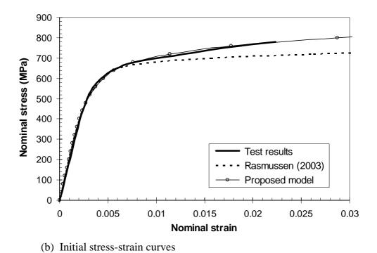
Figure A.35 Nominal stress-strain curves for the transverse compression coupon cut from the duplex stainless steel plate tested by Rasmussen *et al.* (2003).
