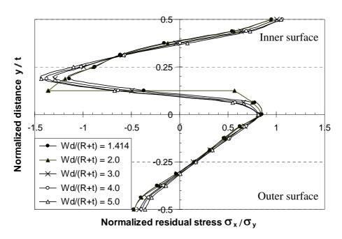
(b) Transverse residual stress (section A-A in Figure 5.10)
