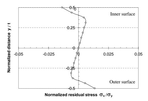
Figure 5.12 Through-thickness variations of residual stresses at the mid-web section of specimen PBC14 with D=1100 mm.
