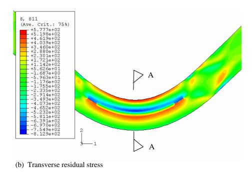
Figure 5.5 Stress contours in a 1-in. thick 90° cold-bent HY-80 steel plate.
