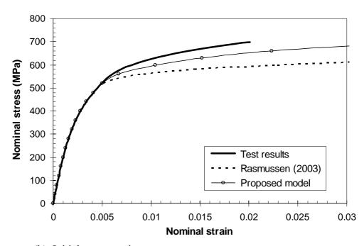
Figure A.31 Nominal stress-strain curves for the flat compression coupon cut from section RHS 100×50×6 tested by Gardner and Nethercot (2004).
