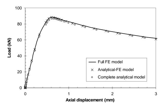
Figure C.7 Load-axial displacement curves for the stub column.
