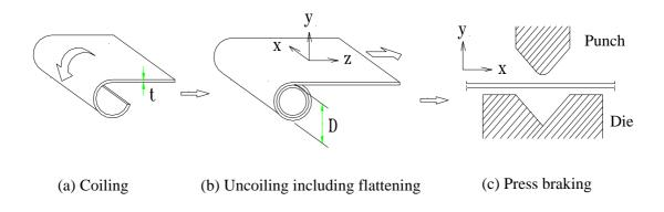
Figure 1.2 Manufacturing process of press-braked sections.
