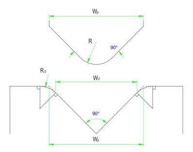
Figure 8.4 Dimensions of die and punch.
