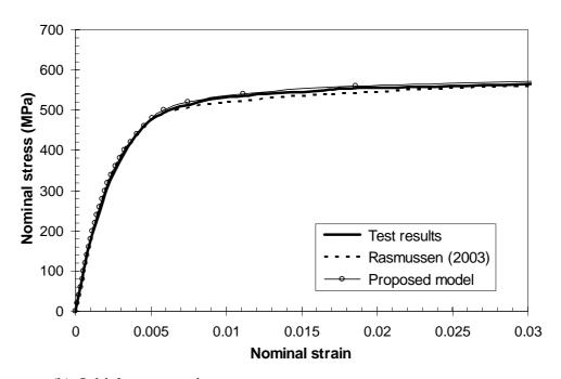
Figure A.1 Nominal stress-strain curves for the tension coupon cut from the thick lipped channel section tested by Macdonald *et al.* (2000).
