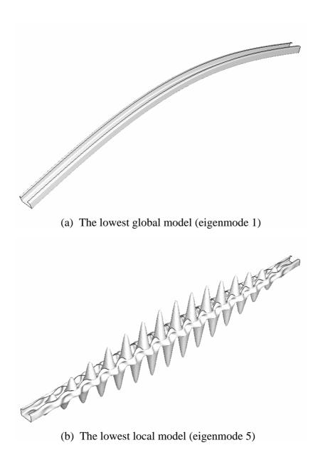
Figure 9.4 Eigenmodes for the 2000-mm high pin-ended carbon steel column.
