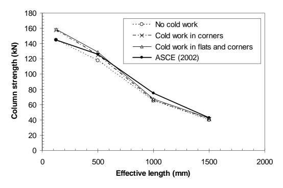
Figure 9.16 Comparison of column strengths between the advanced finite element approach (FEA) and the effective width method of the SEI/ASCE 8-02 specification (ASCE 2002) for fixed-ended stainless steel columns.
