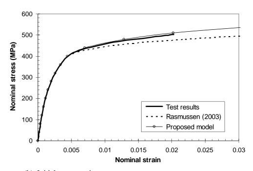
Figure A.7 Nominal stress-strain curves for the flat compression coupon cut from section SHS 100×100×3 tested by Gardner and Nethercot (2004).
