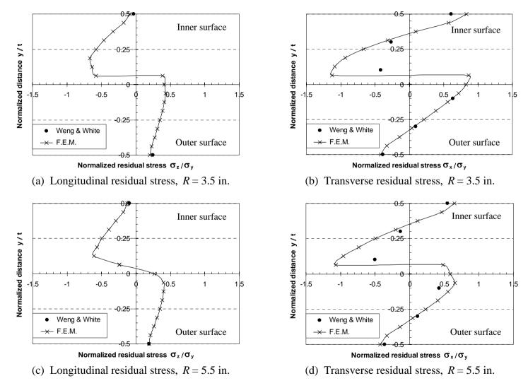
Figure 5.6 Comparison of finite element results with experimental results from Weng and White (continued).
