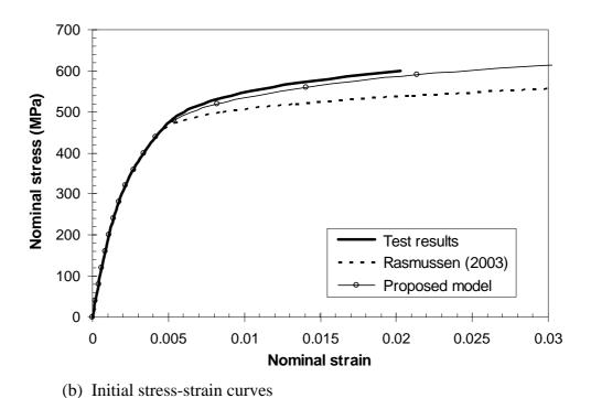
Figure A.29 Nominal stress-strain curves for the flat compression coupon cut from section RHS 100×50×4 tested by Gardner and Nethercot (2004).
