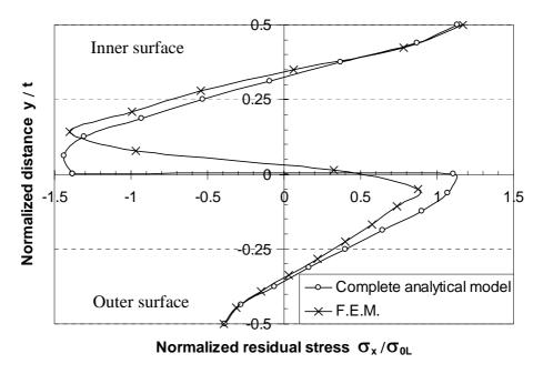
(b) Transverse residual stress at the center of the lip-flange corner (section A-A)
