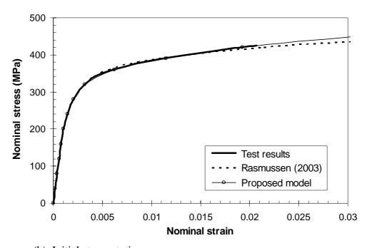
Figure A.13 Nominal stress-strain curves for the flat compression coupon cut from section SHS 100×100×8 tested by Gardner and Nethercot (2004).
