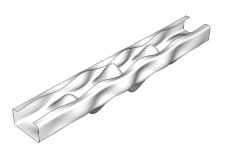
Figure 9.6 The first eigenmode for the 500-mm high pin-ended carbon steel column.
