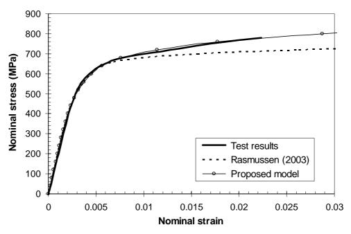
Figure 3.5 Nominal stress-strain curves for the transverse compression coupon cut from the duplex stainless steel plate tested by Rasmussen *et al.* (2002).
