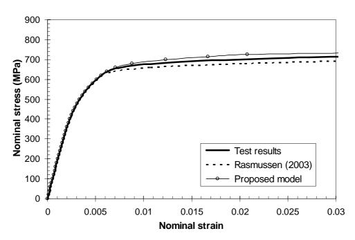
Figure A.30 Nominal stress-strain curves for the flat tension coupon cut from section RHS 100×50×6 tested by Gardner and Nethercot (2004).
