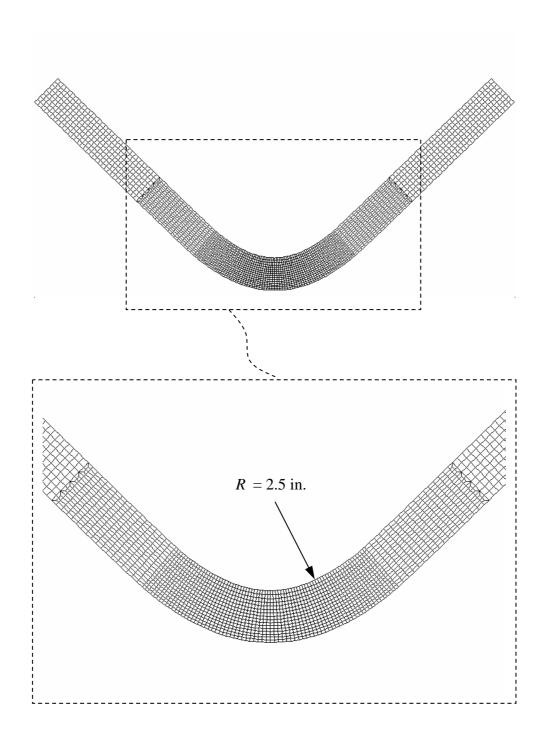
Figure 5.4 Deformed mesh for a 1-in. thick  $90^{\circ}$  cold-bent HY-80 steel plate.
