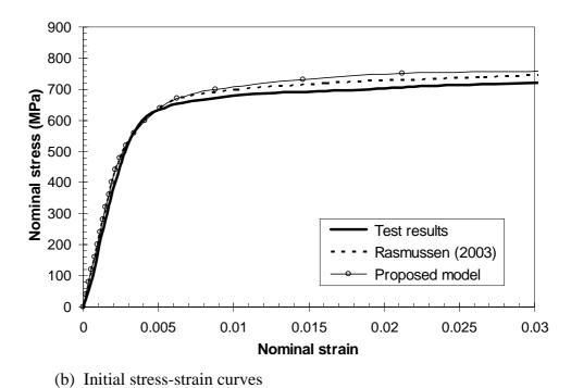
Figure 3.4 Nominal stress-strain curves for the transverse tension coupon cut from the duplex stainless steel plate tested by Rasmussen *et al.* (2002).
