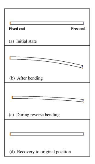
Figure 4.3 Pure bending of a flat strip.
