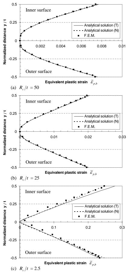
Figure 7.6 Comparison of equivalent plastic strains between the analytical solution and finite element analysis, for different  $R_c/t$  ratios.
