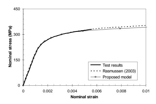
Figure A.36 Nominal stress-strain curves for the longitudinal tension coupon cut from the ferritic stainless steel plate tested by Korvink *et al.* (1995).
