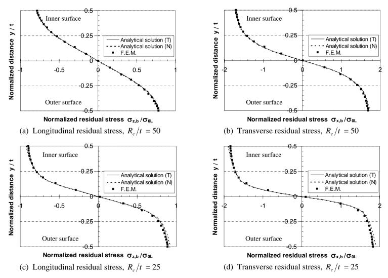
Figure 7.5 Comparison of residual stresses between the analytical solution and finite element analysis, for different  $R_c/t$  ratios.
