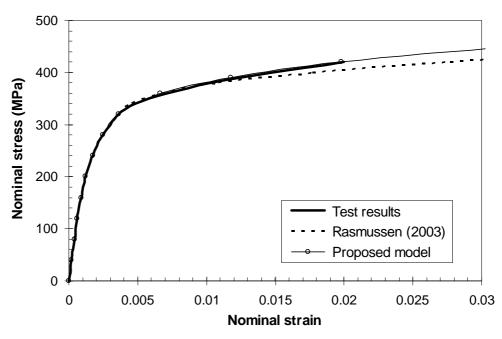
Figure A.23 Nominal stress-strain curves for the flat compression coupon cut from section RHS 150×100×4 tested by Gardner and Nethercot (2004).
