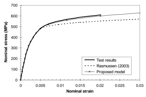
Figure 3.3 Nominal stress-strain curves for the flat compression coupon cut from section RHS 100×50×3 by Gardner and Nethercot (2004).
