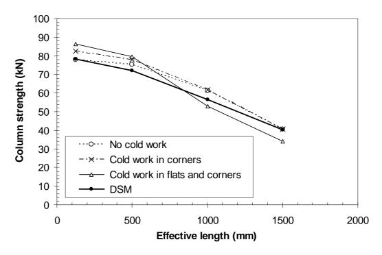
Figure 9.7 Comparison of column strengths between the advanced finite element approach (FEA) and the direct strength method (DSM) of the NAS (2001) specification for fixed-ended carbon steel columns.
