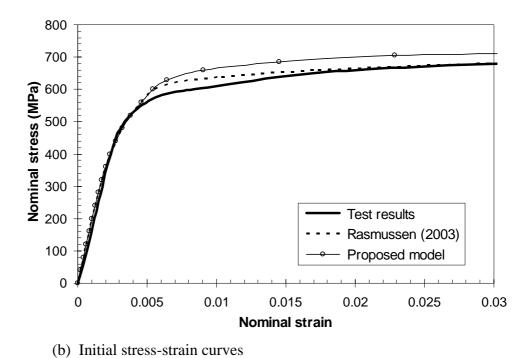
Figure A.32 Nominal stress-strain curves for the longitudinal tension coupon cut from the duplex stainless steel plate tested by Rasmussen *et al.* (2003).
