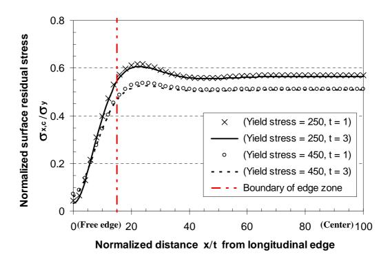
Figure B.1 Residual stresses on the outer surface after coiling.
