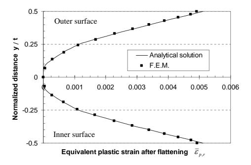
Figure 4.8 Comparison of equivalent plastic strains between the analytical solution and finite element analysis for the austenitic stainless steel sheet.
