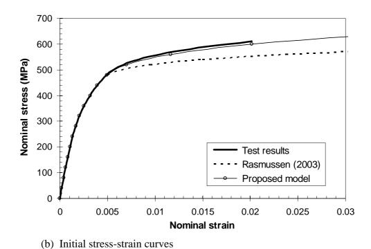
Figure A.27 Nominal stress-strain curves for the flat compression coupon cut from section RHS 100×50×3 tested by Gardner and Nethercot (2004).
