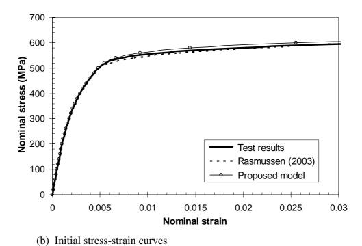
Figure 3.2 Nominal stress-strain curves for the flat tension coupon cut from section RHS 100×50×3 by Gardner and Nethercot (2004).
