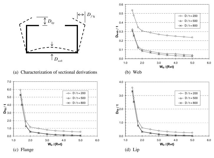
Figure 8.5 Effect of die size and coiling curvature on cross-sectional deviations of the carbon steel section.
