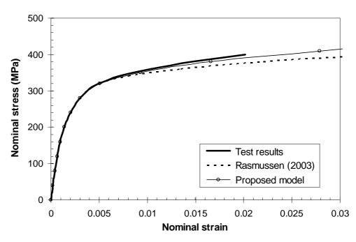
Figure A.15 Nominal stress-strain curves for the flat compression coupon cut from section SHS 150×150×4 tested by Gardner and Nethercot (2004).
