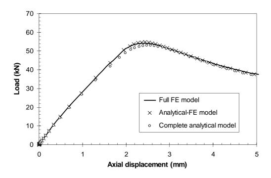
Figure C.9 Load-axial displacement curves for the 2000-mm high fixed-ended column.
