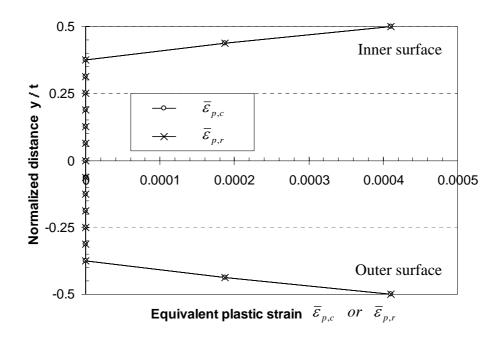
Figure 5.8 Equivalent plastic strains due to coiling and uncoiling in specimen PBC14 with  $D=1100~\mathrm{mm}$ .
