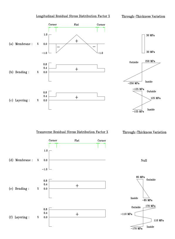
Figure 2.3 Idealized residual stress distributions in cold-formed steel square hollow sections (reproduced from Key and Hancock 1993).
