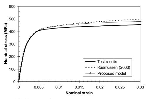
Figure A.6 Nominal stress-strain curves for the flat tension coupon cut from section SHS 100×100×3 tested by Gardner and Nethercot (2004).
