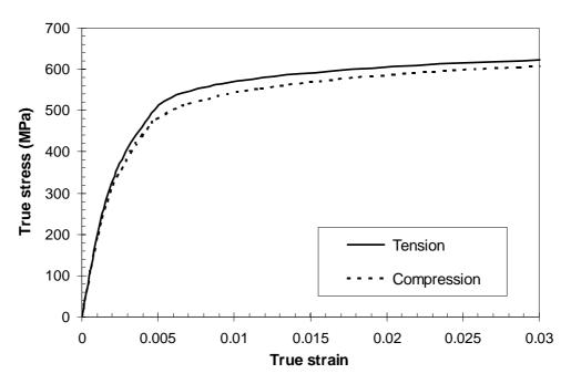
Figure 3.11 Typical true stress-strain curves for stainless steel defined by the 3-stage full-range stress-strain model.
