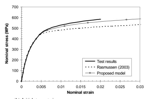
Figure A.3 Nominal stress-strain curves for the flat compression coupon cut from section SHS 80×80×4 tested by Gardner and Nethercot (2004).
