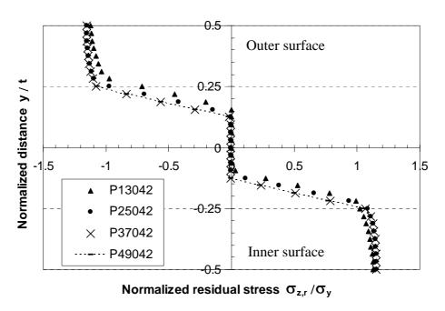
(b) Longitudinal residual stresses at points P13042 through P49042
