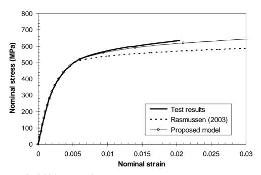
Figure A.11 Nominal stress-strain curves for the flat compression coupon cut from section SHS 100×100×6 tested by Gardner and Nethercot (2004).
