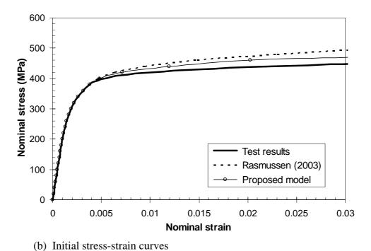
Figure A.4 Nominal stress-strain curves for the flat tension coupon cut from section SHS  $100 \times 100 \times 2$  tested by Gardner and Nethercot (2004).
