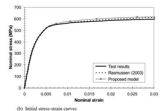
Figure A.10 Nominal stress-strain curves for the flat tension coupon cut from section SHS 100×100×6 tested by Gardner and Nethercot (2004).
