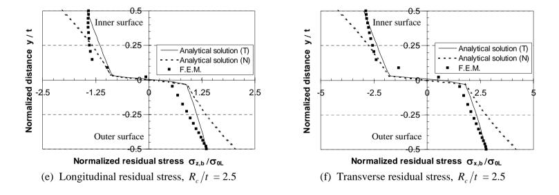
Figure 7.5 Comparison of residual stresses between the analytical solution and finite element analysis, for different  $R_c/t$  ratios (continued).
