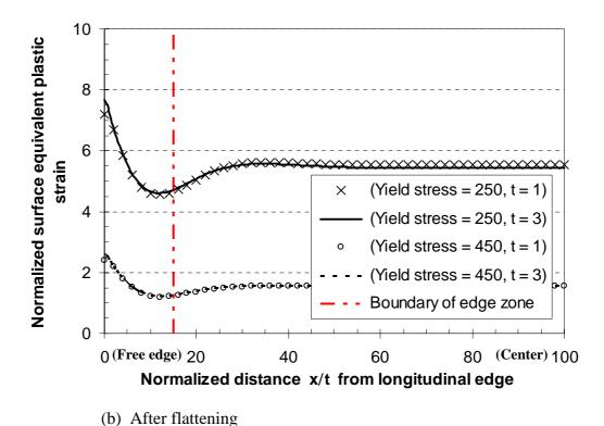
Figure B.3 Equivalent plastic strains on the outer surface due to coiling and uncoiling (including flattening).
