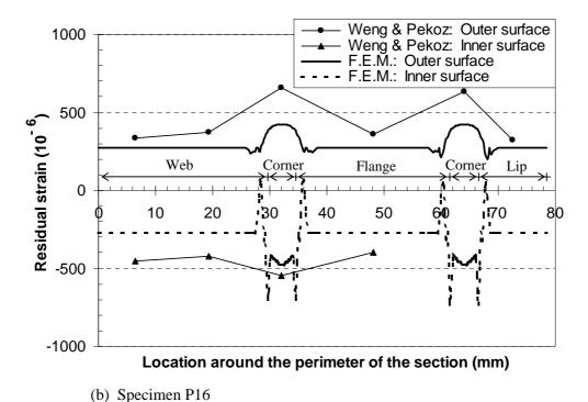
Figure 5.9 Longitudinal surface residual strain distributions in Weng and Peköz's sections with D = 1100 mm.
