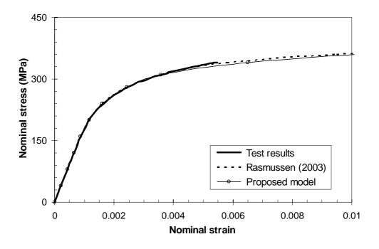
Figure 3.7 Nominal stress-strain curves for the longitudinal compression coupon cut from the ferritic stainless steel plate tested by Korvink *et al.* (1995).
