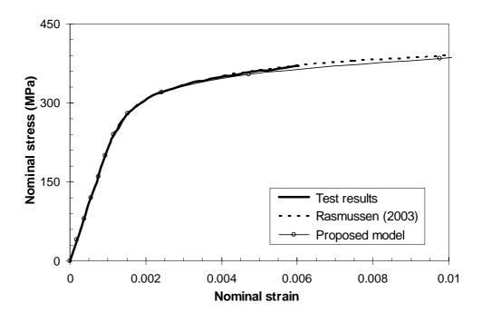
Figure A.39 Nominal stress-strain curves for the transverse compression coupon cut from the ferritic stainless steel plate tested by Korvink *et al.* (1995).
