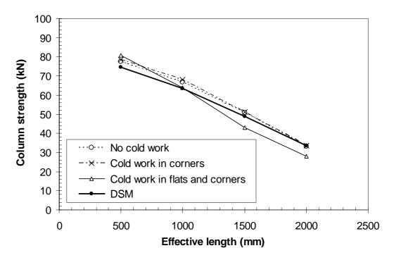
Figure 9.8 Comparison of column strengths between the advanced finite element approach (FEA) and the direct strength method (DSM) of the NAS (2001) specification for pin-ended carbon steel columns.
