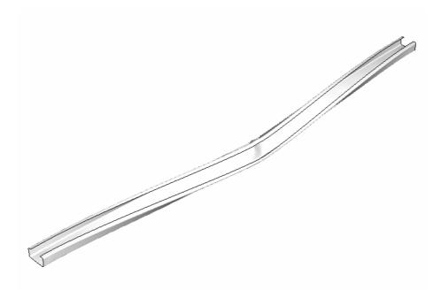
Figure 9.10 Post-failure deformed shape of the 2000-mm high fixed-ended carbon steel column with D/t=200.
