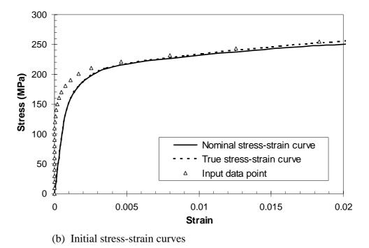
Figure 4.4 Stress-strain curves for the longitudinal tension of the austenitic stainless steel.
