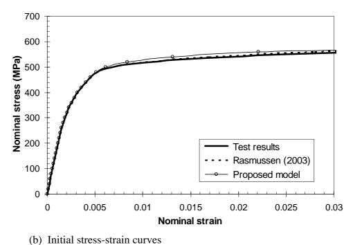
Figure A.2 Nominal stress-strain curves for the flat tension coupon cut from section SHS 80×80×4 tested by Gardner and Nethercot (2004).
