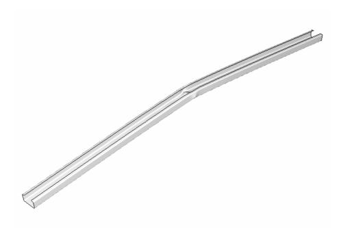
Figure 9.11 Post-failure deformed shape of the 2000-mm high pin-ended carbon steel column with D/t=200.
