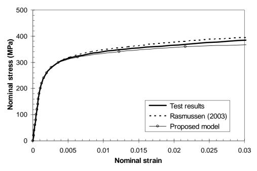
Figure A.22 Nominal stress-strain curves for the flat tension coupon cut from section RHS 150×100×4 tested by Gardner and Nethercot (2004).
