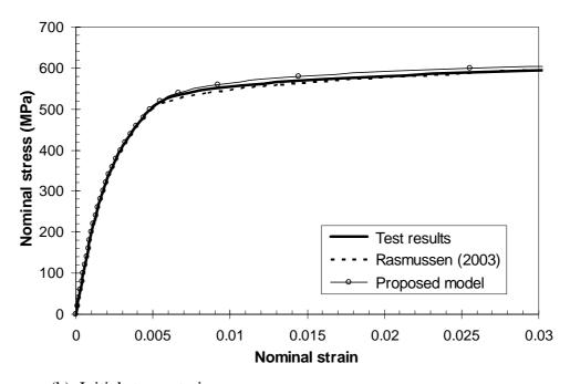
Figure A.26 Nominal stress-strain curves for the flat tension coupon cut from section RHS  $100 \times 50 \times 3$  tested by Gardner and Nethercot (2004).
