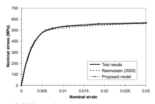
Figure 3.1 Nominal stress-strain curves for the tension coupon cut from the thick lipped channel section tested by Macdonald *et al.* (2000).
