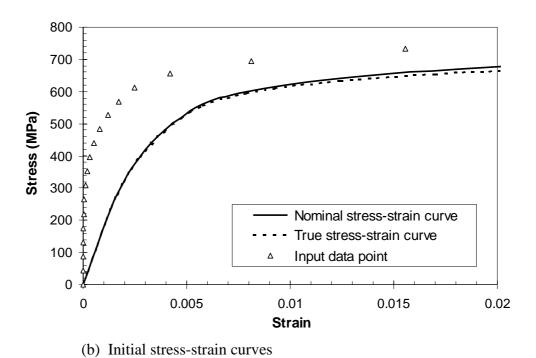
Figure 7.2 Stress-strain curves for longitudinal compression.
