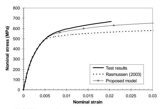
Figure A.17 Nominal stress-strain curves for the flat compression coupon cut from section RHS 60×40×4 tested by Gardner and Nethercot (2004).
