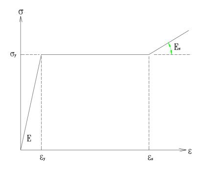
(a) Tri-linear elastic-plastic strain-hardening relationship for flat portions
