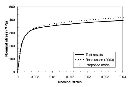
Figure A.14 Nominal stress-strain curves for the flat tension coupon cut from section SHS 150×150×4 tested by Gardner and Nethercot (2004).
