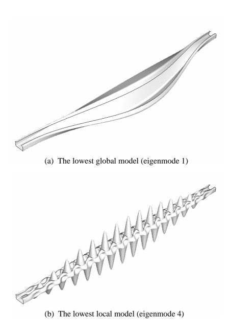
Figure 9.3 Eigenmodes for the 2000-mm high fixed-ended carbon steel column.
