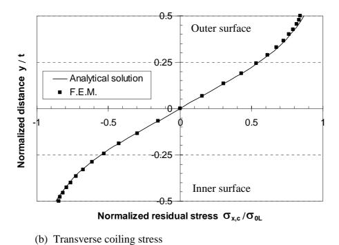
Figure 7.3 Comparison of residual stresses between the analytical solution and finite element analysis.
