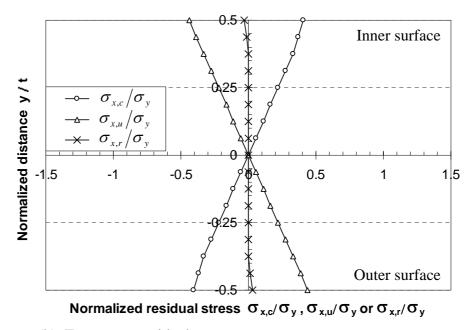
Figure 5.7 Residual stresses due to coiling and uncoiling in specimen PBC14 with  $D=1100~\mathrm{mm}$ .
