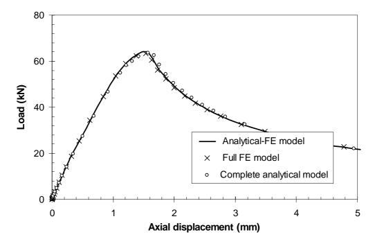
Figure C.10 Load-axial displacement curves for the 1000-mm high pin-ended column.
