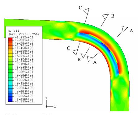
Figure 5.10 Stress contours in the lip-flange corner of specimen PBC14 with D = 1100 mm.
