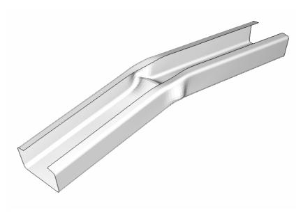
(b) Column with cold work in both flats and corners due to a coil diameter D = 200 t
