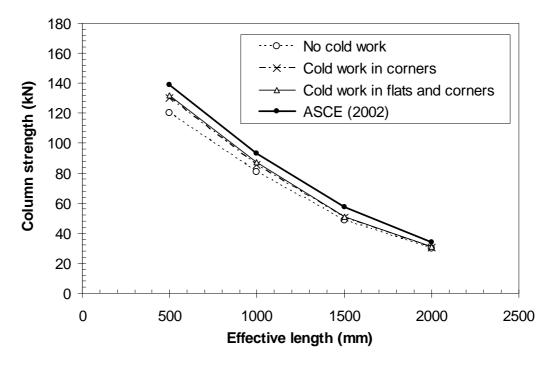
Figure 9.17 Comparison of column strengths between the advanced finite element approach (FEA) and the effective width method of the SEI/ASCE 8-02 specification (ASCE 2002) for pin-ended stainless steel columns.
