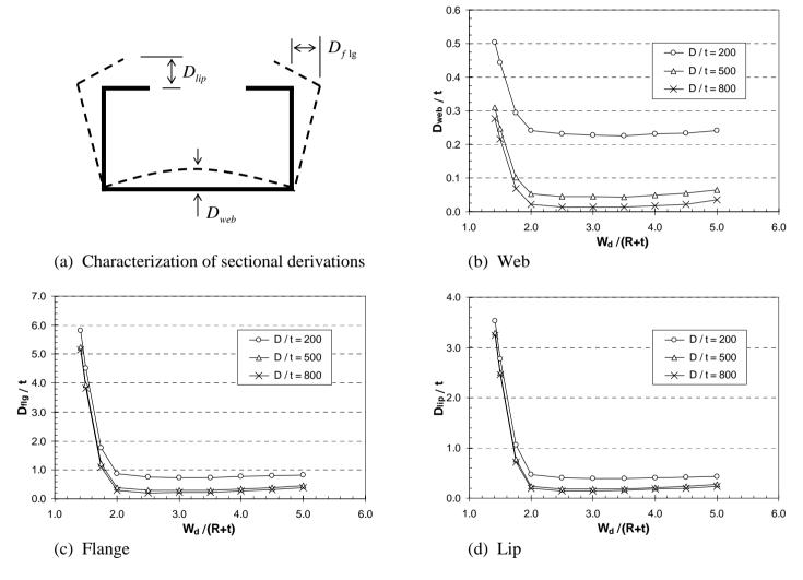
Figure 8.16 Effects of the die size and coiling curvature on cross-sectional deviations of the austenitic stainless steel section.
