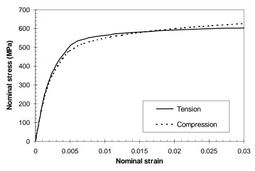
Figure 3.10 Typical nominal stress-strain curves for stainless steel defined by the 3-stage full-range stress-strain model.
