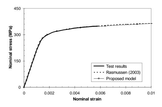
Figure A.38 Nominal stress-strain curves for the transverse tension coupon cut from the ferritic stainless steel plate tested by Korvink *et al.* (1995).
