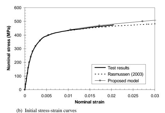
Figure A.25 Nominal stress-strain curves for the flat compression coupon cut from section RHS 100×50×2 tested by Gardner and Nethercot (2004).
