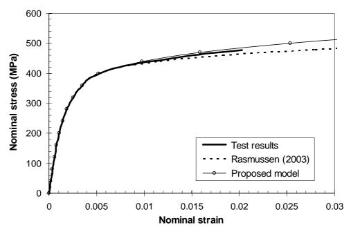
Figure A.5 Nominal stress-strain curves for the flat compression coupon cut from section SHS 100×100×2 tested by Gardner and Nethercot (2004).
