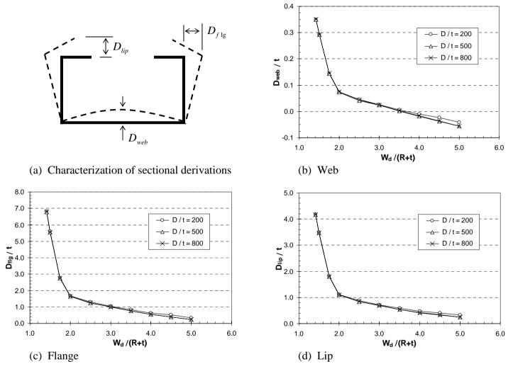
Figure 8.17 Effects of the die size and coiling curvature on cross-sectional deviations of the duplex stainless steel section.
