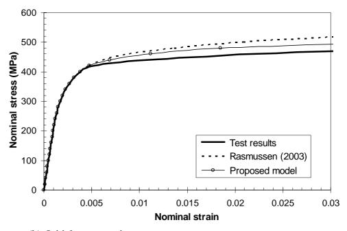
Figure A.24 Nominal stress-strain curves for the flat tension coupon cut from section RHS  $100 \times 50 \times 2$  tested by Gardner and Nethercot (2004).
