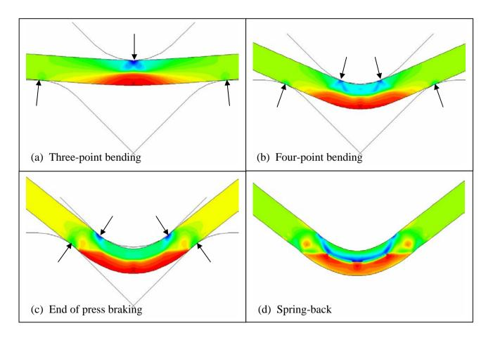
Figure 8.6 Deformation process and contact conditions of a 90° bent corner with a small die size  $(W_d = \sqrt{2}(R+t))$ .
