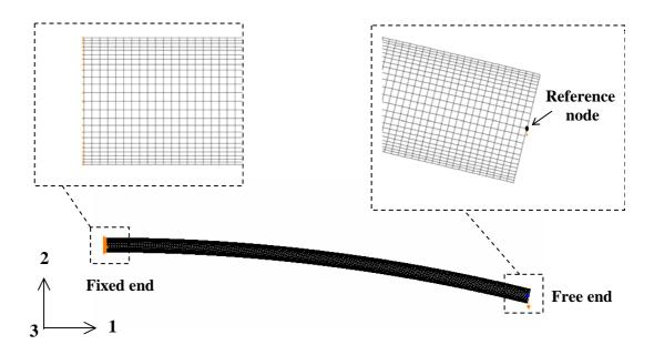
Figure 4.2 Mesh and boundary conditions.
