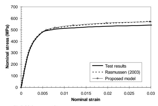
Figure A.8 Nominal stress-strain curves for the flat tension coupon cut from section SHS 100×100×4 tested by Gardner and Nethercot (2004).
