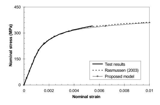
Figure A.37 Nominal stress-strain curves for the longitudinal compression coupon cut from the ferritic stainless steel plate tested by Korvink *et al.* (1995).
