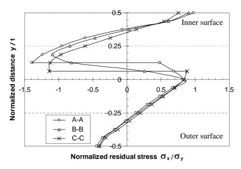
Figure 5.11 Through-thickness variations of residual stresses at different locations in the lip-flange corner of specimen PBC14.
