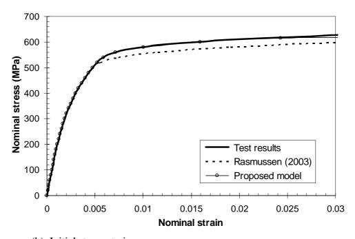
Figure A.16 Nominal stress-strain curves for the flat tension coupon cut from section RHS 60×40×4 tested by Gardner and Nethercot (2004).
