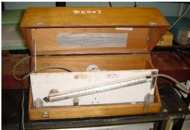
Instructions: The manometer may be used in a number of alternative positions. To move from one position to another, spring supporting tube slightly forward, and move into the required location. Level panel by two screws provided. After locating limb reset zero by rotating knob on panel. Do not force beyond limit of travel.
