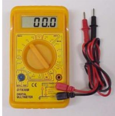
Fig. 3-7 A digital multi-meter for wattmeter calibration
