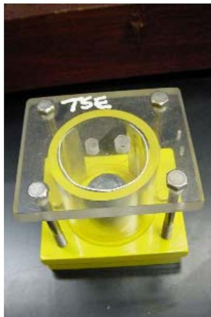
Fig. 3-6 Thermocouple calibrator
