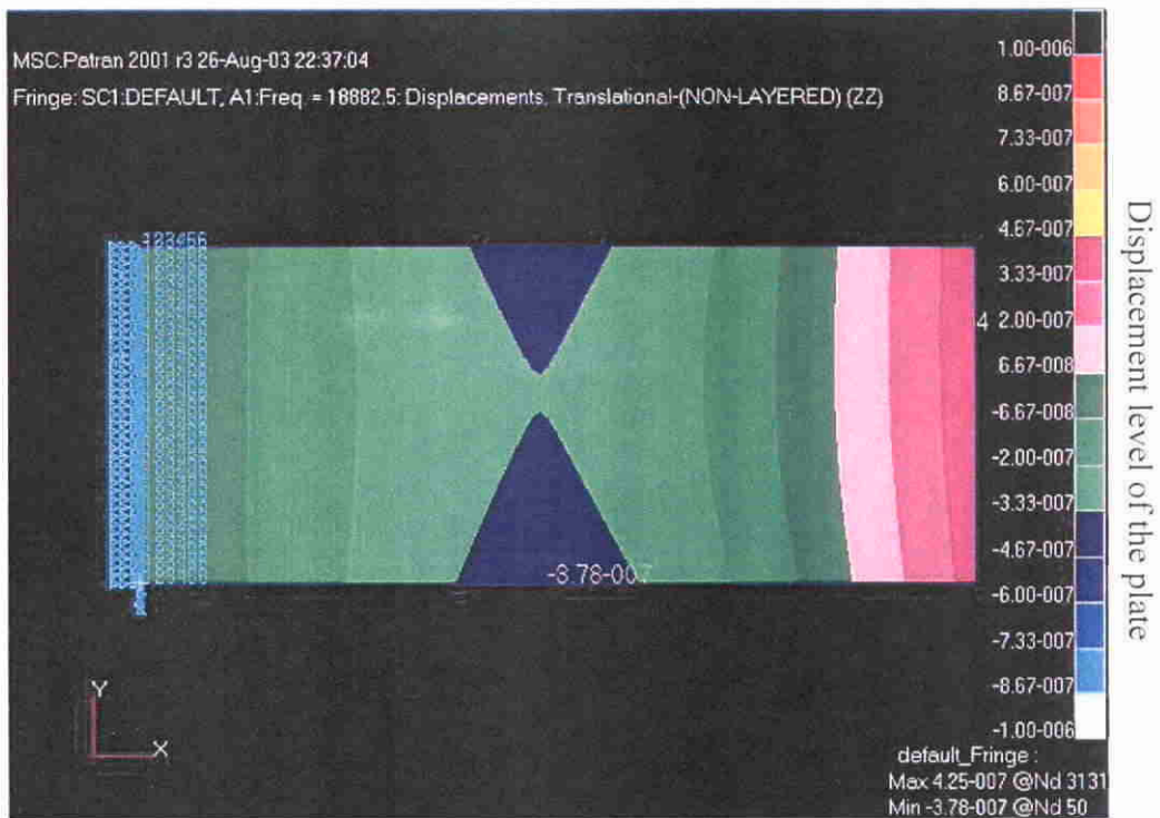
Figure 3.1.26. Vibration amplitude of the plate with Translational absorber
