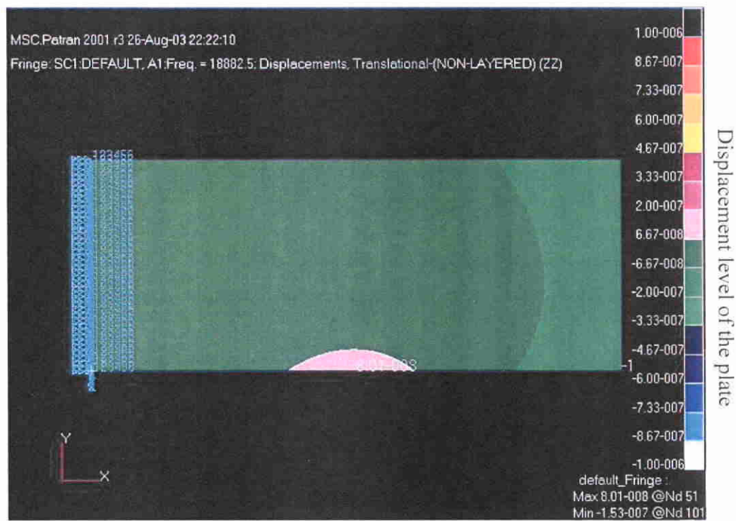
Figure 3.1.27. Vibration amplitude of the plate with Rotational absorber
