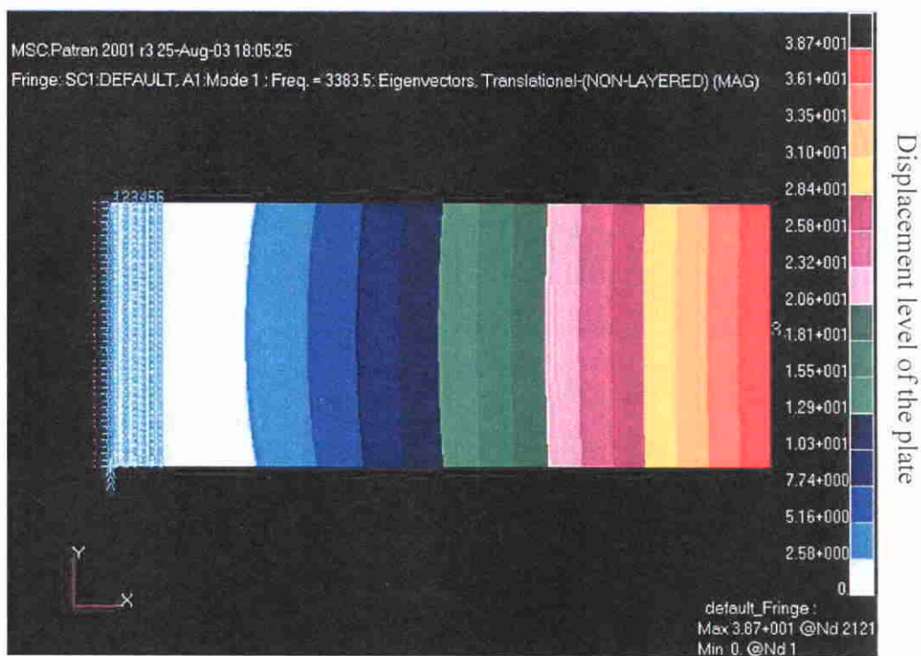
Figure 3.1.22. The first mode of the plate (The first beam mode)
