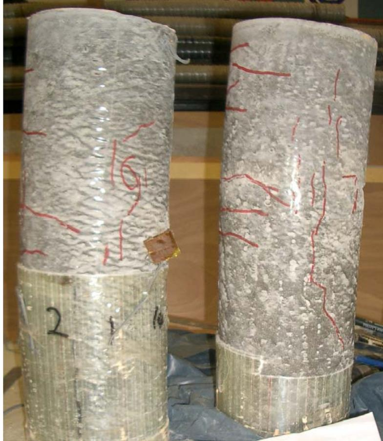
(c) Cracks on tension side
