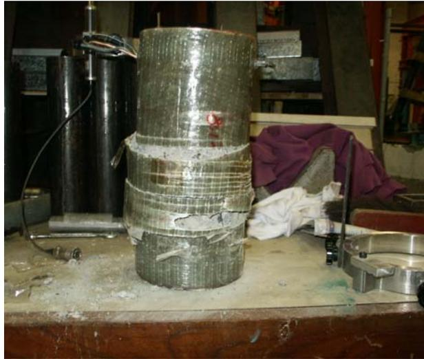
Figure 3.7 DSTC specimen after test
