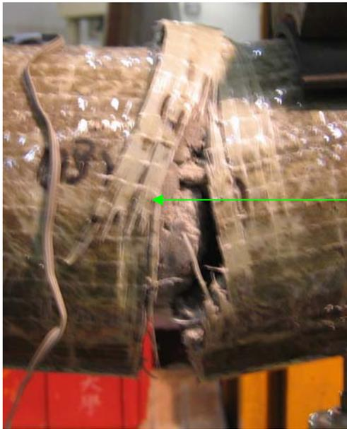
Rupture of the FRP tube in the compression zone due mainly to hoop tension
