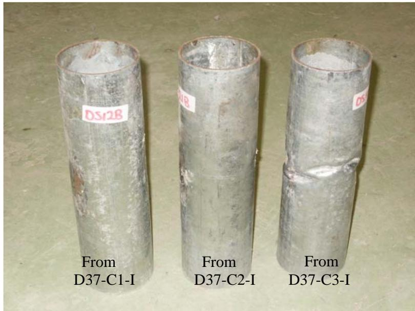
(a) Steel tubes from different DSTCs
