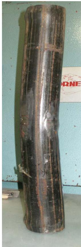
Figure 7.2 Buckling of hollow steel tube
