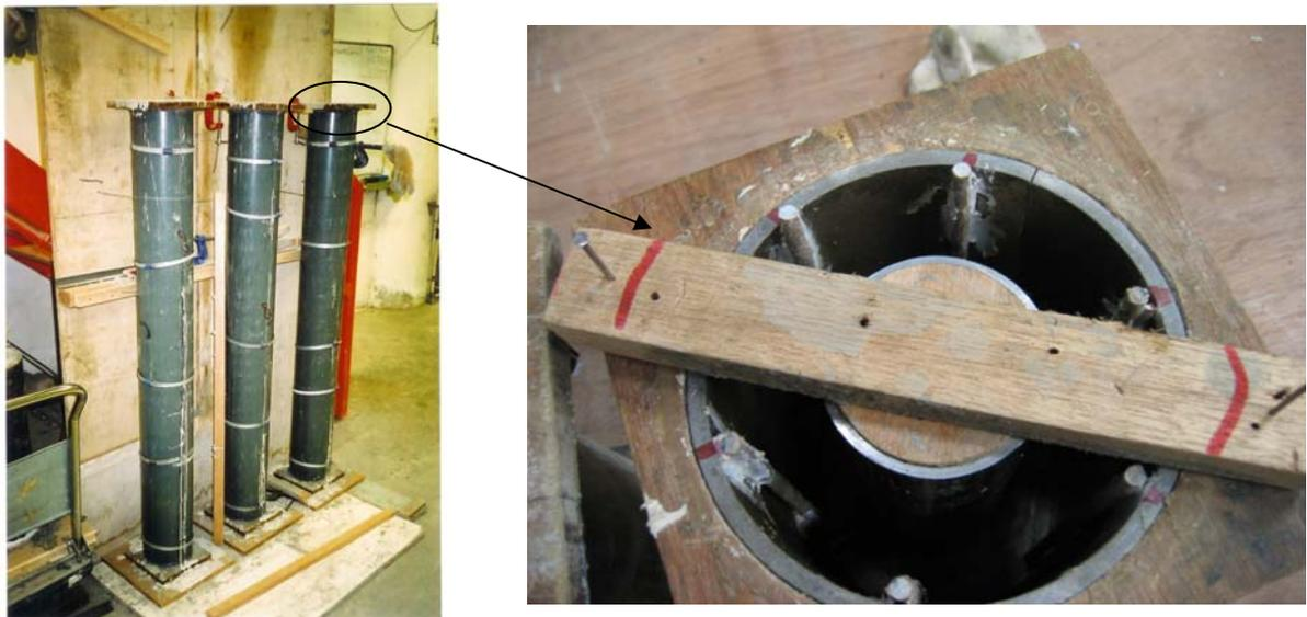
Figure 6.4 Formwork for casting concrete
