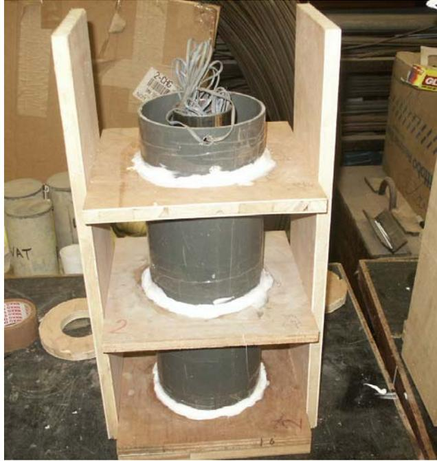
Figure 7.1 Form for casting concrete
