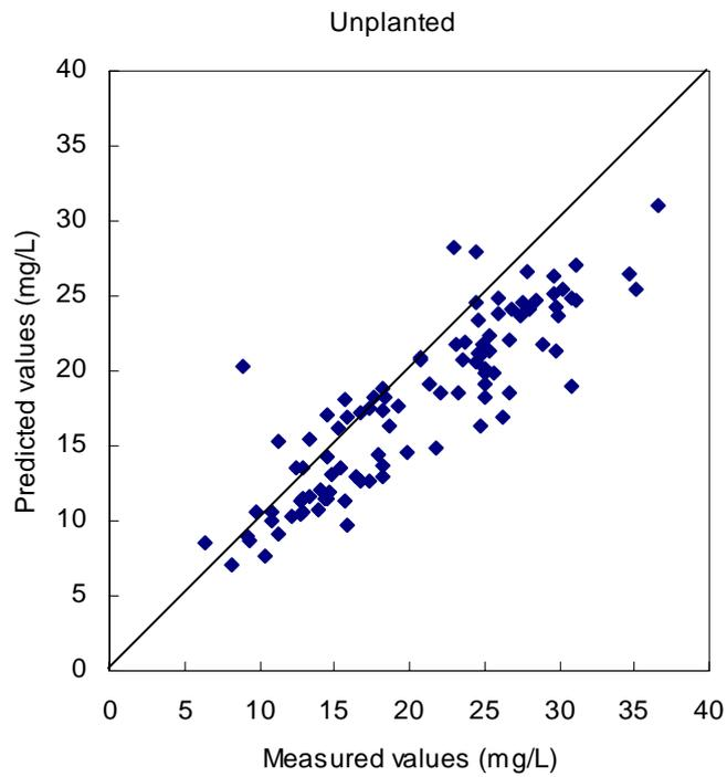
Figs. 5.2 show the fitness of the measured effluent concentrations with the predicted effluent concentrations from the first-order kinetics model.
