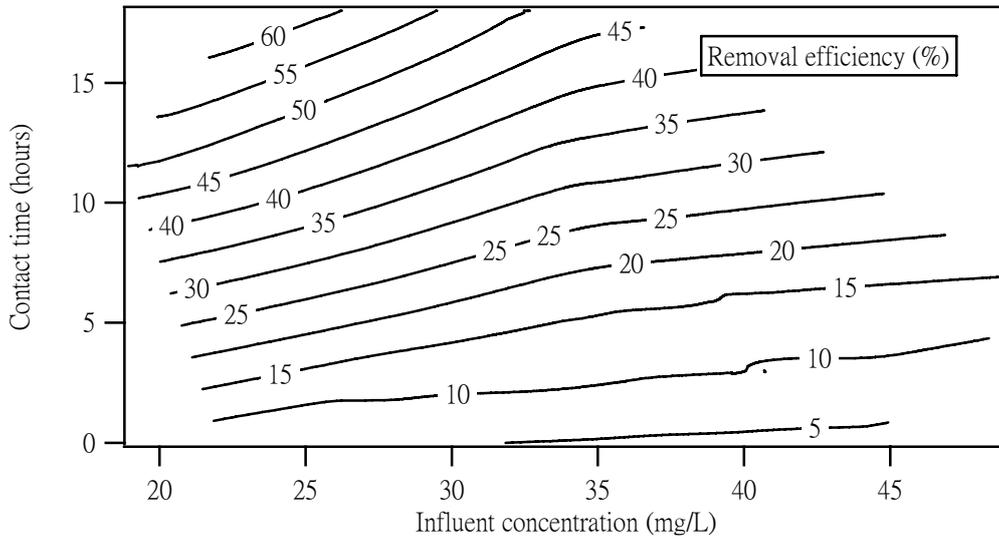
Fig. 6.1 Contour plot for ammonia nitrogen removal prediction at sewage temperature in a range of  $9.8\text{ }^{\circ}\text{C} < T < 20\text{ }^{\circ}\text{C}$ .
