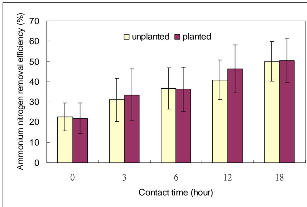
Fig. 4.15  $\text{NH}_3\text{-N}$  removal efficiency in the planted and the unplanted systems with different contact times in the pilot experiment
