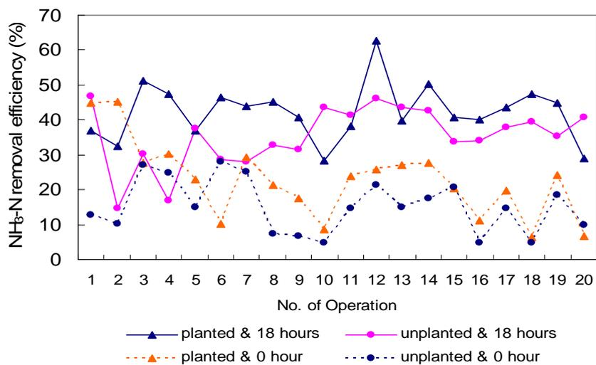
Fig. 4.8 NH<sub>3</sub>-N removal efficiency in laboratory-scale system.
