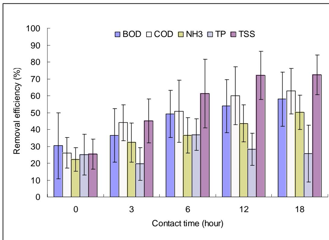
Fig. 4.20 Effects of contact time on different pollutant removal efficiencies in the pilot-scale system.
