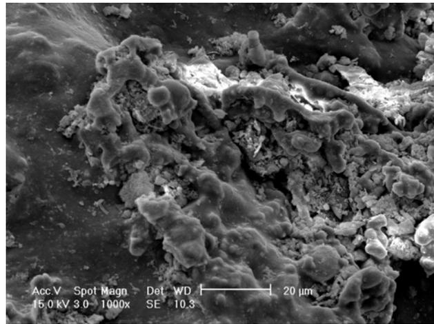
Figs. 4.12 Biofilm formed on the surface of coal slag
