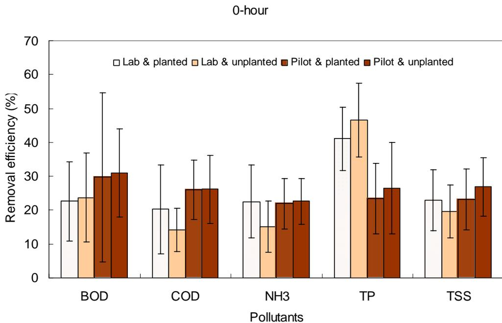
Fig. 4.28 Comparison of removal efficiencies of different pollutants in laboratory-scale and pilot-scale experiments in 0-hour contact time.
