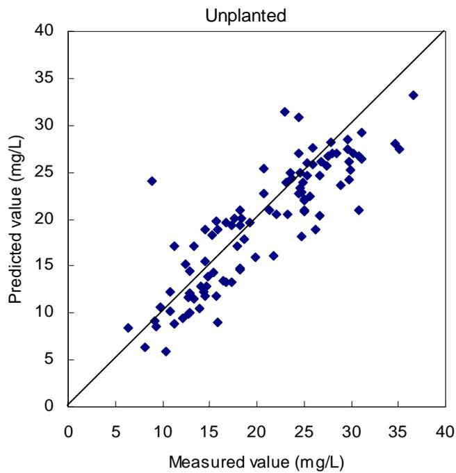
Figs. 5.1 show the fitness of the measured effluent concentrations with the predicted effluent concentrations from multivariate regression model.
