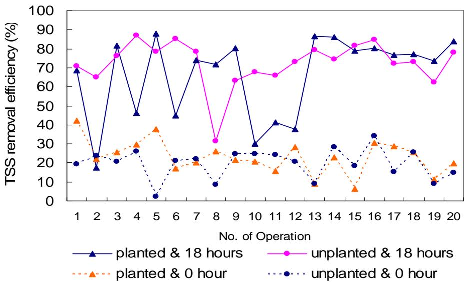
Fig. 4.10 TSS removal efficiency in laboratory-scale system.
