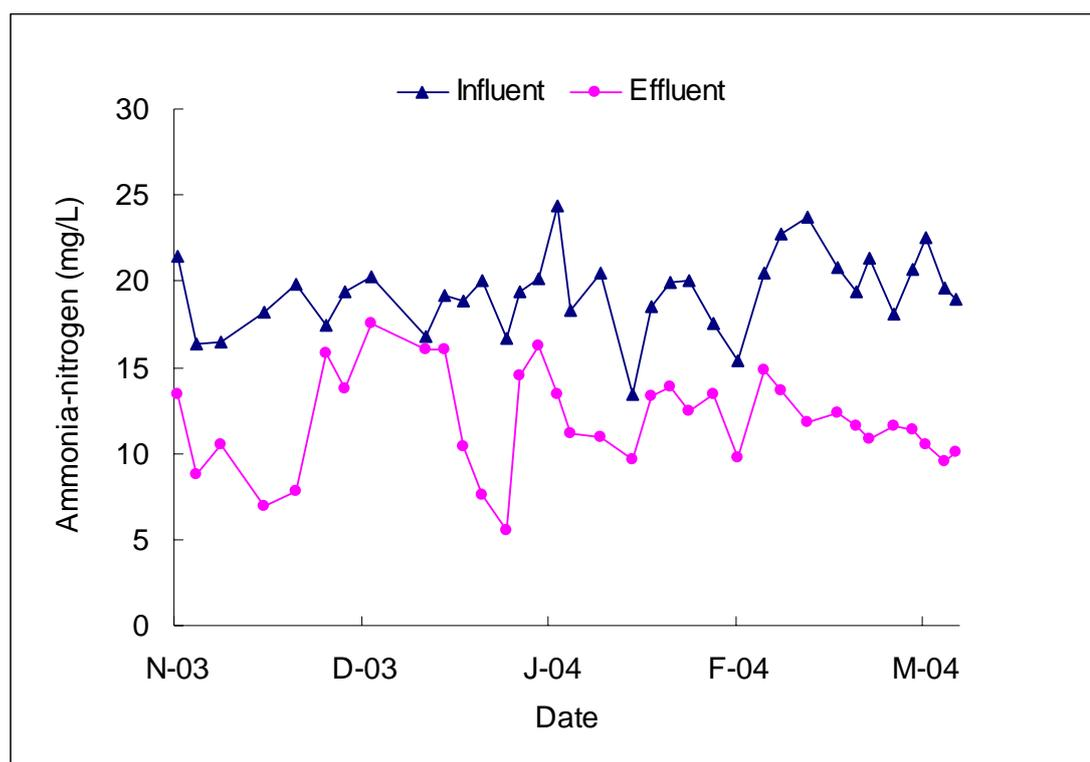
Fig. 4.5 Start-up period of laboratory-scale system (reflected by ammonia nitrogen concentrations)
