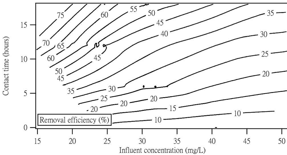
Fig. 6.2 Contour plot for ammonia nitrogen removal prediction at sewage temperature in a range of  $20.0\text{ }^{\circ}\text{C} \leq T < 35\text{ }^{\circ}\text{C}$ .
