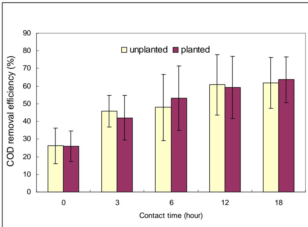
Fig. 4.17 COD removal efficiency in the planted and the unplanted systems with different contact times in the pilot experiment
