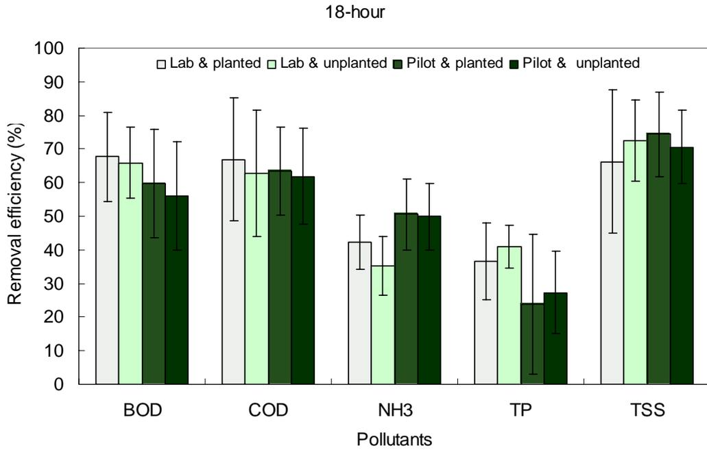
Fig. 4.27 Comparison of removal efficiencies of different pollutants in laboratory-scale and pilot-scale experiments in 18-hour contact time.
