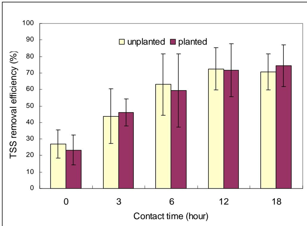
Fig. 4.19 TSS removal efficiency in the planted and the unplanted systems with different contact times in the pilot experiment
