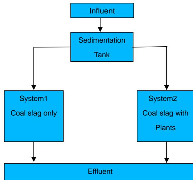
Fig. 3.5 Schematic flow of the pilot-scale systems
