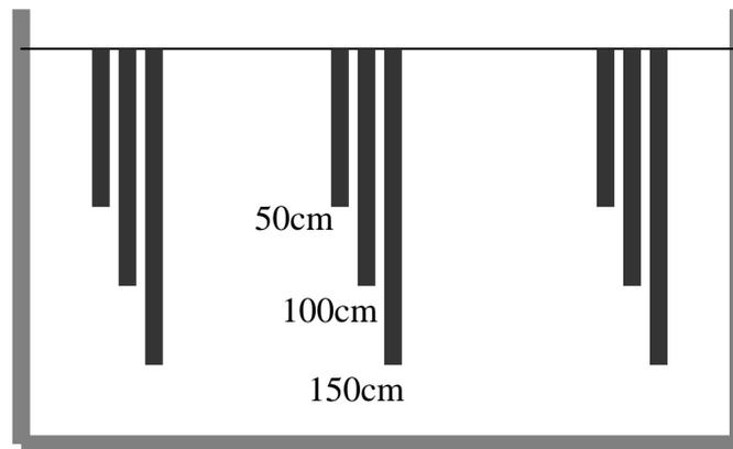
Fig. 3.8 Depths of hollow pipes for D.O. measurement (side view).
