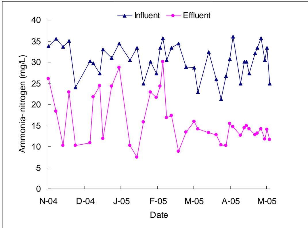
Fig. 4.11 Start-up period of the pilot-scale system (reflected by ammonia nitrogen concentrations)
