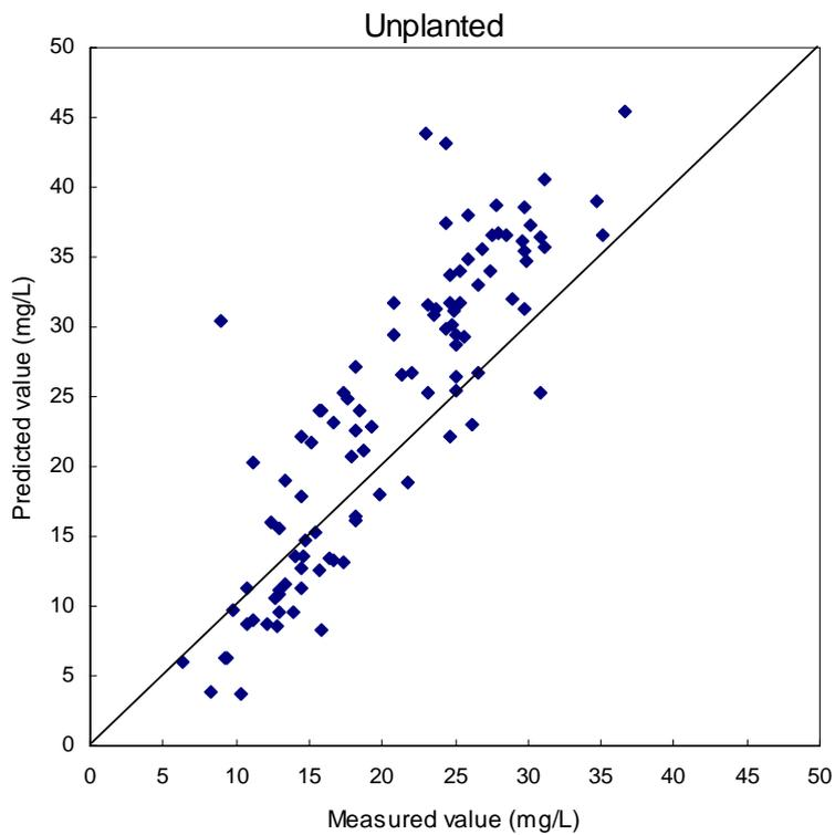
Figs. 5.3 show the fitness of the measured effluent concentrations with the predicted effluent concentrations from the mass balance model.
