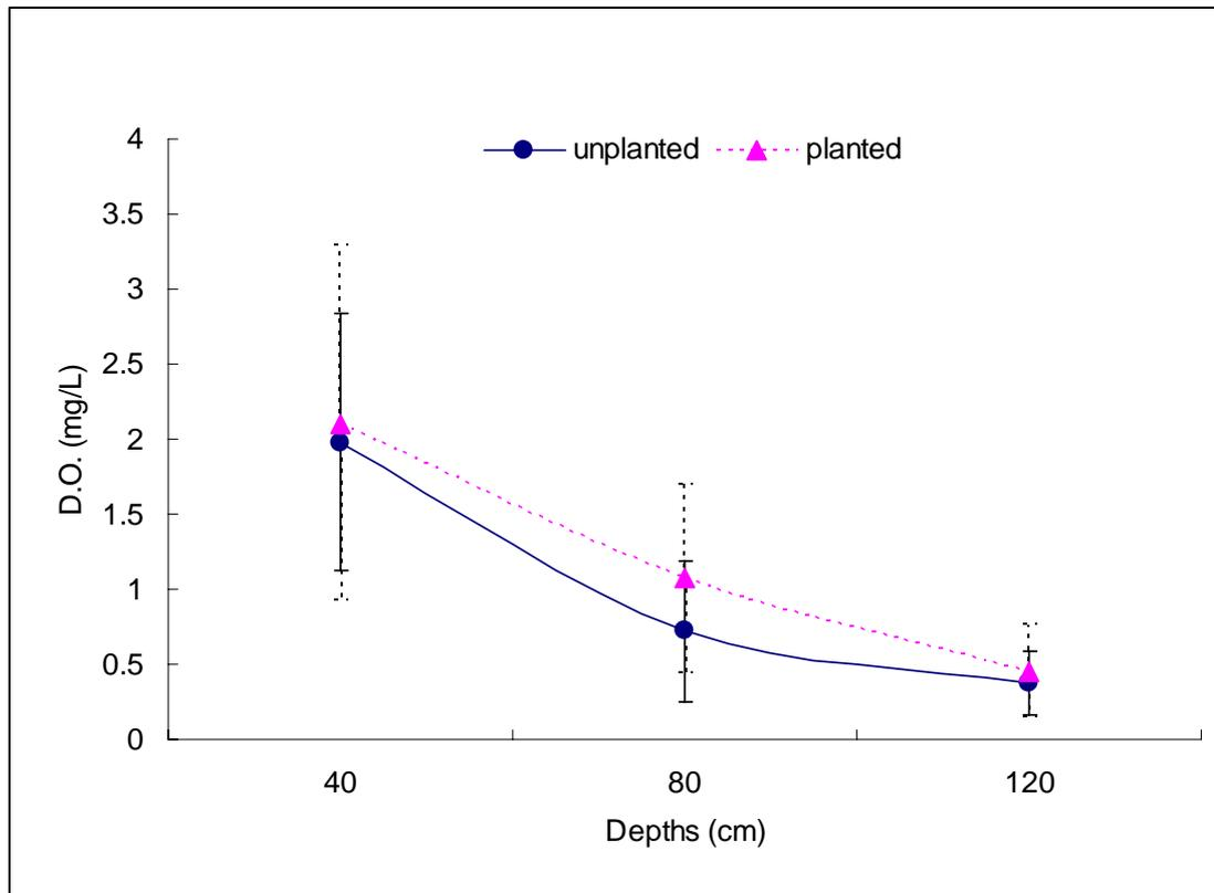
Fig. 4.21 D.O. levels in different depths of planted and unplanted systems
