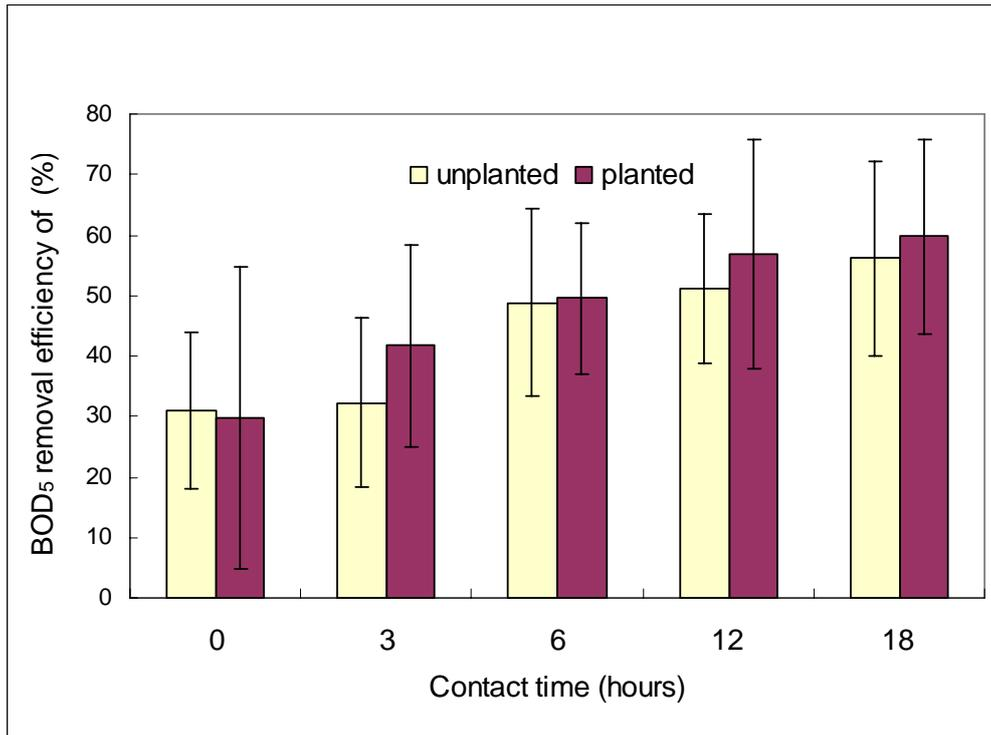
Fig. 4.16 BOD<sub>5</sub> removal efficiency in the planted and the unplanted systems with different contact times in the pilot experiment
