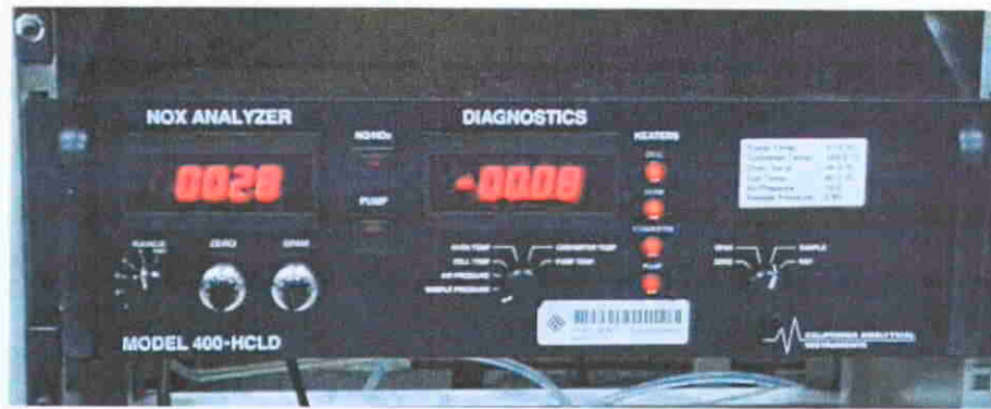
Figure 4.7 Heated chemiluminescence NO x gas analyser.
