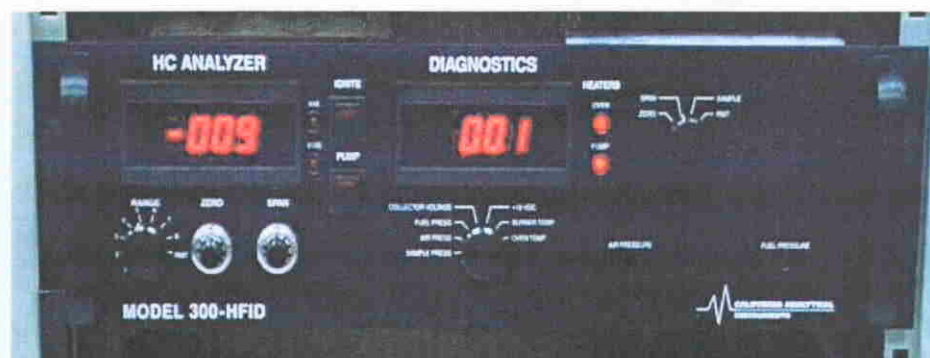
Figure 4.6 Heated flame ionisation detection HC gas analyser.
