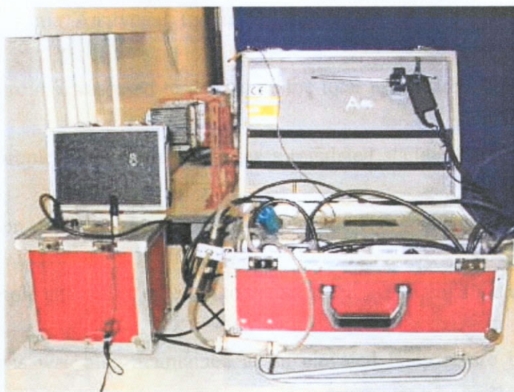
Figure 4.5 Non-dispersive infra-red CO and CO 2 gas analyser.
