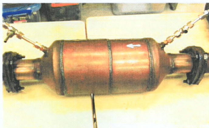
Figure 4.12b A platinum-based diesel oxidation catalyst (DOC-Type B).
