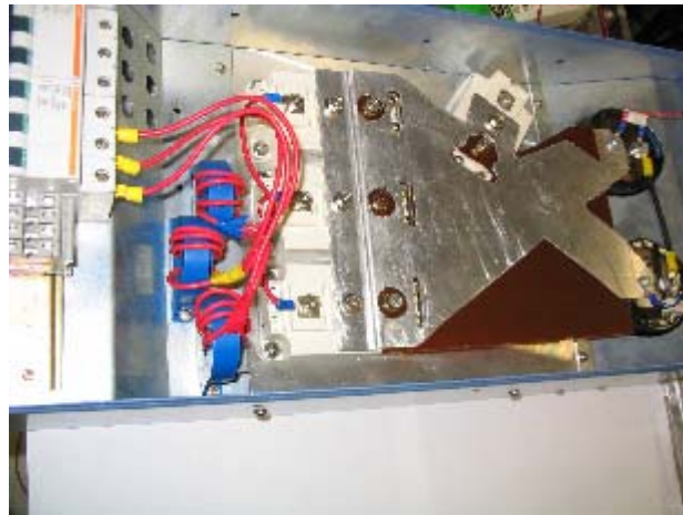
Figure A.8.1 The main circuit of the proposed SAPF in the laboratory system
