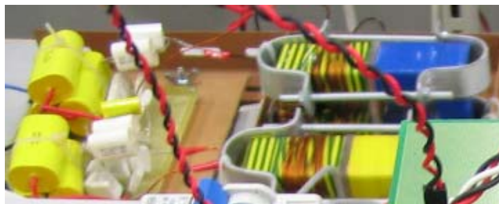
Figure A.8.2 The switching ripple filter used in the laboratory system
