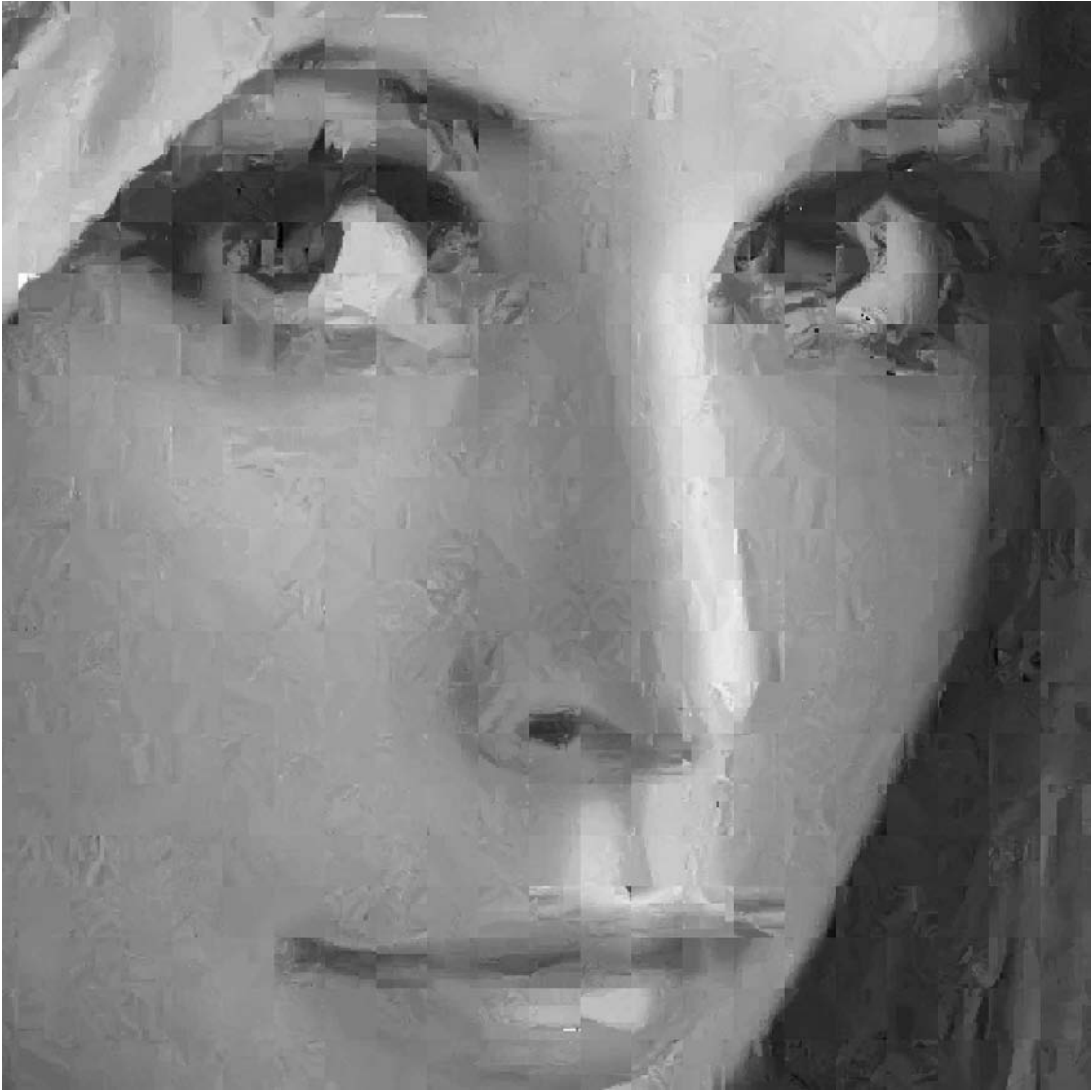
Figure 9-1 Traditional Fractal magnification Algorithm with magnification factor \alpha=8
