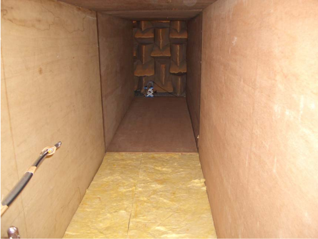
FIG. 3.10 The model corridor with a single impedance discontinuity.
