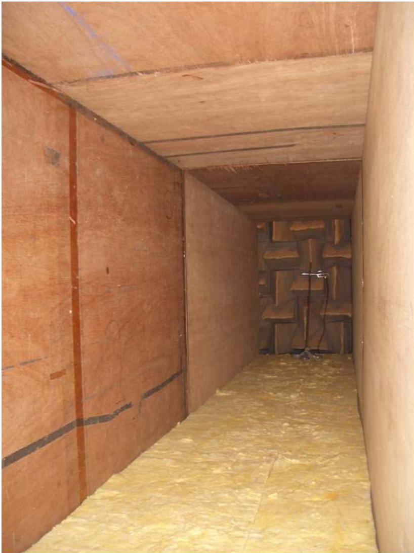
FIG. 2.15: Model corridor in the anechoic chamber.
