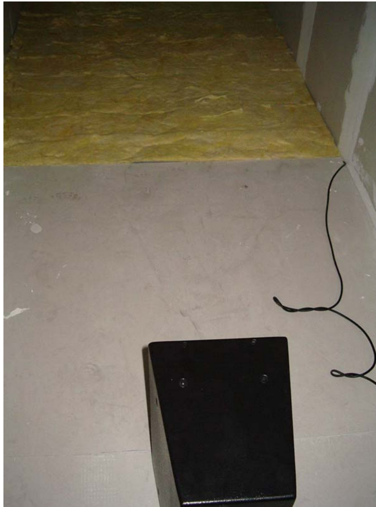
FIG. 3.13: The loud speaker placed inside the model tunnel with a single impedance discontinuity.
