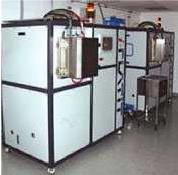
Figure 1.9: PLATIT PL 50 Cathodic Arc Physical Vapor Deposition (CAPVD) system
