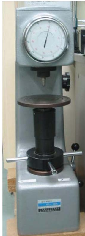
Figure 4.7: Hardness indenter used for checking goodness of coating adhesion.
