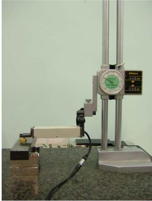
Figure 4.12 Surface profilometer for measuring coating  $R_a$  value.
