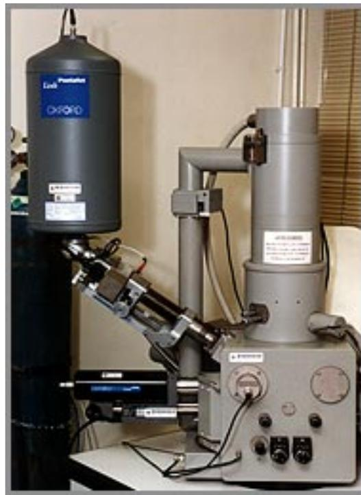
Figure 4.13: SEM for surface morphology (The Hong Kong Polytechnic University Materials Research Centre (MRC)).
