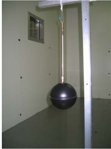
Fig. 7.6 A globe thermometer at 0.6 m height in the air conditioned room
