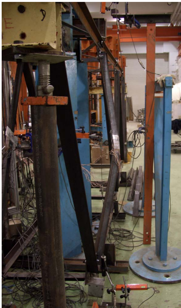
Figure 7.7 Weak-axis buckling (webs on same side, double-bolted)
