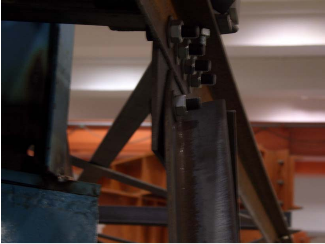
Figure 7.6 Rotation of the specimen at the connection (webs on same side, single-bolted)
