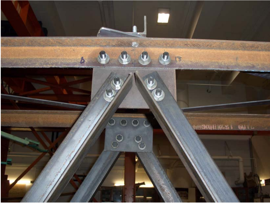
Figure 7.2 Connection details (web on same side, double-bolted)
