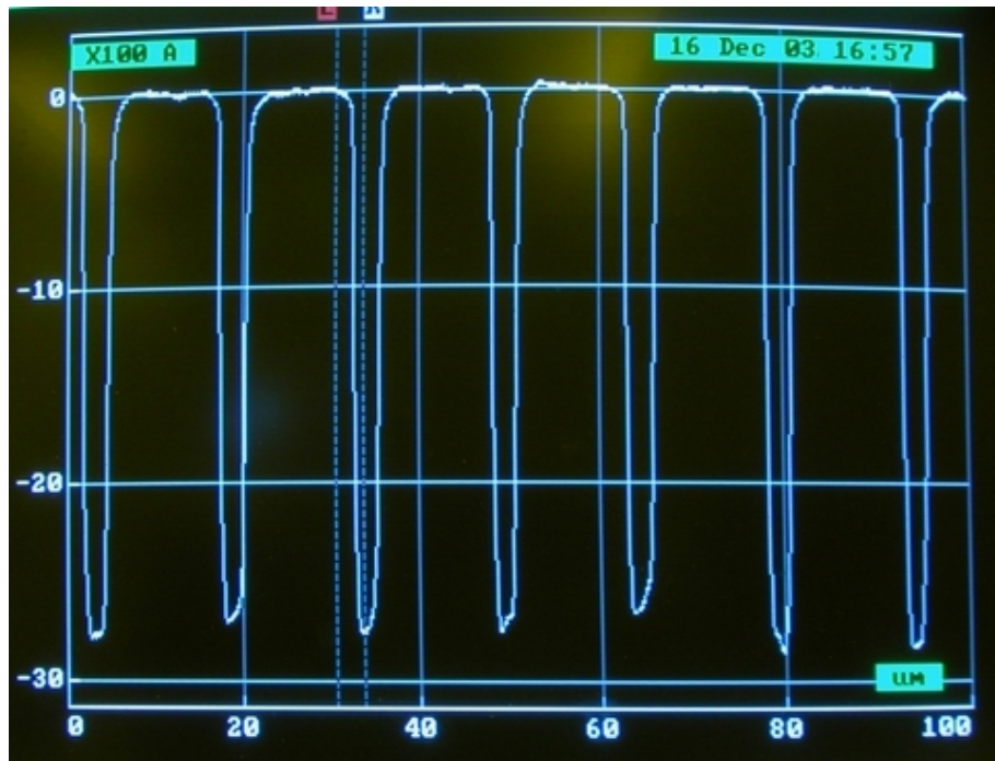
Figure 4.2 \alpha -Step profile of a typical PEC wet etching with holes as pattern
