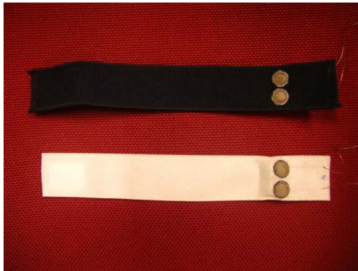
Figure 57 Inner part of the wristband with 2 fabric electrodes
