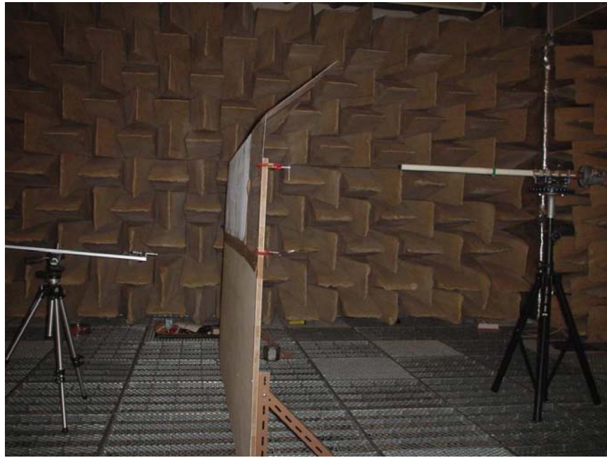
Photo 5.1 – the actual set up of the indoor experiment inside the anechoic chamber
