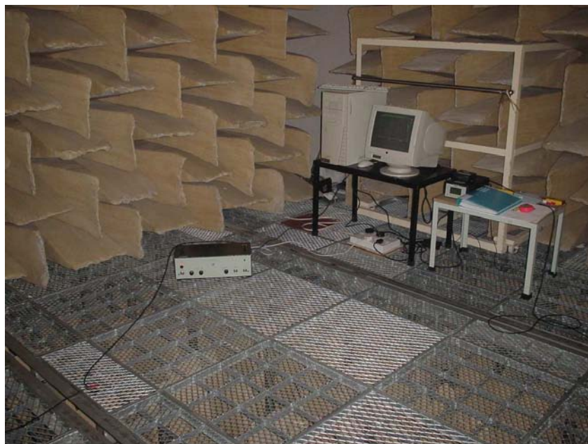
Photo 5.1 – the actual set up of the indoor experiment inside the anechoic chamber
