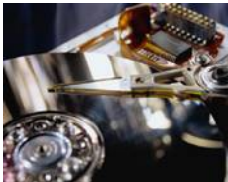
Figure 3-2 A hard disk with GMR read head. After ref. [3.7].
