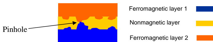
Figure 3-13 Schematic for the formation of pinhole in PSV structure
