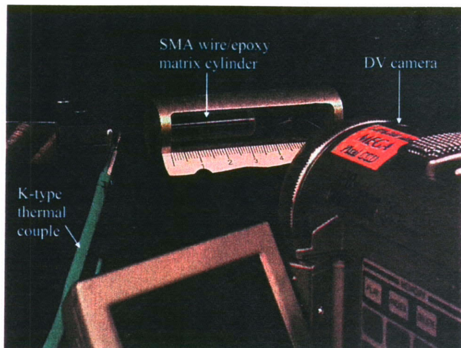
Figure 6.5 Debonding process is recorded by high resolution digital video camera.
