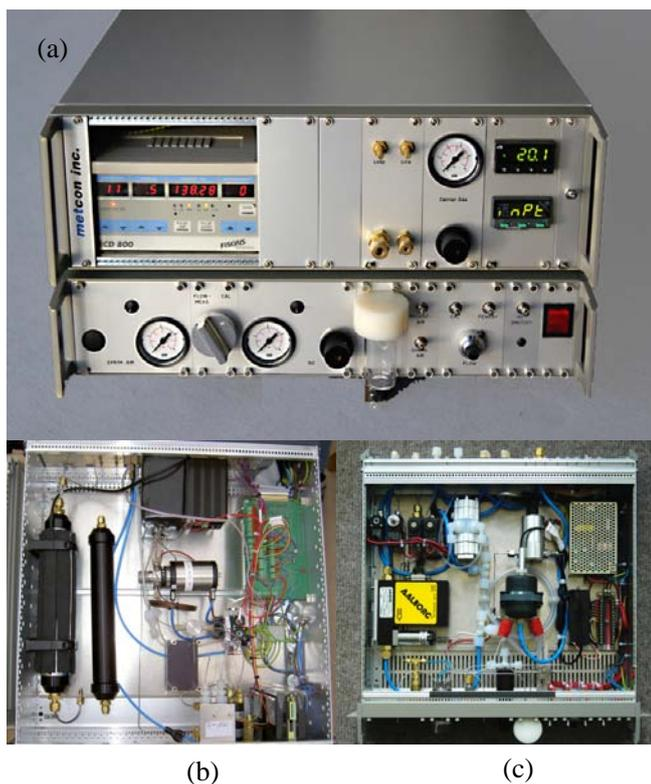
**Figure 4-12.** PAN-Analyzer and Cal-Unit: (a) PAN-Analyzer (above) and calibration unit (below); (b) PAN-Analyzer; (c) calibration unit.
