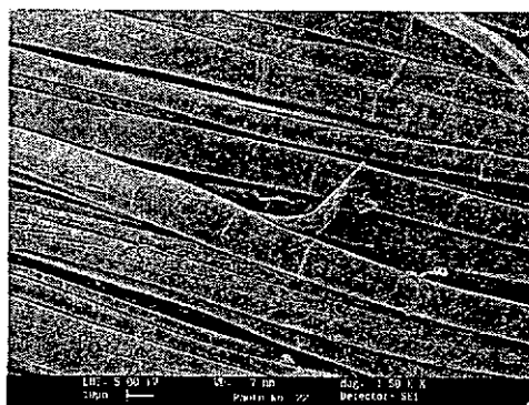
Figure 7.12: SEM micrograph of 100% tension mercerized linen
