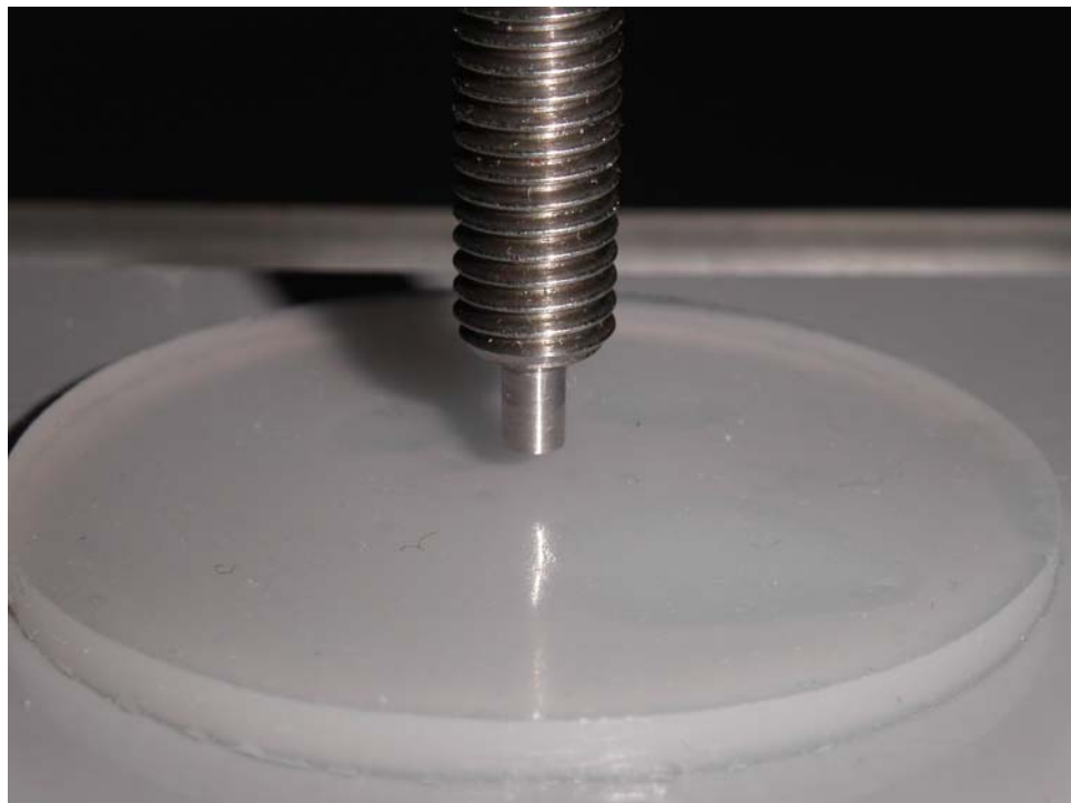
Figure 32 Indentation on the silicone phantom using Instron material testing system, indenter radius was 1.5 mm.
