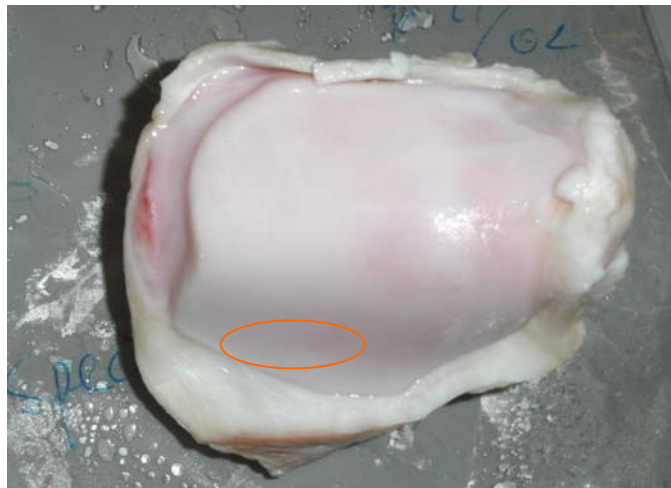
Figure 33 Fresh bovine patella with a layer of articular cartilage was bought from market and rinsed by isotonic PBS solution before experiment. The orange circle indicates the tested flat area located at the lateral articular facet of the patella.
