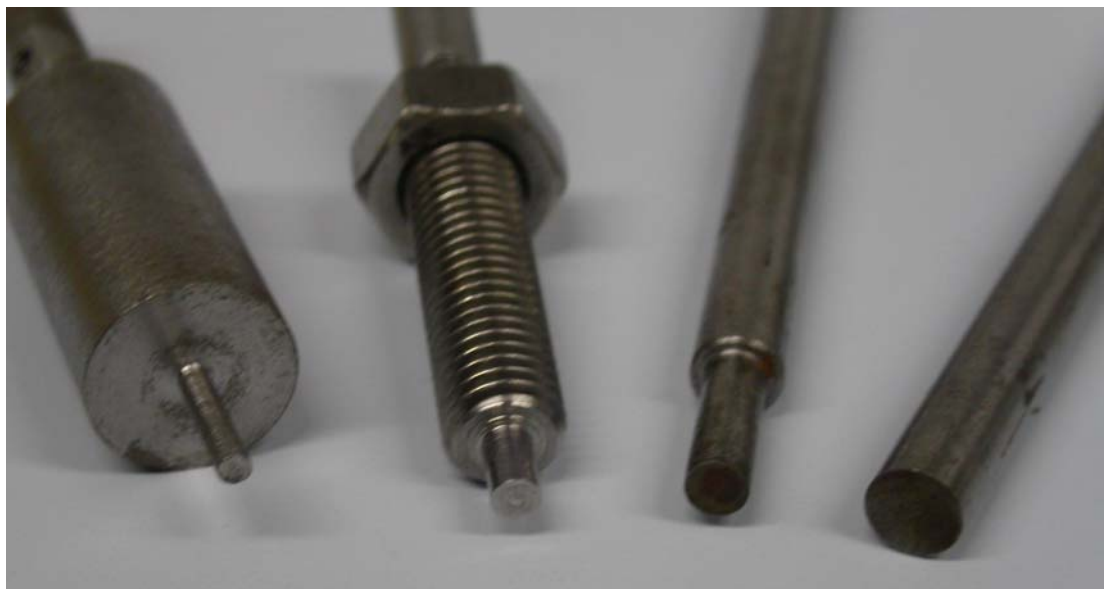
Figure 31 Indentors with different radius (from left to right, 1 mm, 1.5 mm, 2 mm and 3 mm).
