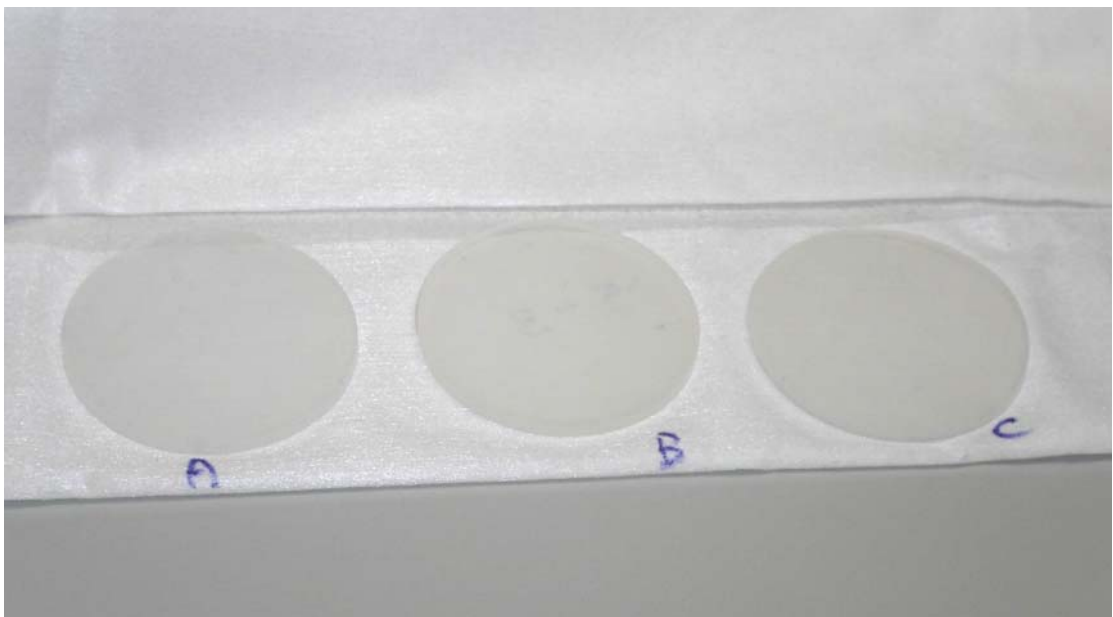
Figure 27 Three circular sheet silicone phantoms were fabricated from a material with almost the same mechanical properties as TC-2 silicone phantom, which was prepared for indentation test in this study.
