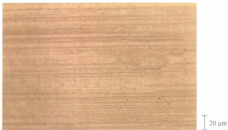
Figure 3.8a Pure LCP photomicrograph at 400×
