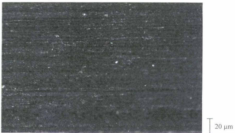
Figure 3.8f 5 % CB/LCP photomicrograph at 400×
