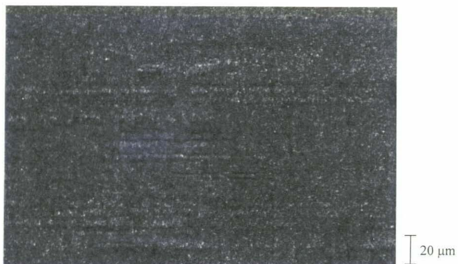
Figure 3.8g 6 % CB/LCP photomicrograph at 400 \times
