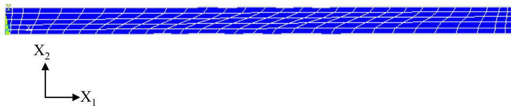
Figure 2.3 The simulated vibration mode shape at f_{111} in the X_1 - X_2 plane at the center of the quartz plate ( X_3 = 1.1 mm).
