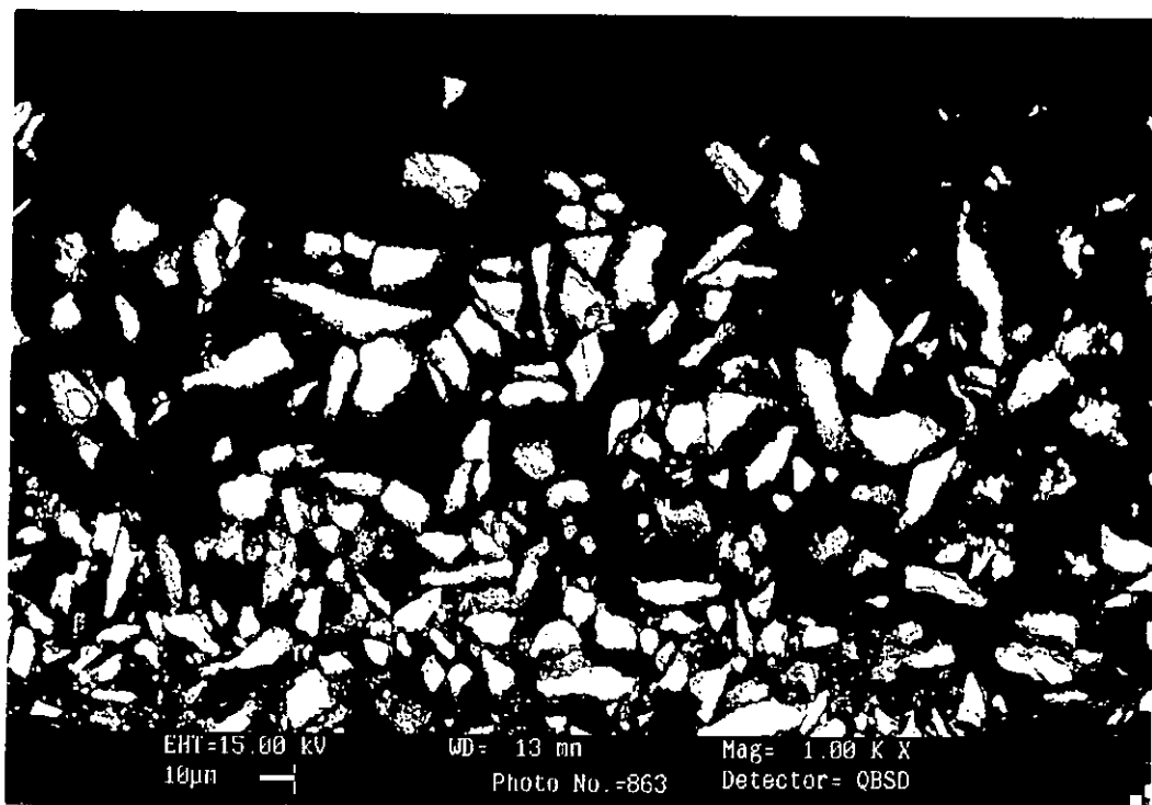
Figure 4.22 Cross-section of specimen D, layer clad with 40% Mo and 60% WC powder.
