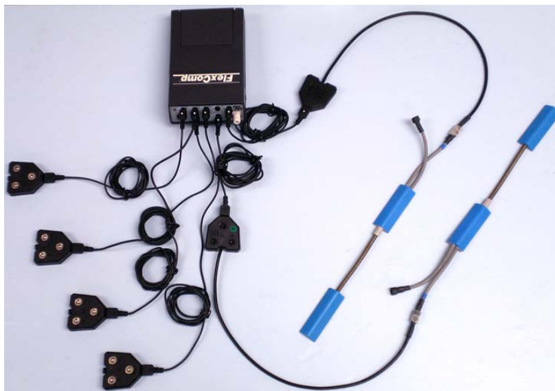
Figure 6-1: Flexcomp data acquisition system. The system had four EMG electrodes and two electrogoniometers connected.
