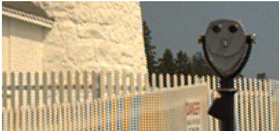
Figure 2.3 Simulation result generated by the smooth hue transition-based demosaicing algorithm [24]
