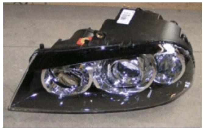
Figure 1.3b: Alfa Romeo HID Headlamp.
