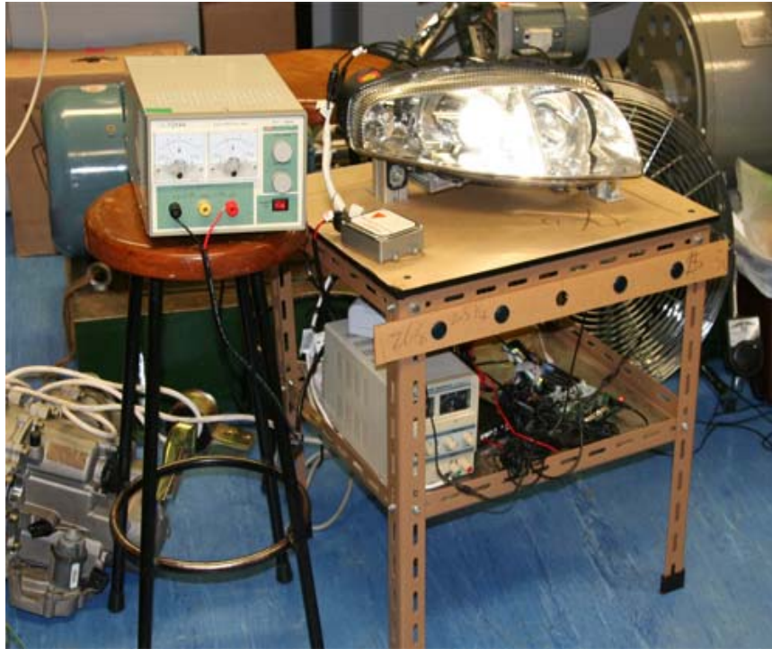
Figure 6.4: Testing Platform of Low Beam Levelling System
