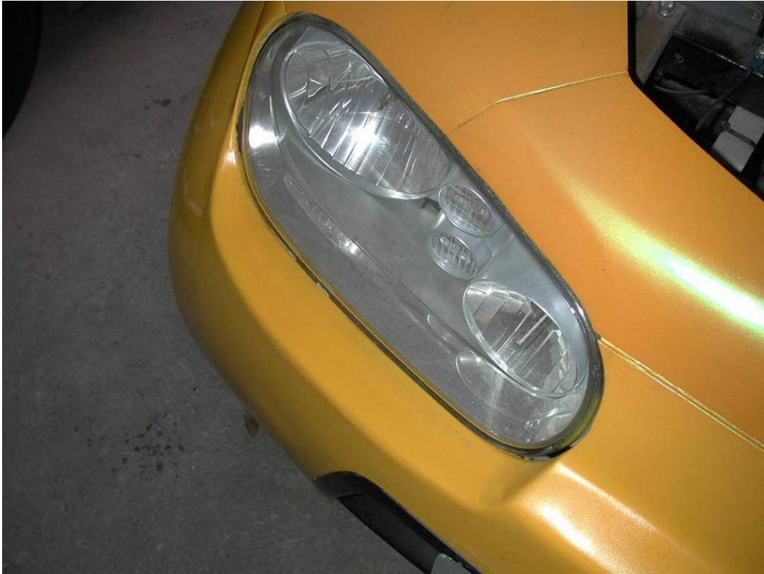
Figure A.8 HID installed to the PolyU EV4.
