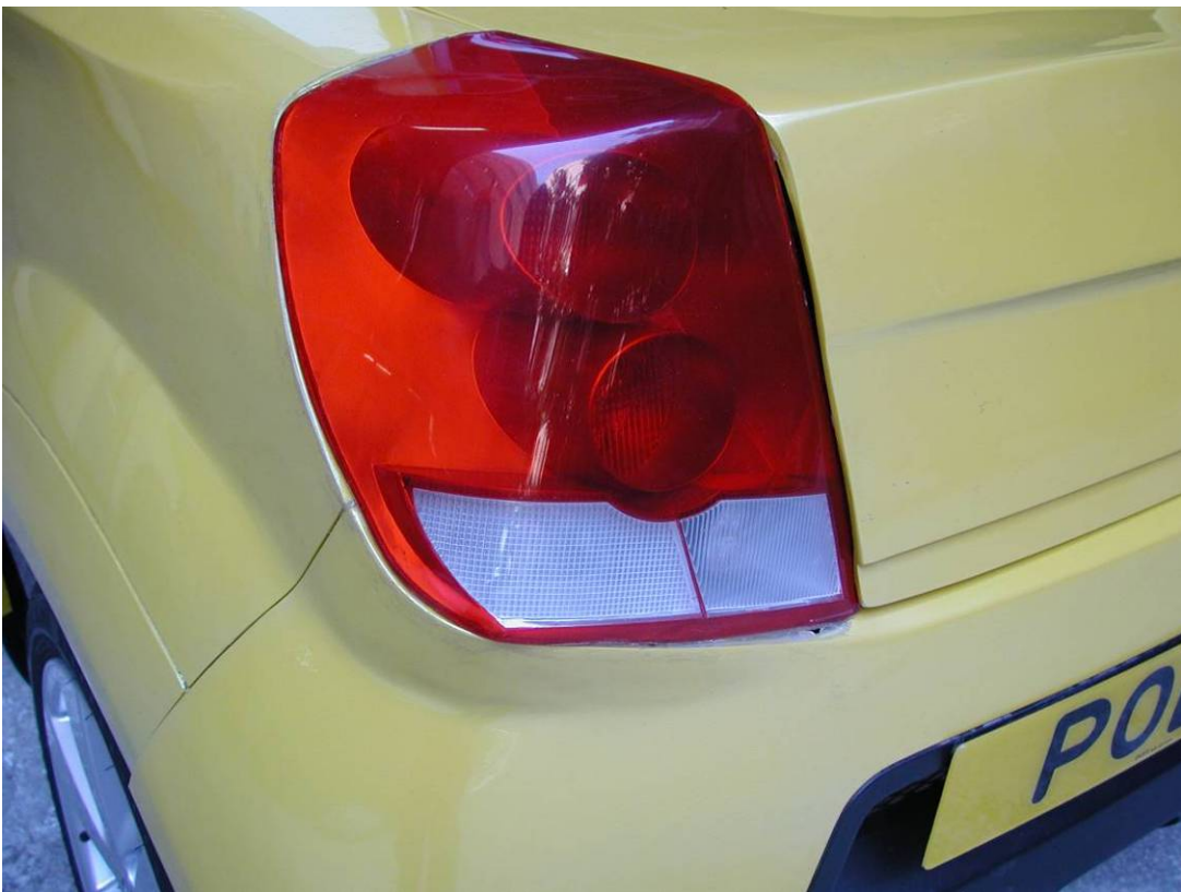
Figure A.9 LED rear lighting installed in PolyU EV4
