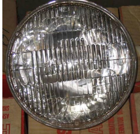
Figure 1.2: Headlamp with glass magnifier (Corning Conaphore headlamp)
