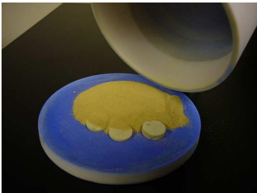
Figure 2.6 Photograph of the configuration used in calcination and sintering.
