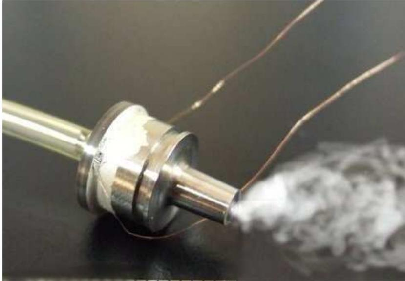
Figure 7.5 Horizontal nebulization under a 120V p-p driving voltage.
