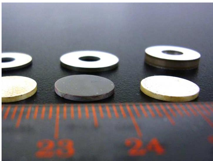
Figure 2.9 Photograph of piezoelectric ceramic samples.
