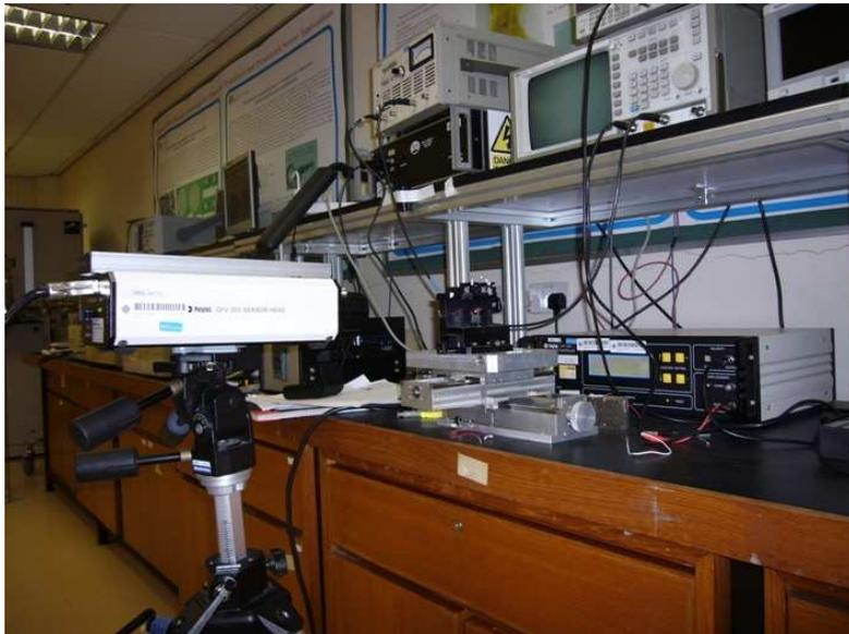
Figure 6.1 A photograph of the Laser Doppler Vibrometer setup in our laboratory.
