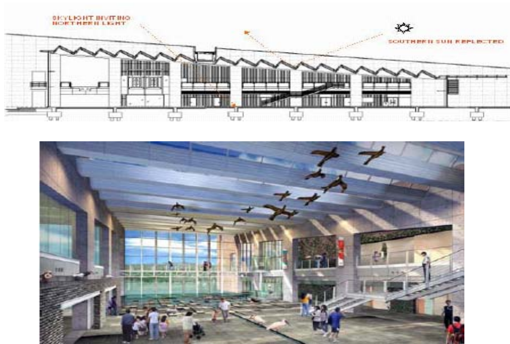
Figure 6.8 Skylight and Curtain Wall System provide the Visitor Centre with Natural Lighting
