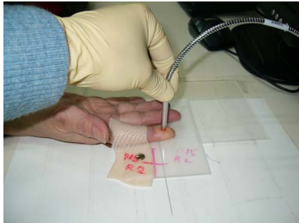
Figure 7-1: NIR spectroscopic probe measurement with customized finger mould
