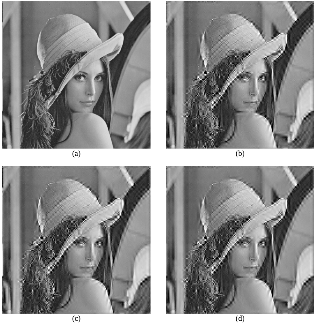
Figure 5.9 Reconstructed images of the (a) original image, (b) conventional EZW algorithm, (c) modified EZW algorithm with pre-processing of the value of threshold of two and (d) modified EZW algorithm with pre-processing of the value of threshold of five respectively with three decomposition levels using Daubechies 9/7 kernel
