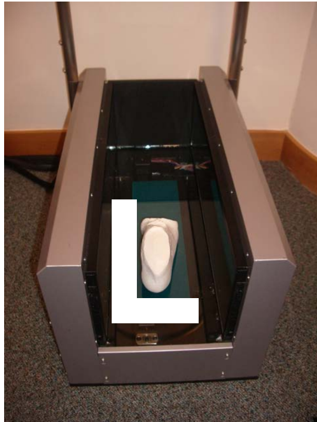
Figure 3.4.3-4 An L-frame helped to locate the plaster models in the same position on the scanning platform for each scanning
