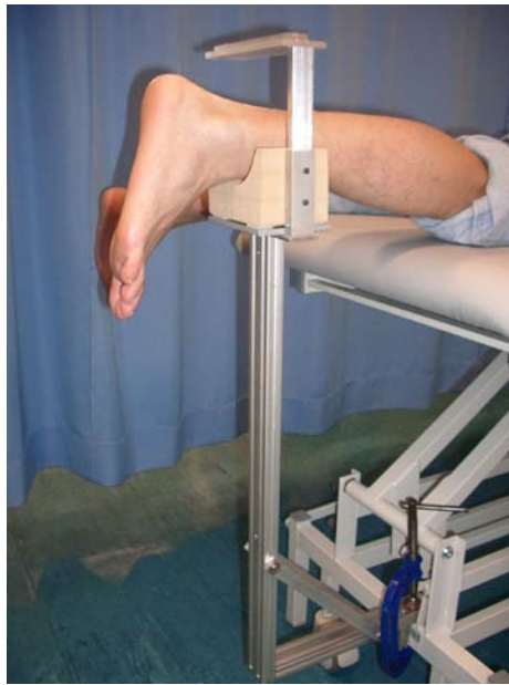
Figure 3.3.1-6 The u-shaped cushioned ankle support attached to the examination table for stabilizing the lower leg at the knee joint axis horizontal.
