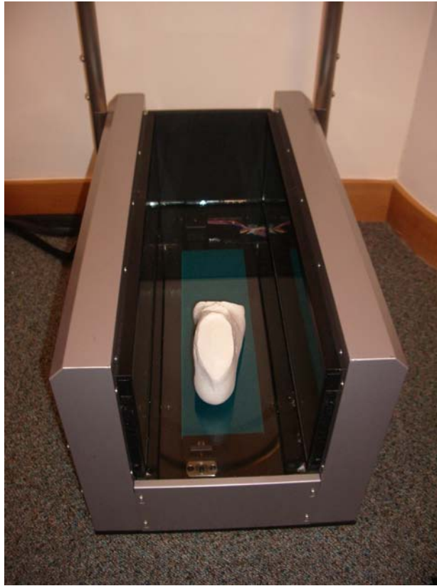
Figure 3.2.1-1 The INFOOT Foot Shape Scanner with the plaster model
