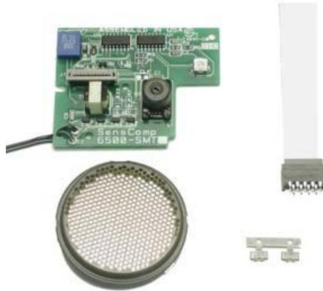
Figure 3-7: Polaroid 6500 series ranging module
