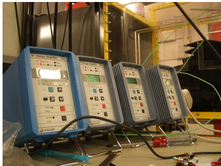
Figure 2.21 The charge amplifiers of the piezo-electric load cells.
