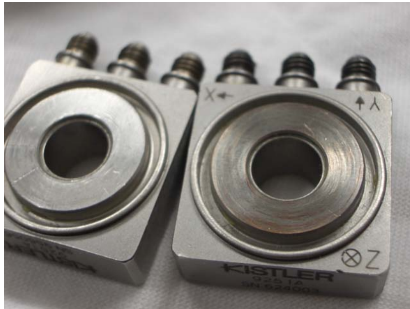
Figure 2.15 Piezo-electric load cells.
