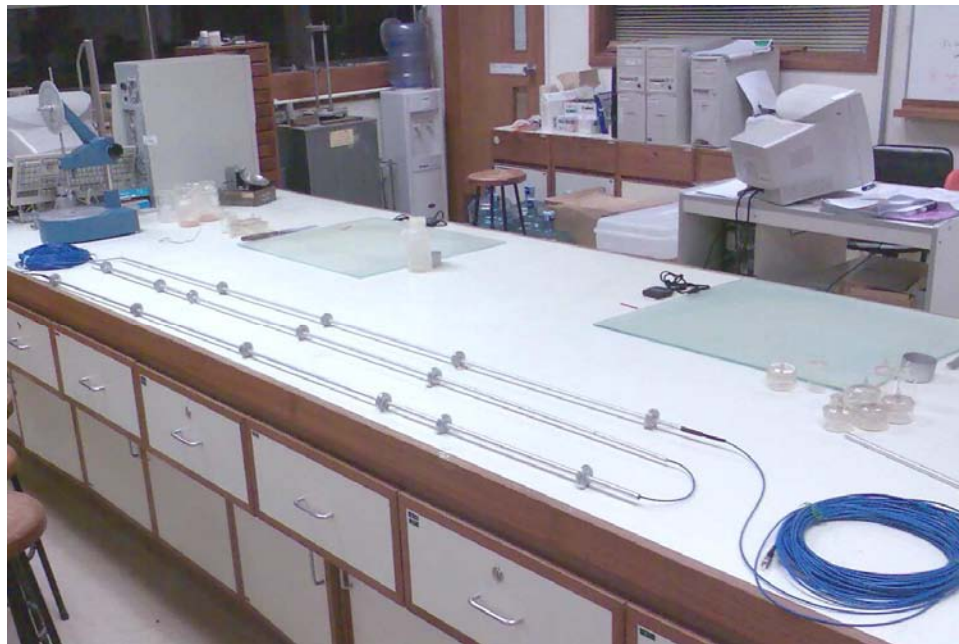
Figure 7.3 Photograph of the tube packaged FBG strain sensing arrays before field installation
