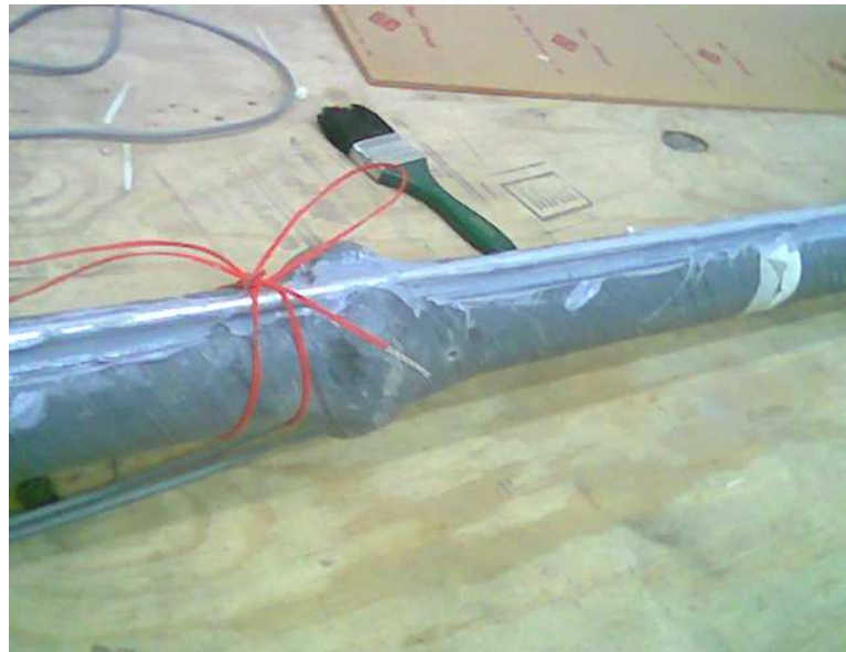
(b) FBG-B sensors in an aluminum pipe for continuous average strains
