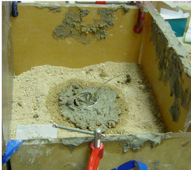
(b) Grouting of the hole by cement-bentonite slurry
