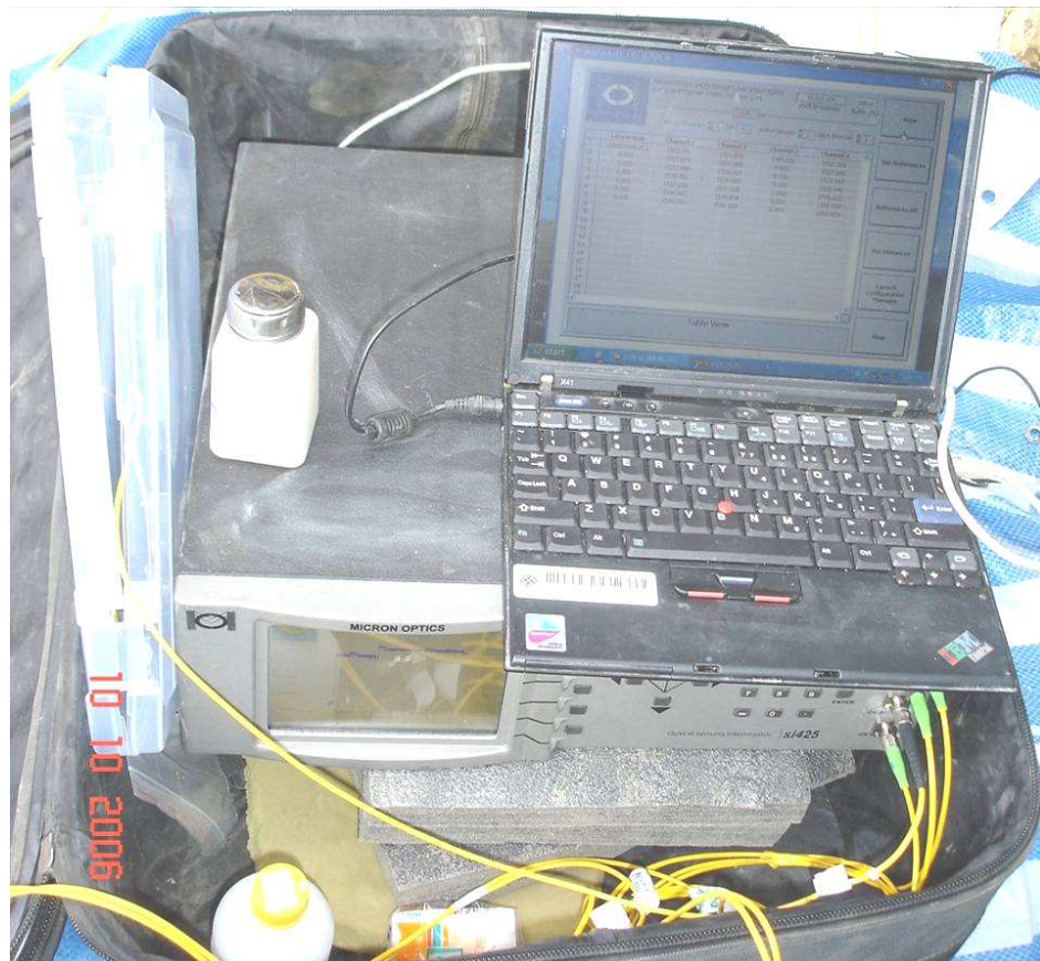
(b) An optical sensing interrogator si425 for measuring FBG readings
