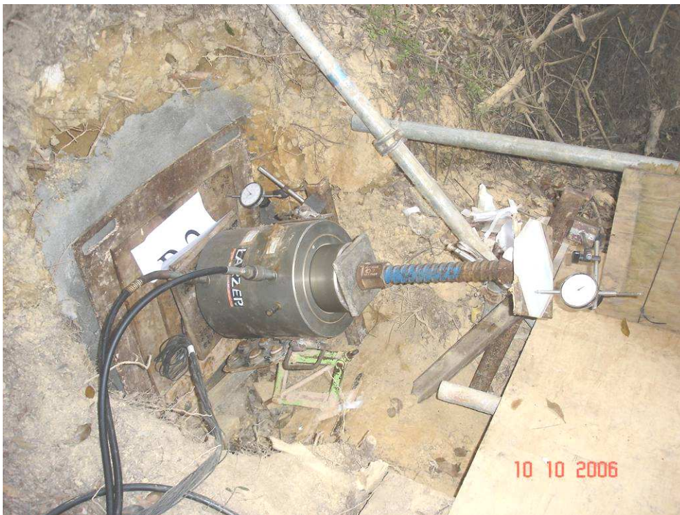
(a) Pullout test set-up
