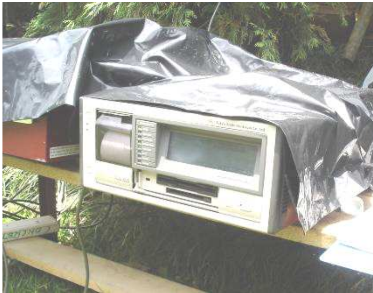
(c) A data logger for taking data of strain gauges, LVDTs and a load cell
