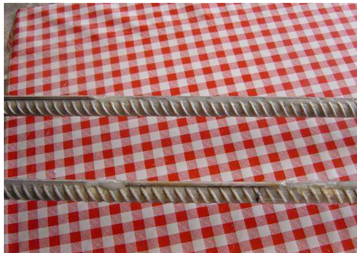
(a) Details of the soil nail instrumented with FBG strain and temperature sensors prior to installation
