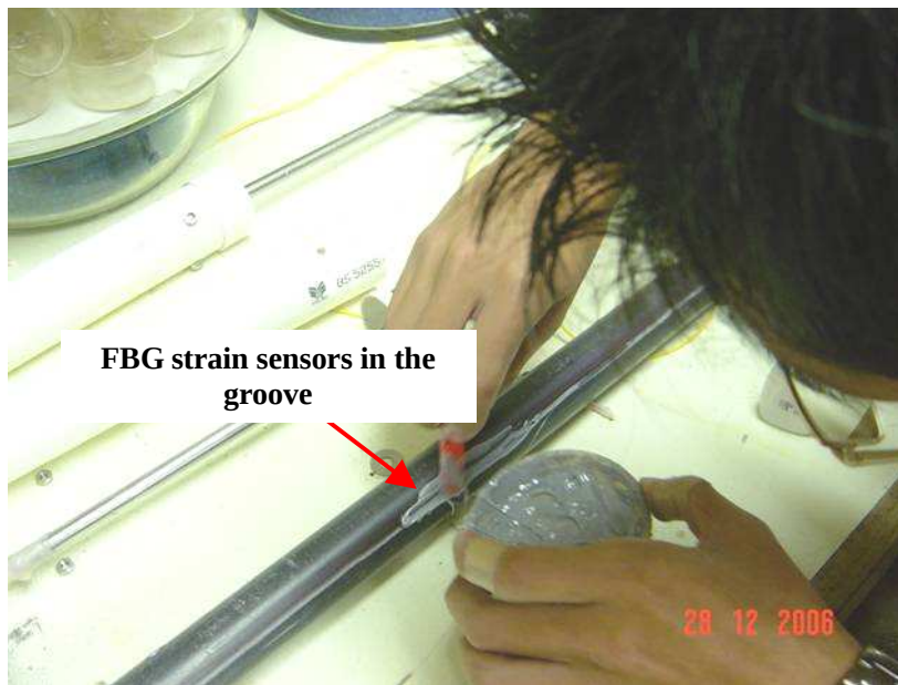
Figure 3.30 Fabrication of the FBG in-place inclinometer
