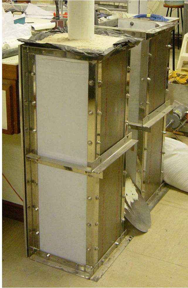
(a) Preparation of a hole for installing the settlement tube
