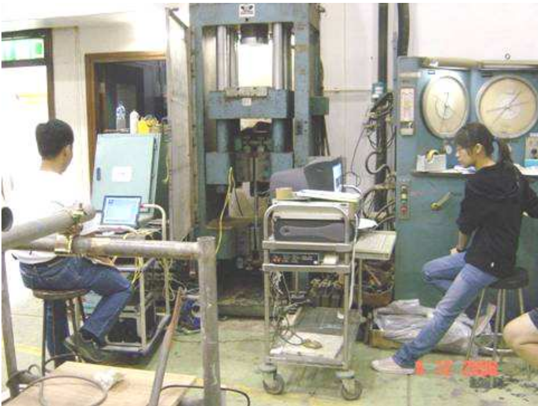
(a) Test set-up of the calibration of a steel bar with surface glued FBG sensors and strain gauges
