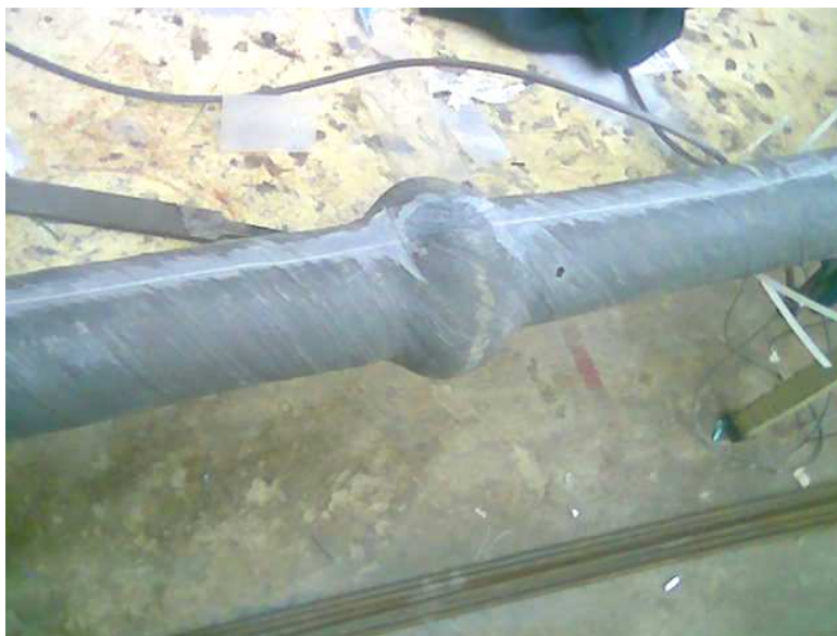
(a) FBG-A sensors on the surface of soil nail for point strains
