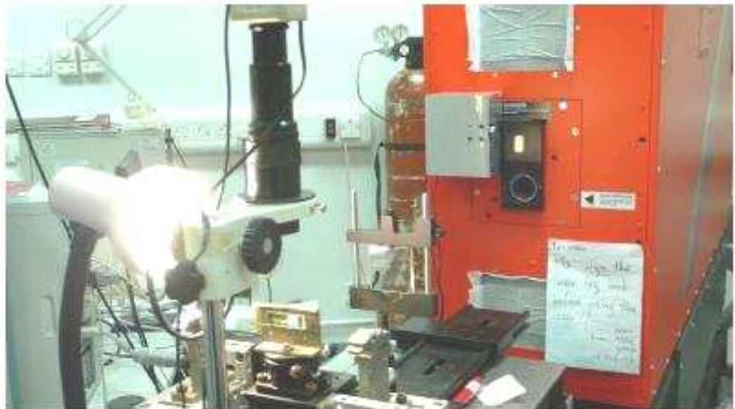
(b) Photograph of writing reflection grating using UV laser
