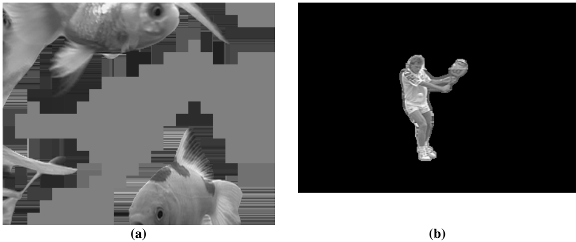
Figure 5-1. Examples of inaccurate video object segmentation (a) a repetitively padded “Goldfish” and (b) an inaccurately segmented object in sequence “Stefan”.
