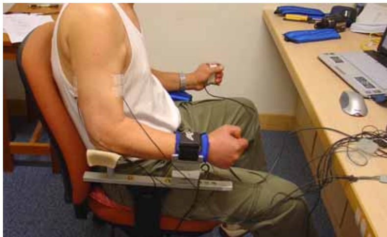
Fig. 2.4 Recording of maximum voluntary grip force produced by the non-affected hand, and EMG of the affected biceps and triceps as a measure of associated reaction
