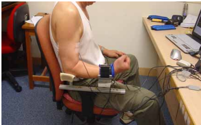
Fig. 2.1 Experimental set-up for recording of MIVC of the affected elbow flexors and extensors
