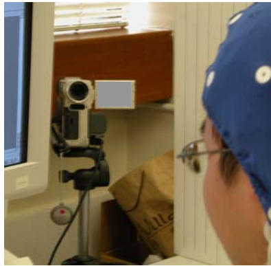
Figure 4.15. Video camera for recording the eye blink rate.
