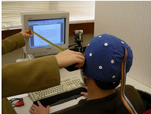
Figure 4.4. Measuring the distance between the subject and the monitor.
