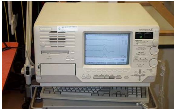
Figure 4.10. Nihon Kohden multi-functional device for capturing EEG signals.
